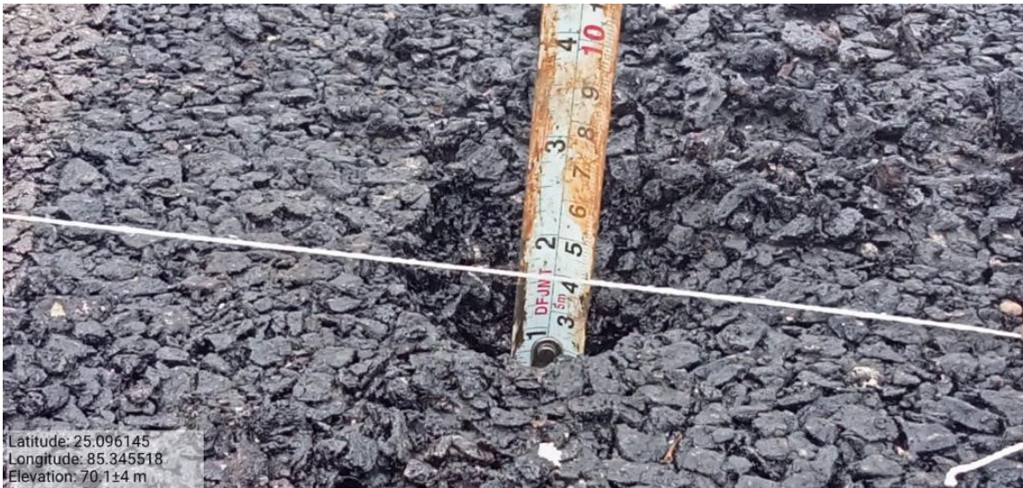
Figure 4.2 Thickness of pavement after SDBC
