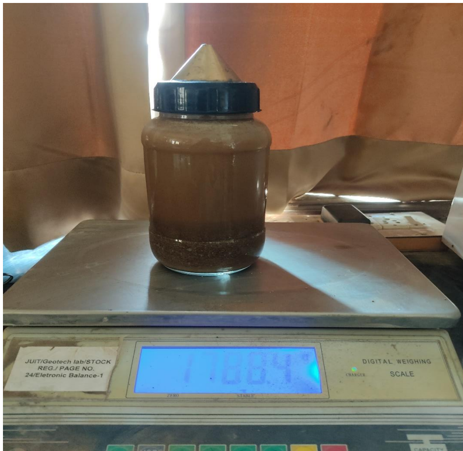
Figure 3.3 Pycnometer with soil + distilled water
