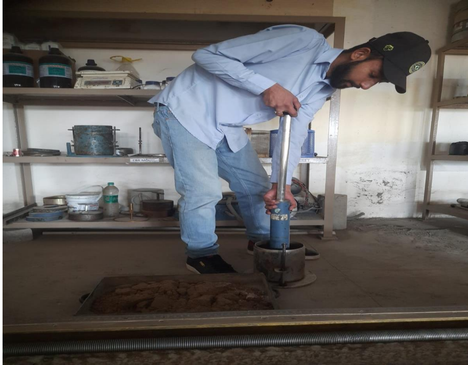
Figure 3.8 Compaction of soil in mould Source: JUIT, Transportation Engineering Lab
