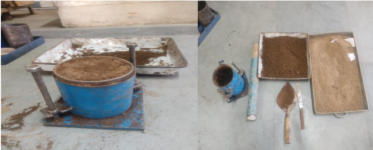
Figure 3.7 Proctor mould with compacted soil
