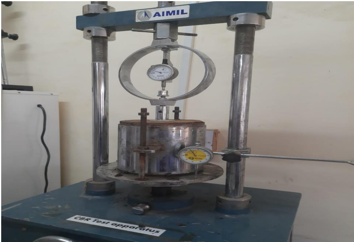
Figure 3.9 CBR Testing machine setup
