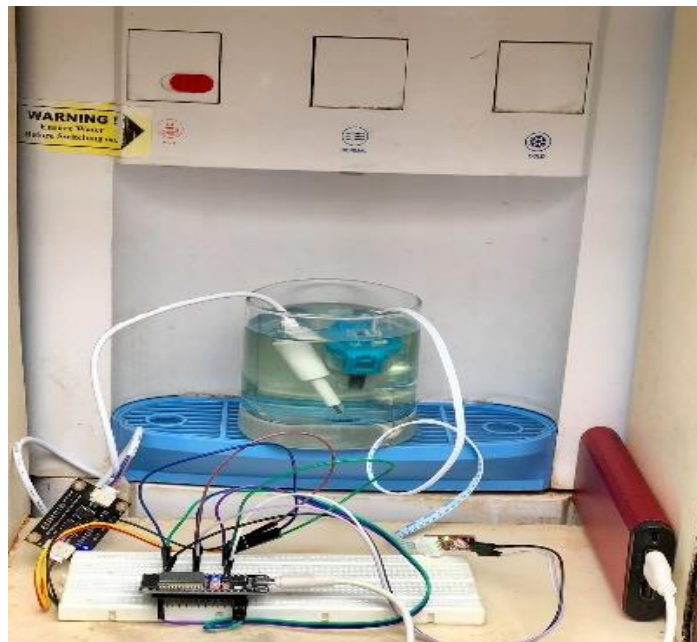
Fig 9. IoT implementation setup for detection of Water Quality
