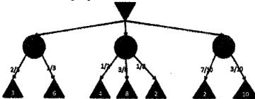
Circle nodes are chance nodes, the top node is a min node, and the bottom nodes are max nodes.
