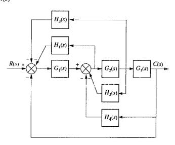
2. Using Mason's rule, find the transfer function,  $T(s) = \frac{C(s)}{R(s)}$  for the system represented below. [CO-2, Marks:4]
