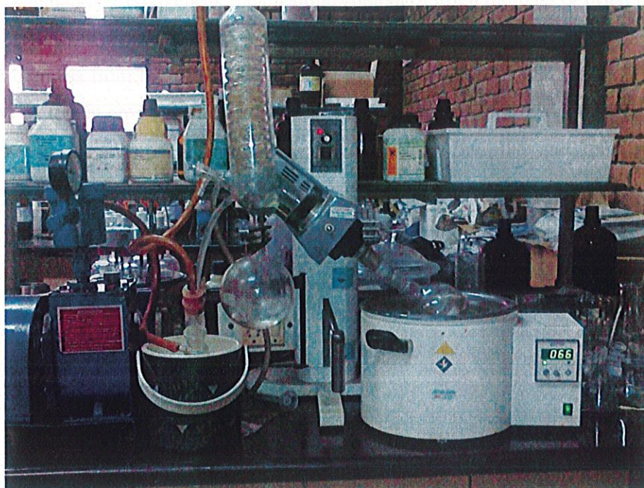
FIG 3.6 evaporation of the organic solvent using rotavac
