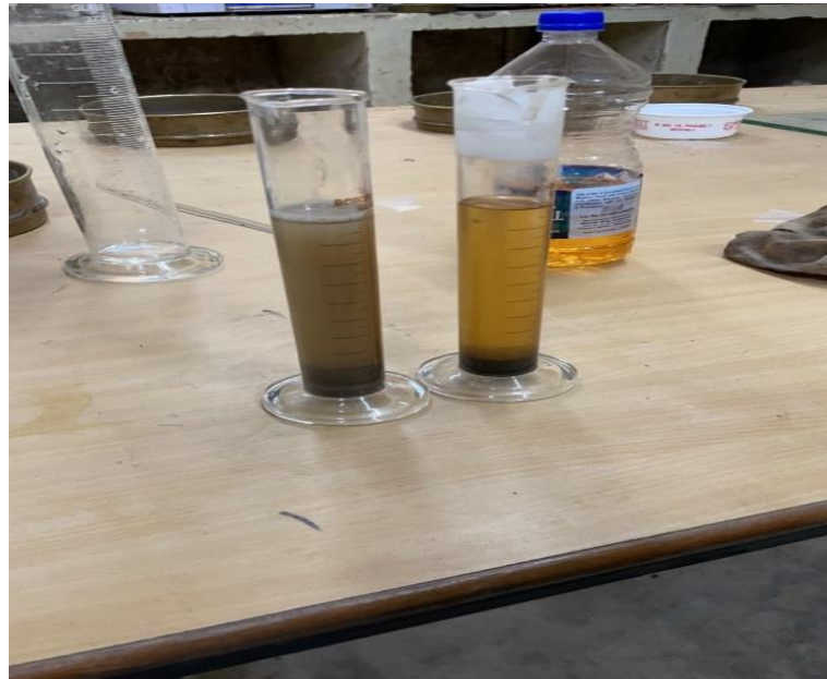
Figure 3.12: DFS tests of admixtures and their combinations
