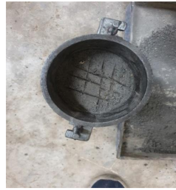
(c) Cut on soil sample for proper bond with next layer
