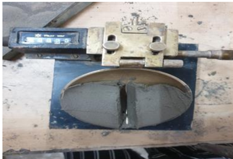
Figure 3.14: Liquid limit test on soil composite using Casagrande's apparatus
