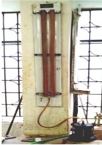
Figure 3.18: Falling head permeability test
