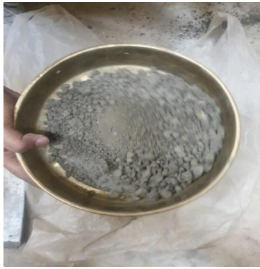
(a) Sieving sample from 4.75 mm sieve
