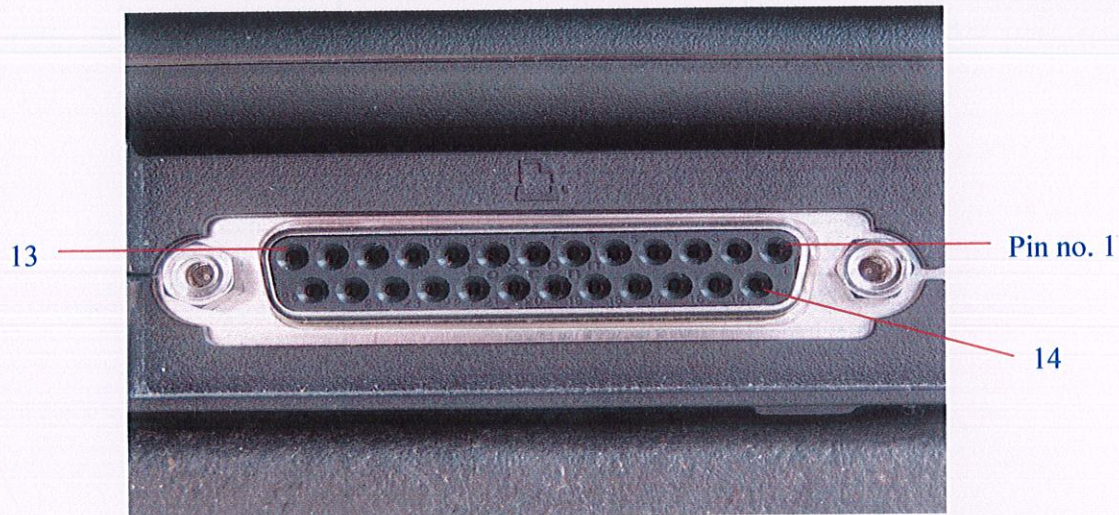
Figure 4.1: A DB-25 parallel printer port
