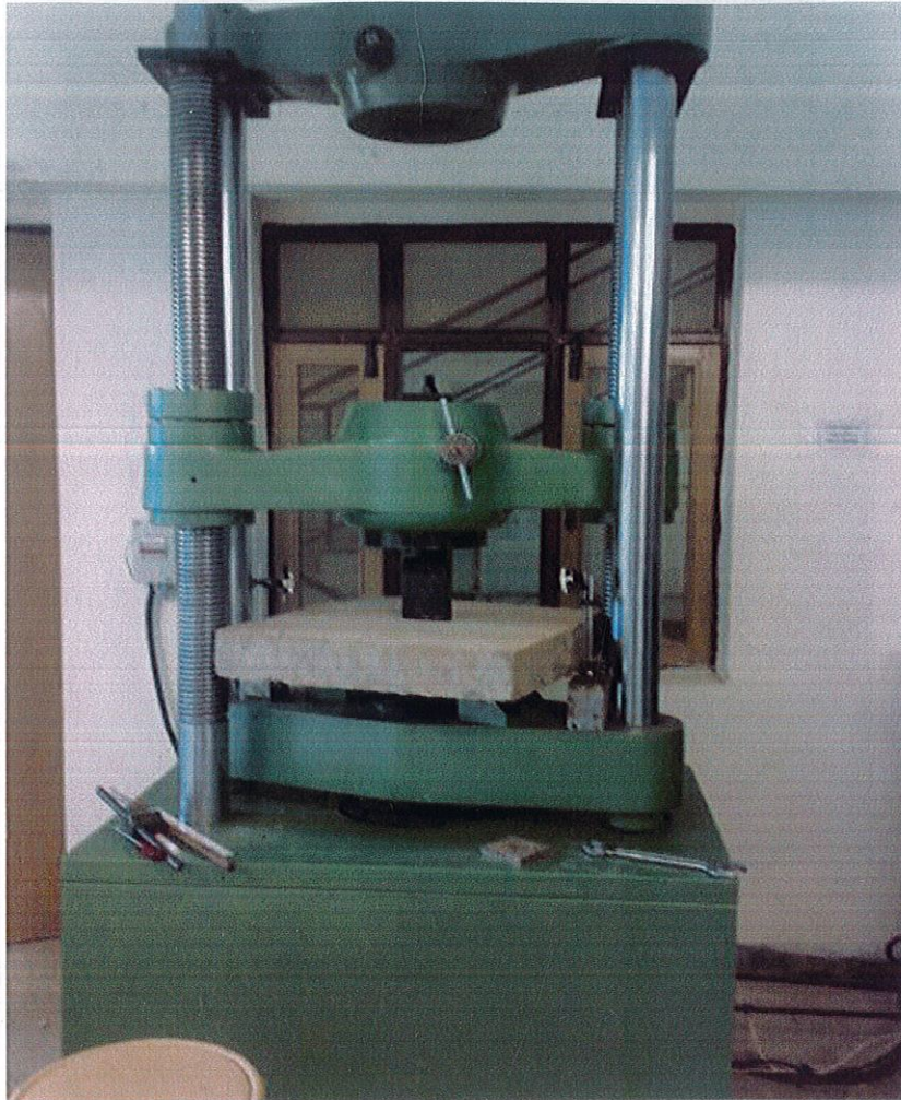
Fig.4.2 Slab being tested on UTM
