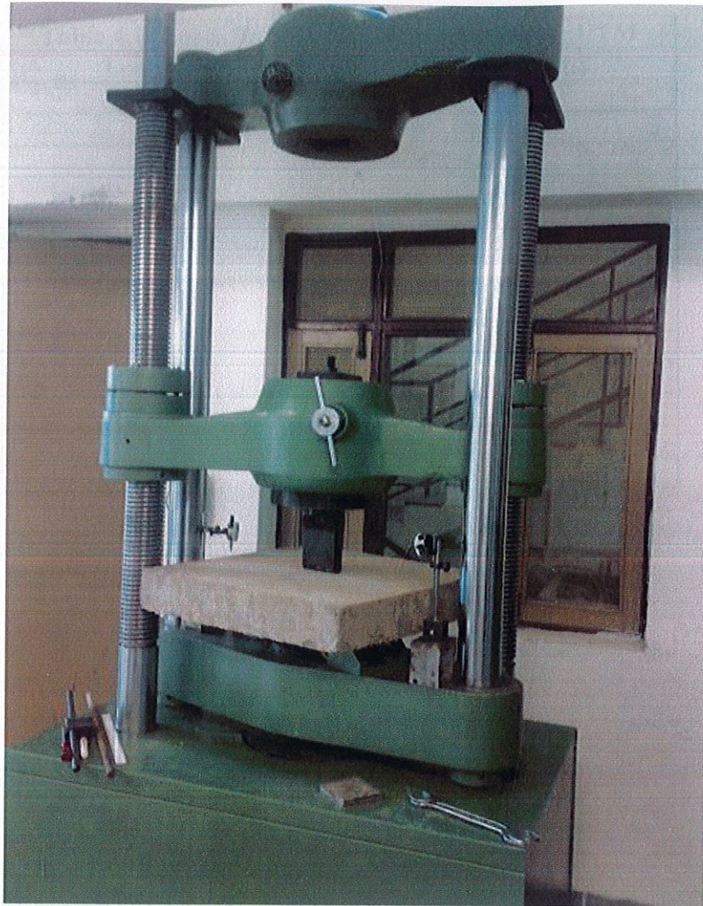
Fig.4.3 A line load is being applied using UTM at the centre of the slab
