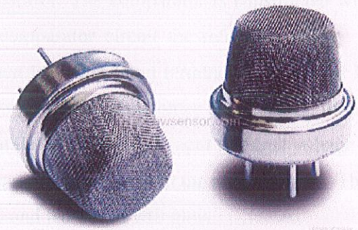
Figure 2.5 Gas Sensor (MQ2)
