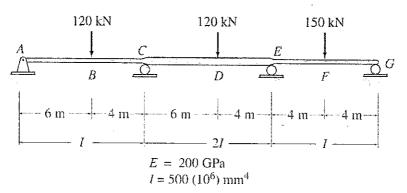
Q.3. Solve the given frame by using Slope Deflection Equation method. E = 200 GPa, I = 500 X (10<sup>6</sup>) mm<sup>4</sup>
