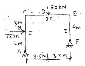
Q.3 Solve the given truss by Force Method.
