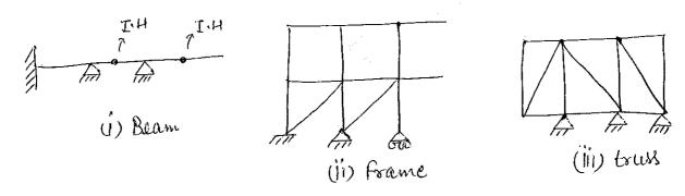
Q.3. Solve the given beam by using force method and draw the bending moment diagram & deflection pattern of the beam.
