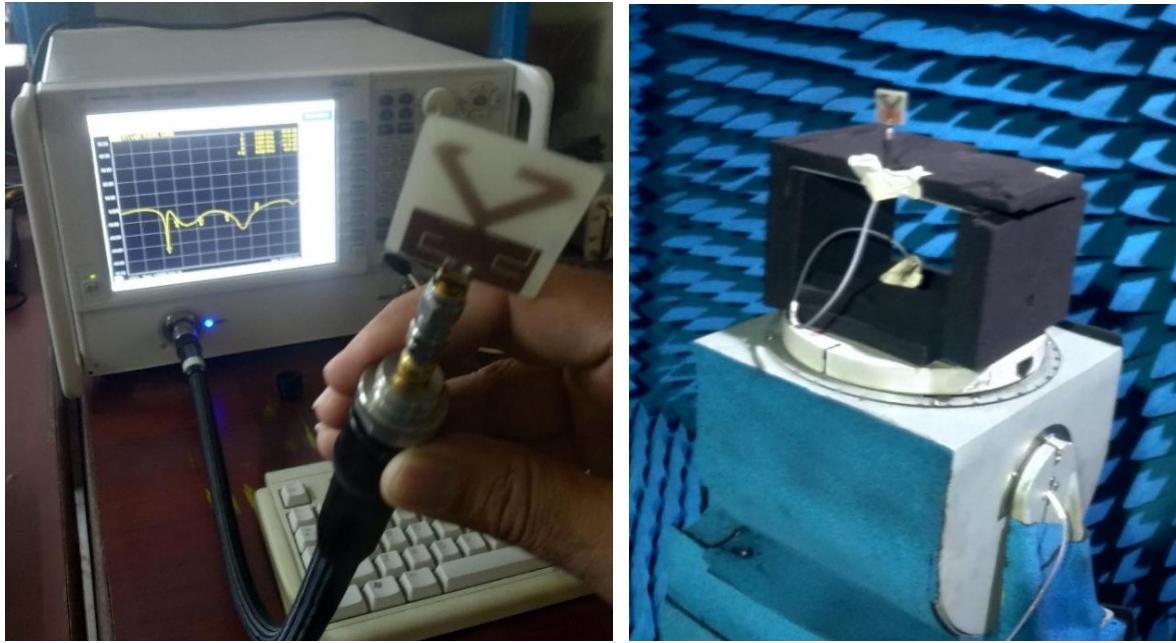
(b) S_{11} measurement of prototyped antenna with VNA
