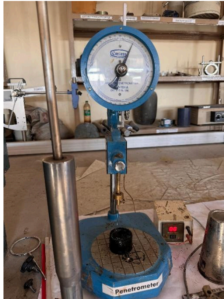
Figure 3. 7 PenetrationApparatus for bitumen and modified bitumen
