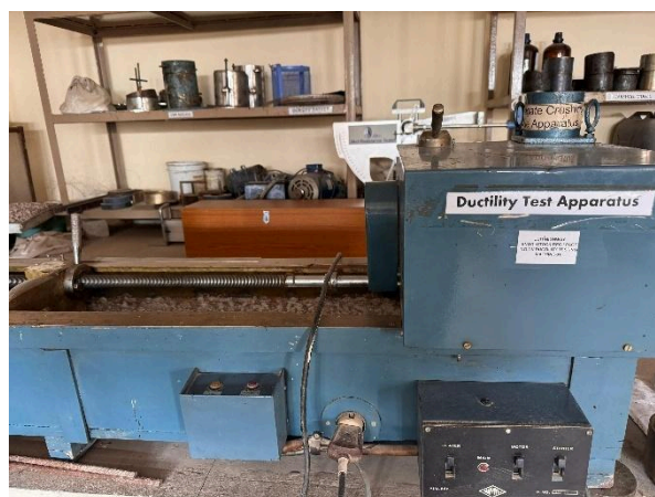
Figure 3. 8 Ductility test apparatus for bitumen and modified bitumen
