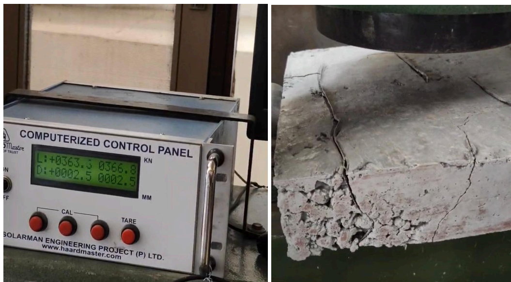
Figure 4.6 Testing of PCCBP Slab
