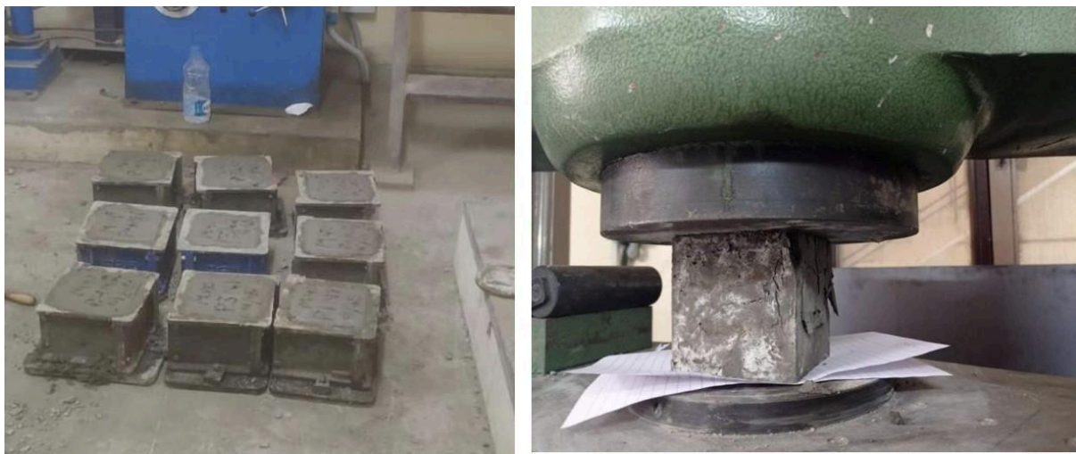
Figure3. 13 (a)Compressive Strength Casting (Cube-15cm*15cm*15cm)(b) Compressive testing using UTM
