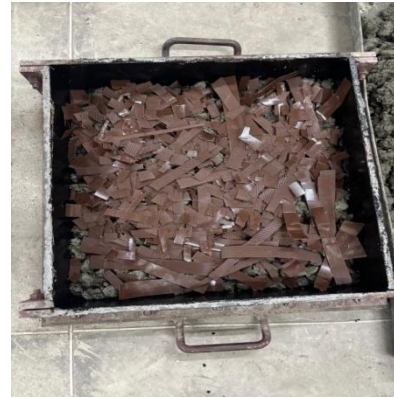
Figure3. 4 Plastic Cell Filled Concrete & Shredded waste Plastic Concrete slab
