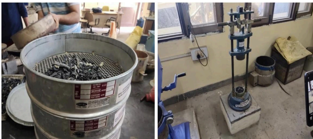
Figure3. 11(a) Sieve Analysis of Plastic Waste (b) Impact Test for Plastic Waste
