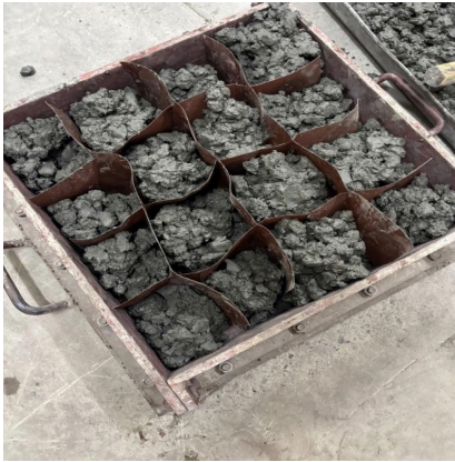
Figure3. 4 Plastic Cell Filled Concrete & Shredded waste Plastic Concrete slab
