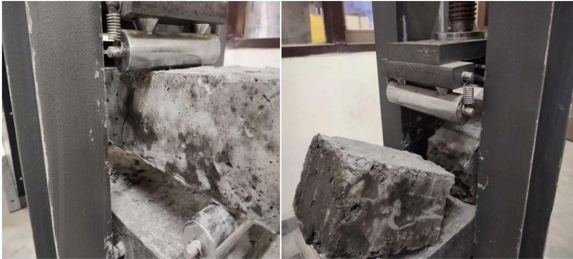
Figure3. 14 Flexural Strength Testing using third point loading
