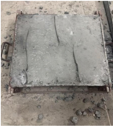
Figure3. 4 Plastic Cell Filled Concrete & Shredded waste Plastic Concrete slab
