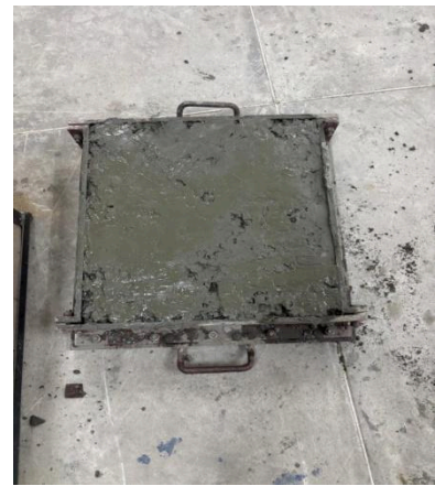
Figure3. 4 Plastic Cell Filled Concrete & Shredded waste Plastic Concrete slab
