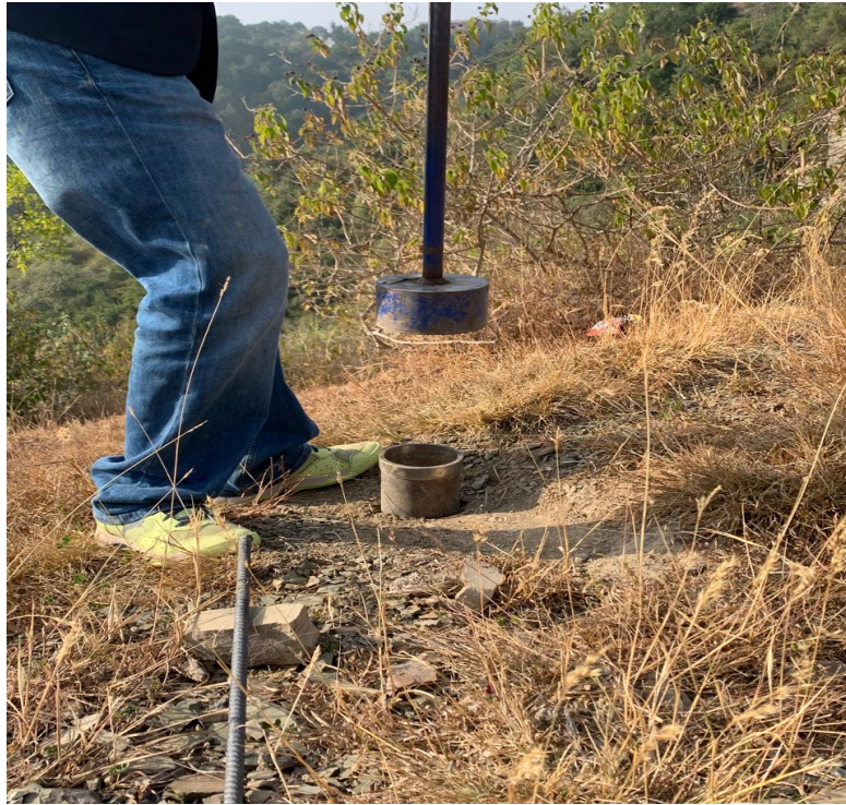
Fig 5.2 – Using rammer for core cutter test
