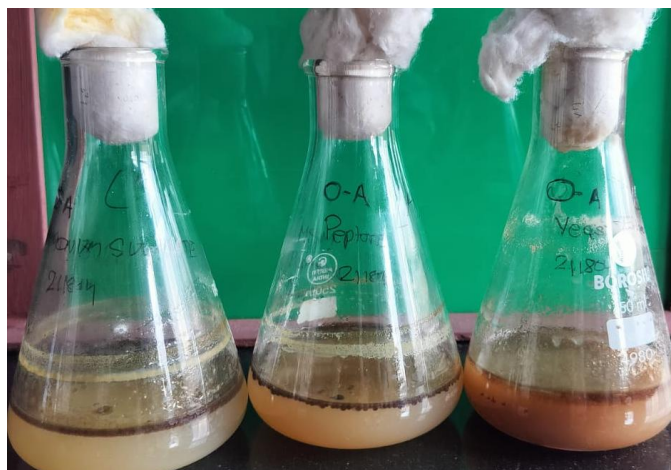
Fig.2: Flasks with nitrogen sources peptone, yeast extract and ammonium sulphate
