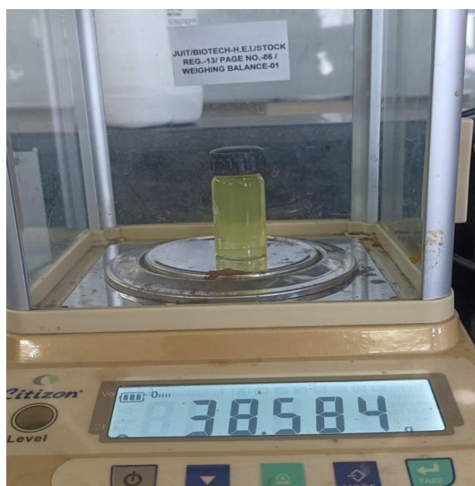
Fig. 3: Density measurement using specific gravity bottle and weighing machine
