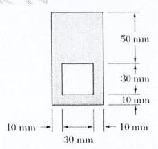
Q.3. Draw the bending stress diagram of the given composite section if the section can take maximum moment of 100 kNm.  $E_{STEEL} = 2.05 \text{ X } 10^5 \text{ N/mm}^2$ ,  $E_{BRASS} = 0.82 \text{ X } 10^5 \text{ N/mm}^2$ .
