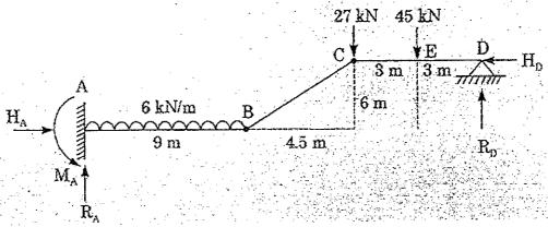
Q.2. Draw the axial force, shear force and bending moment diagram for the given frame. (6)
