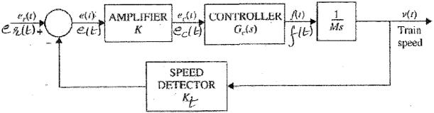
To determine the transfer function of the controller, we apply a step function of 1 volt to the input of the controller, that is,  $e_c(t) = u_s(t)$ . The output of the controller is measured and described by the following equation:
