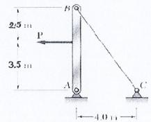
**Q6.**For the given combination of bars, if the temperature of the system is increased by  $60^{\circ}$ C, find the forces generated at the support.
