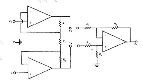
An Op-Amp differential amplifier (as in figure above) is built using four identical resistors, each having a tolerance of ±5%. Calculate the worst possible CMRR. [4]
