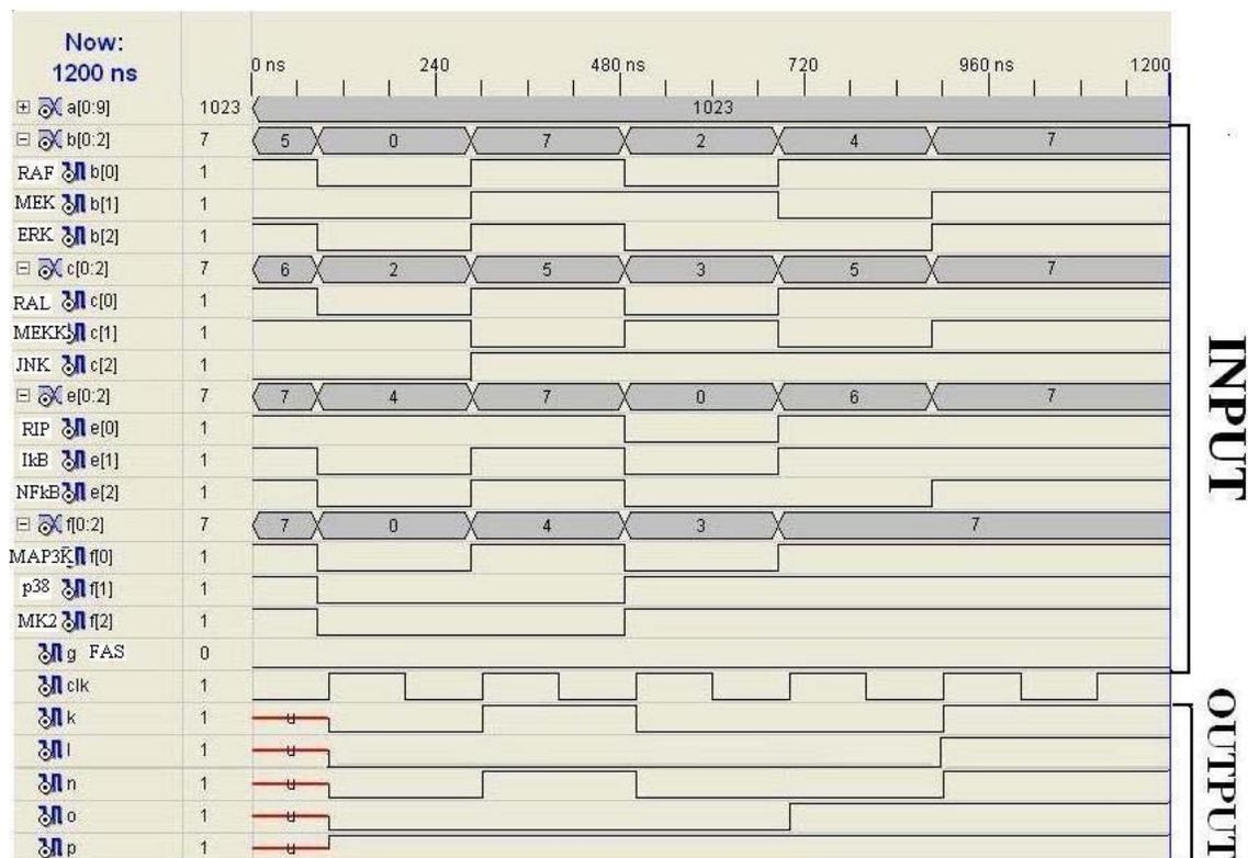
**Fig 2.21** System Implementation of TNF signal cascade using VHDL
