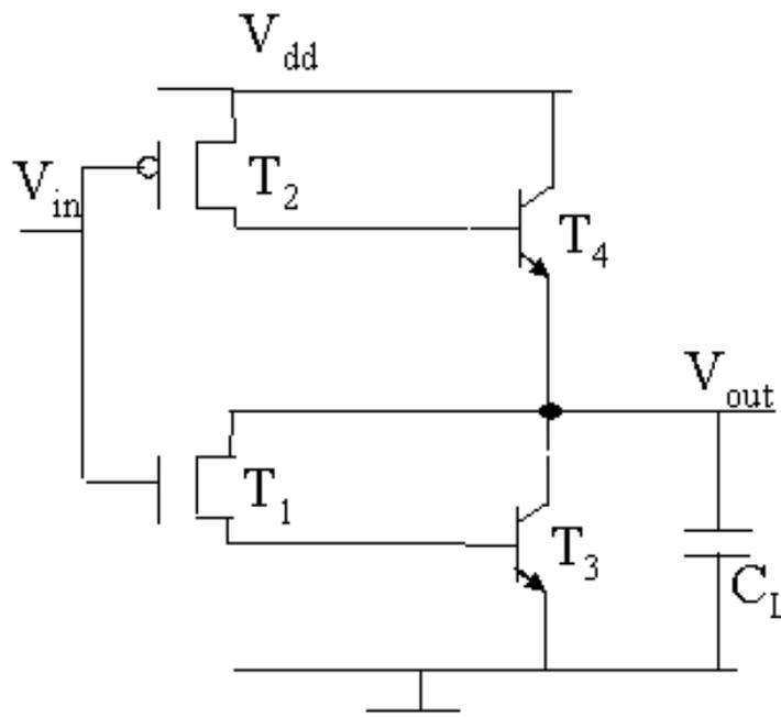
Fig 2.11 BiCMOS Inverter
