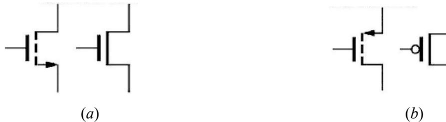
**Fig 2.7** Representation of (a) nMOS transistor (b) pMOS transistor
