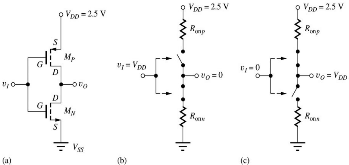
**Fig 2.8** (a) Circuit schematic for a CMOS inverter (b) Simplified operation model with a high input applied (c) Simplified operation model with a low input applied
