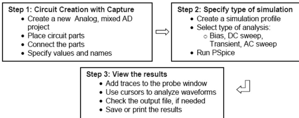
**Fig 2.6** Steps involved in simulating a circuit using SPICE
