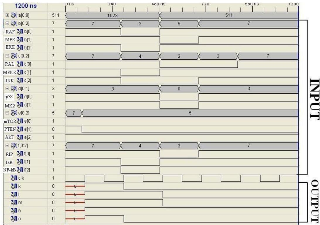
**Fig 2.24** System Implementation of TNF, EGF and Insulin combined signal cascade using VHDL
