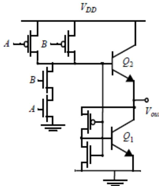
**Fig 2.12** Two input BiCMOS NAND gate
