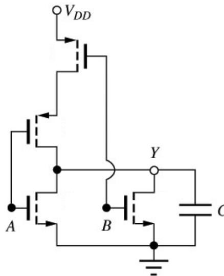
**Fig 2.10** CMOS NOR gate implementation
