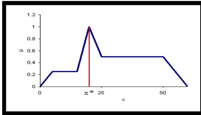
Fig 2.29 Max-membership Defuzzification methods
