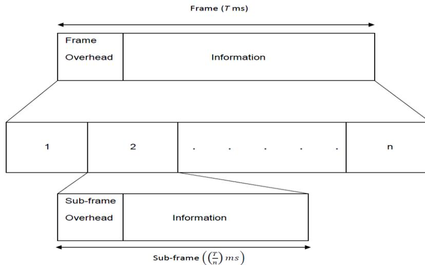
**Fig. 6.4** The detailed frame structure of the proposed scheme.
