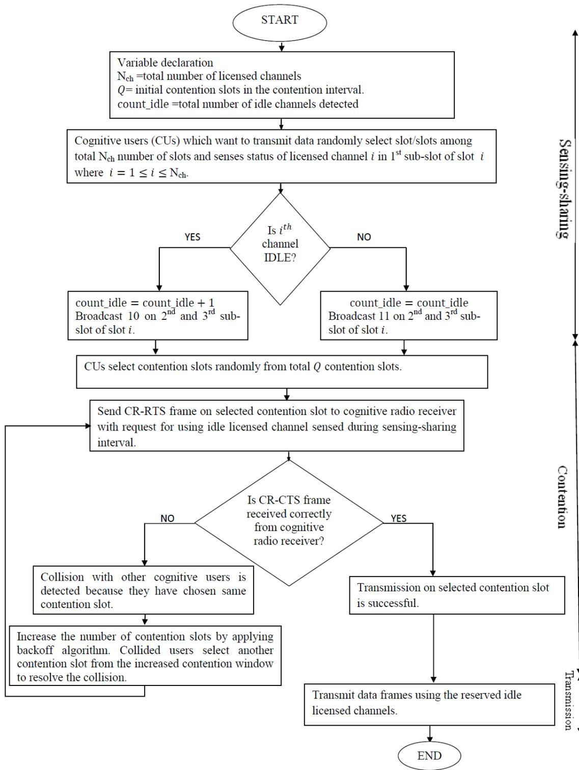
Fig. 2.3 The flow diagram of the proposed MAC protocol.
