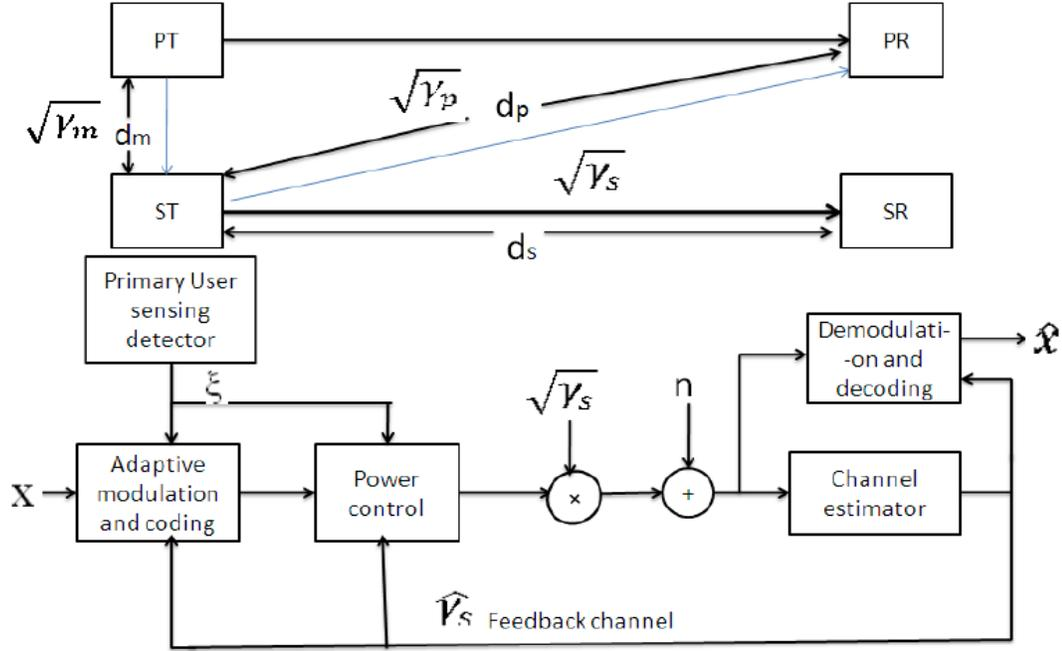
**Fig. 7.1** The proposed spectrum-sharing system model.
