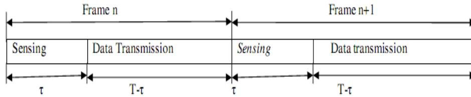
**Fig. 6.1** The frame structure of conventional sensing-based spectrum sharing approach for cognitive radio networks.
