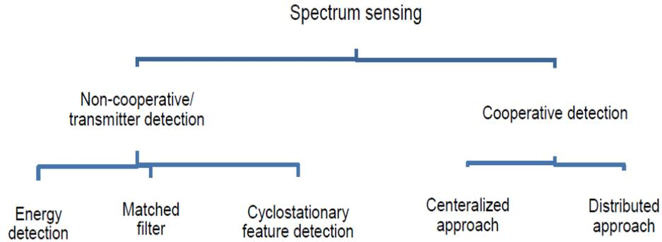
**Fig. 1.3** The spectrum sensing techniques.
