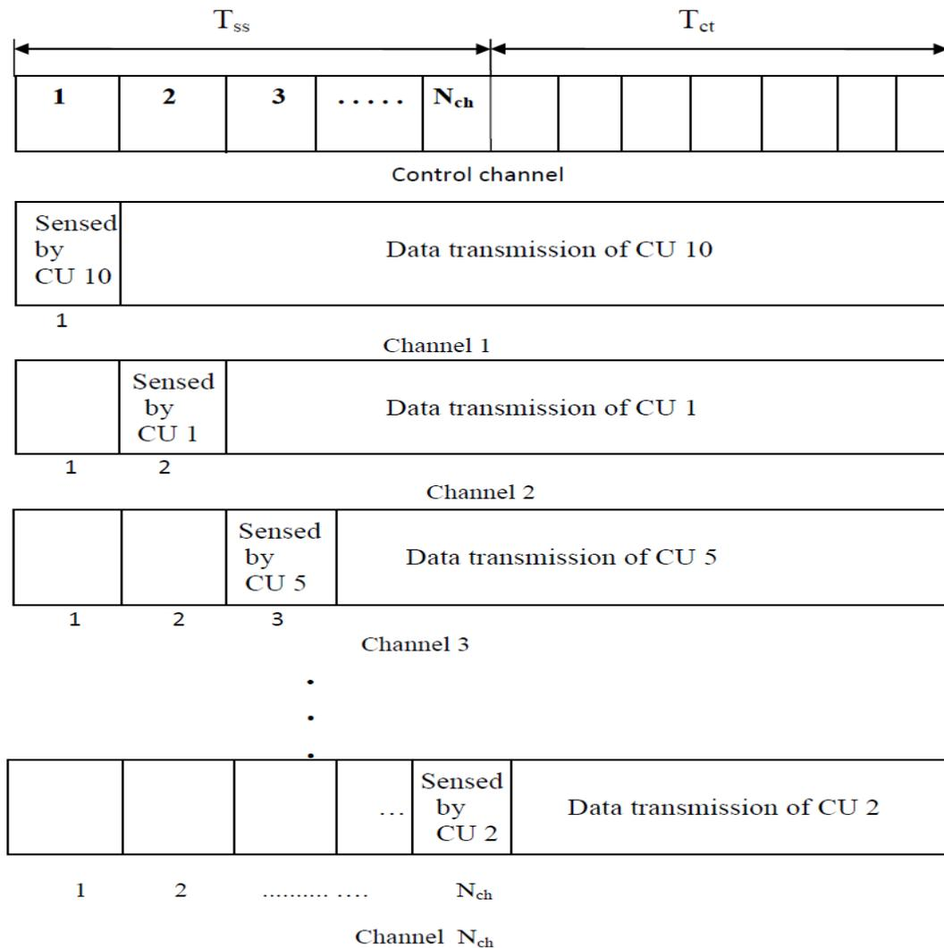
**Fig. 4.2** The proposed scheme to avoid bandwidth wastage in the proposed cognitive radio MAC protocol for the cooperative distributed network.
