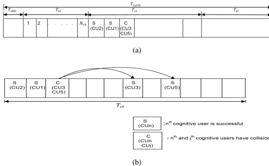
**Fig. 2.2** The control channel structure of (a) the SMC-MAC protocol [116] without the back-off algorithm during the contention interval and (b) the proposed scheme with the back-off algorithm during contention interval.
