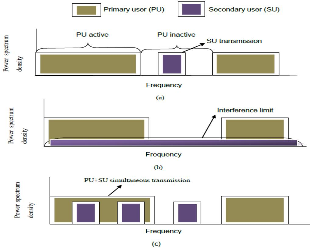
**Fig. 1.7** Spectrum access techniques (a) Spectrum interweave (b) Spectrum underlay, and (c) Spectrum overlay.
