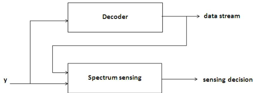
**Fig. 6.3** The receiver structure of cognitive user for the frame structure shown in Fig. 6.2 [156].
