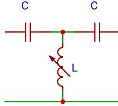
Figure 5.2.1: Unit cell of highpass transmission line model with non-linear inductor
