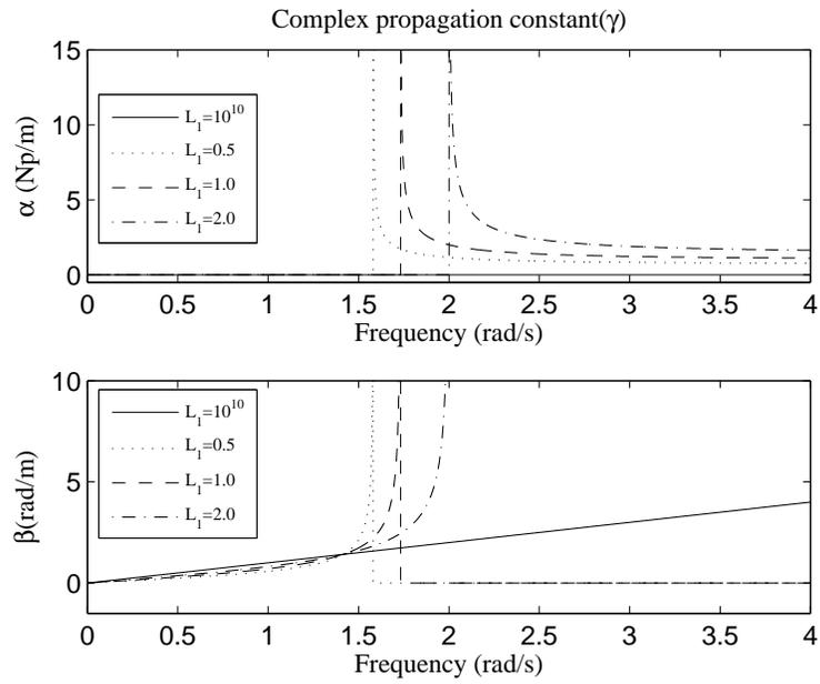
Figure 5.3.4: Complex propagation constant for lowpass with Miller inductive loading
