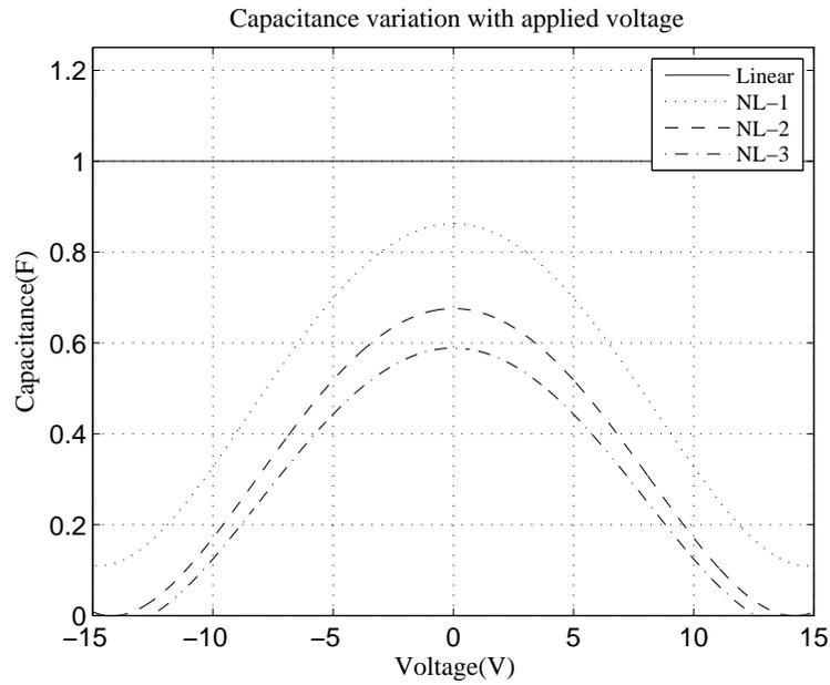
Figure 3.3.2: Variation in capacitance for different non-linearities
