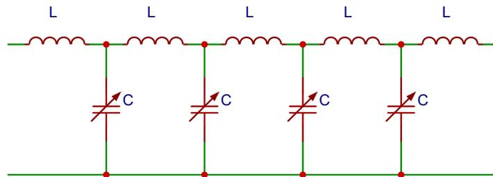
Figure 2.2.2: Equivalent circuit model with variable capacitor
