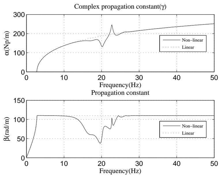
Figure 4.4.13: Complex propagation constant with both elements as non-linear
