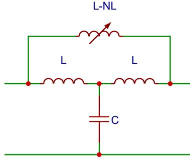
Figure 5.3.1: Unit cell of lowpass transmission line with Miller non-linearity inductor
