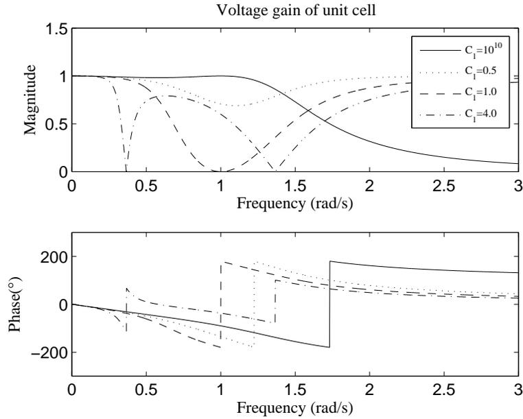
Figure 5.3.6: Voltage gain of unit cell with Miller capacitive loading
