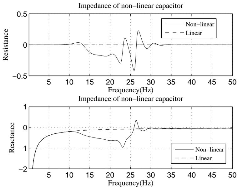
Figure 4.4.8: Impedance of non-linear capacitor
