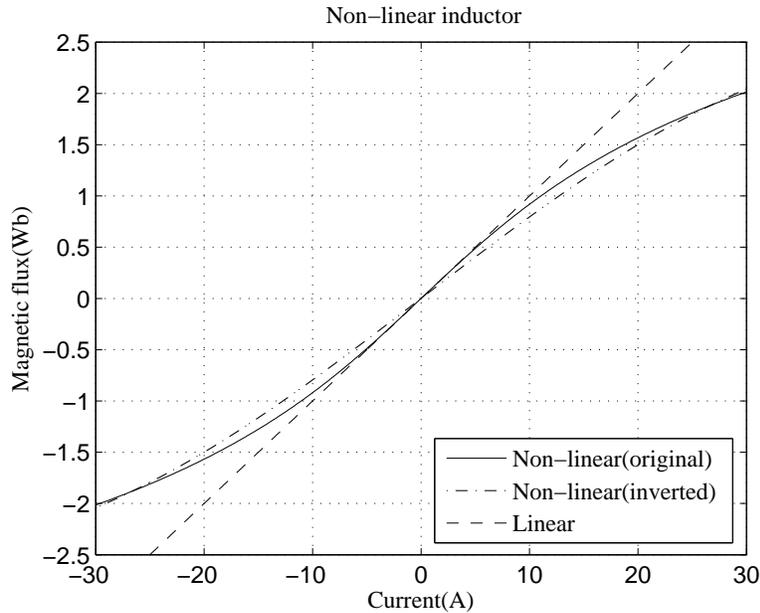
Figure 3.2.1: Relationship between current and magnetic flux for linear and non-linear inductors.
