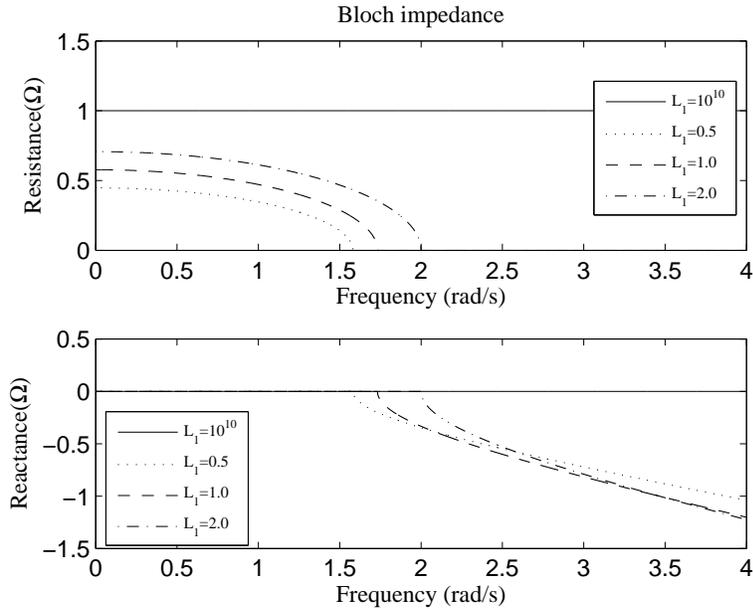
Figure 5.3.3: Bloch impedance of the lowpass equivalent circuit with Miller inductive loading
