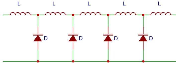
Figure 2.2.1: Non-linear transmission line representation with varactor diodes
