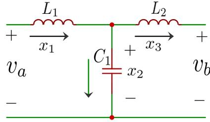
Figure 4.4.3: Lowpass equivalent circuit with state variables
