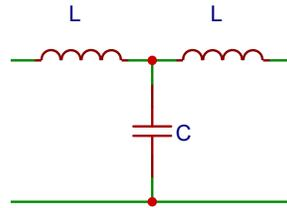
Figure 4.4.1: Unit cell of low-pass transmission line model
