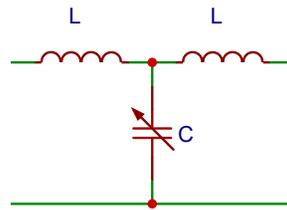
Figure 4.4.2: Unit cell of low-pass transmission line with non-linear capacitor
