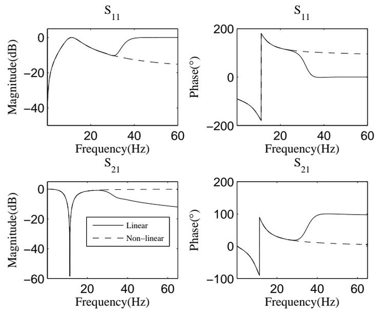
Figure 5.3.11: Scattering matrices for highpass equivalent circuit with non-linear inductor Miller loading
