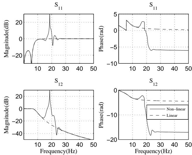
Figure 4.4.10: Scattering matrices of the unit cell with inductor as non-linear
