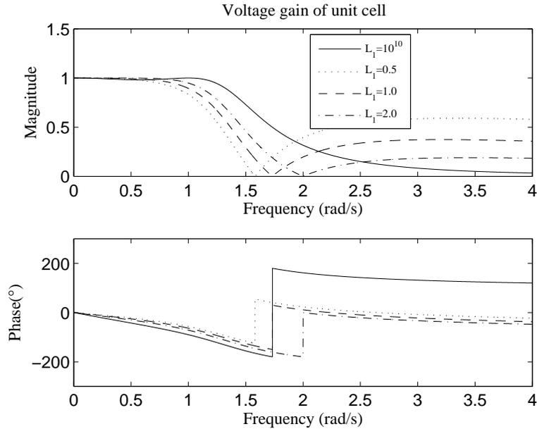
Figure 5.3.2: Voltage gain of unit cell with inductive loading
