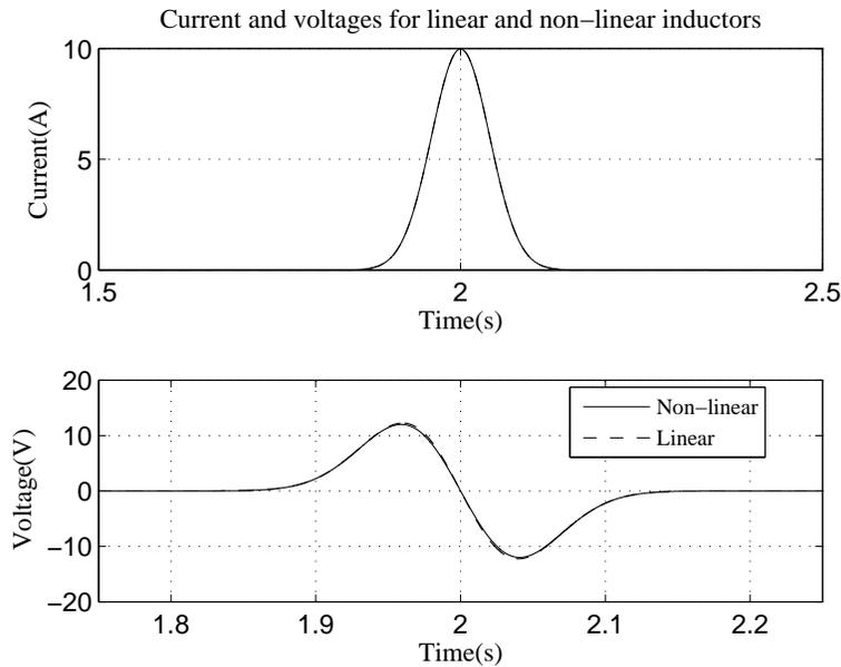
Figure 3.2.2: Time domain signals applied for linear and non-linear inductor.
