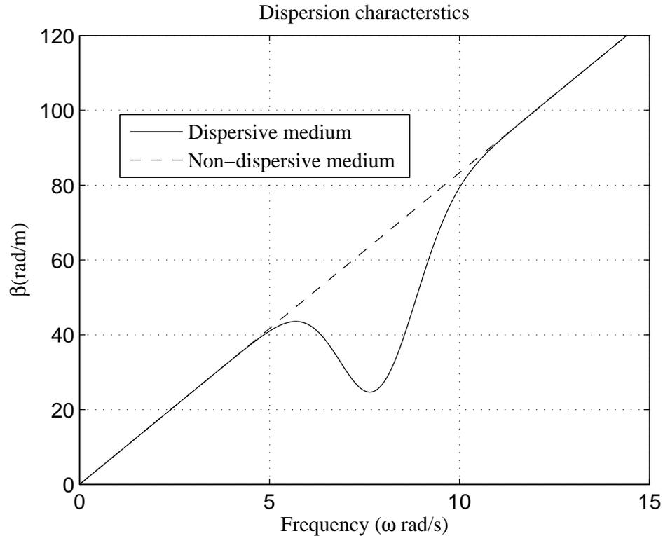
Figure 1.3.1: Typical variations in phase constants ( $\beta$ ) for dispersive and non-dispersive media
