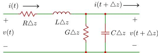
Figure 2.1.2: Equivalent circuit model of transmission line of differential length  $dz$
