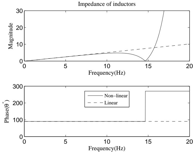
Figure 3.2.4: Impedance of non-linear and linear inductors.
