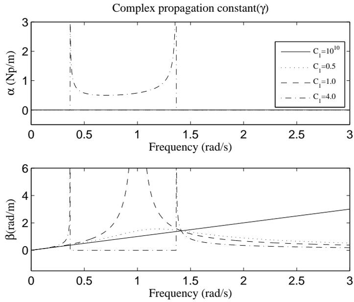
Figure 5.3.8: Complex propagation constant for lowpass Miller capacitive loading
