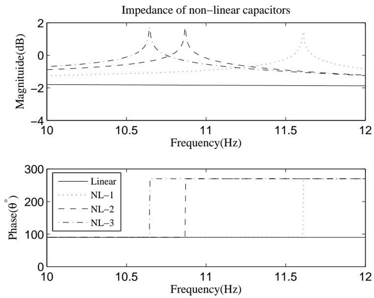
Figure 3.3.5: Changes in self resonating frequency with non -linearity
