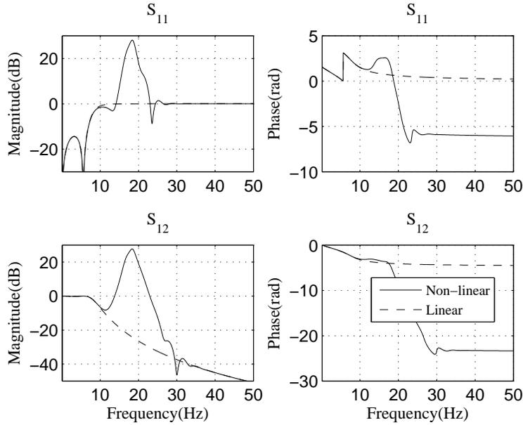
Figure 4.4.6: Scattering matrices of unit cell
