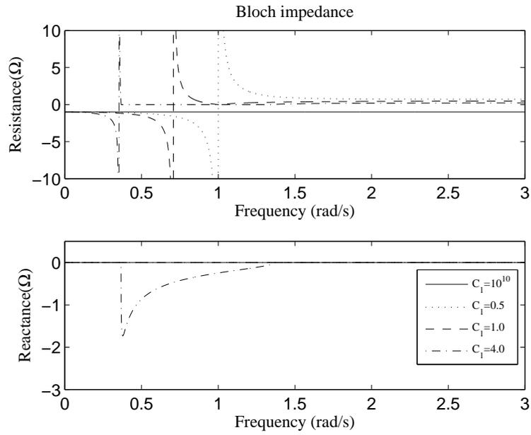
Figure 5.3.7: Bloch impedance of unit cell of Miller capacitive loading
