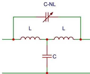
Figure 5.3.5: Unit cell of lowpass transmission line with Miller capacitive loading
