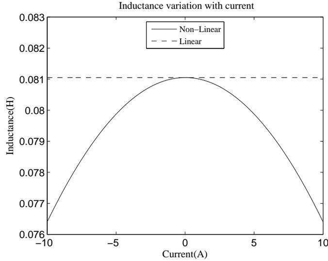
Figure 3.2.3: Variation of inductance with applied current.
