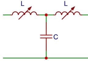
Figure 4.4.9: Unit cell of low-pass transmission line with non-linear inductors
