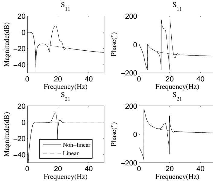
Figure 5.2.2: Scattering parameters for the unit cell of highpass equivalent circuit model with non-linear inductor
