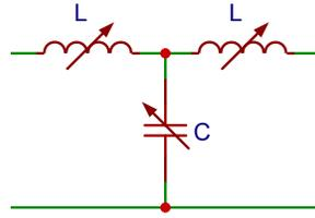
Figure 4.4.12: Unit cell of low-pass transmission line with non-linear elements
