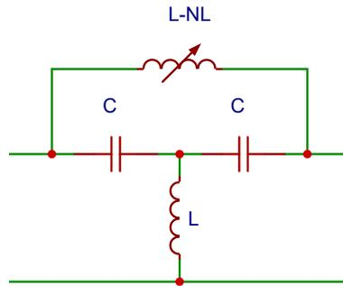
Figure 5.3.10: Highpass equivalent circuit with non-linear inductor Miller loading
