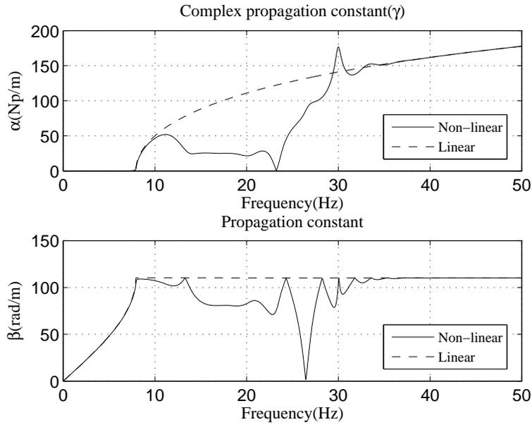
Figure 4.4.7: Complex propagation constant with non-linear capacitor
