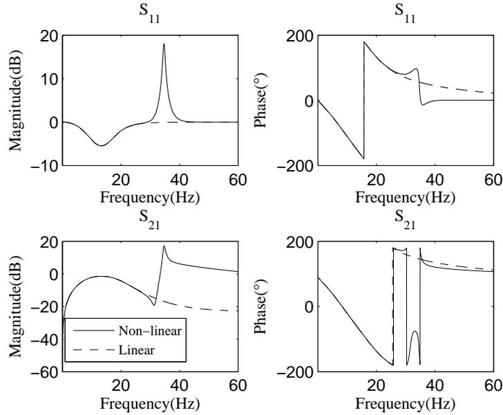
Figure 5.3.9: Scattering matrices for the lowpass Miller non-linear capacitive loading
