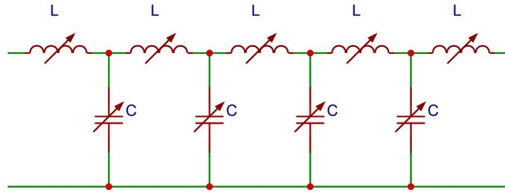
Figure 2.2.3: Considered non-linear transmission line in this thesis
