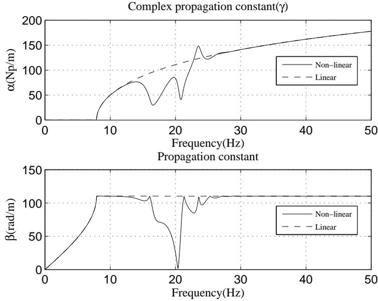
Figure 4.4.11: Complex propagation constant with series inductors as non-linear
