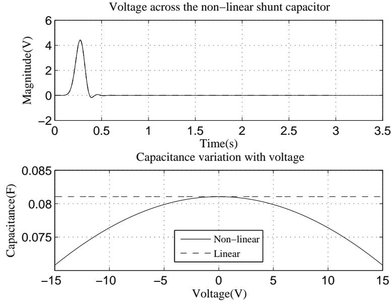
Figure 4.4.4: Variation of capacitance with applied voltage
