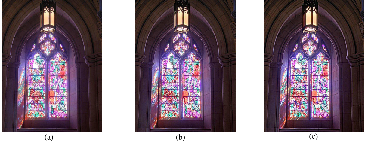
Figure 6.20: Visual inspection: The affect of free parameter r on detail enhancement. It is found that r=2 is sufficient for fine details extraction and gives better results for most cases. Higher value of r brings in artifacts near strong edges. (a); r=1 (b) r=3 ; and (c) r=6 .
