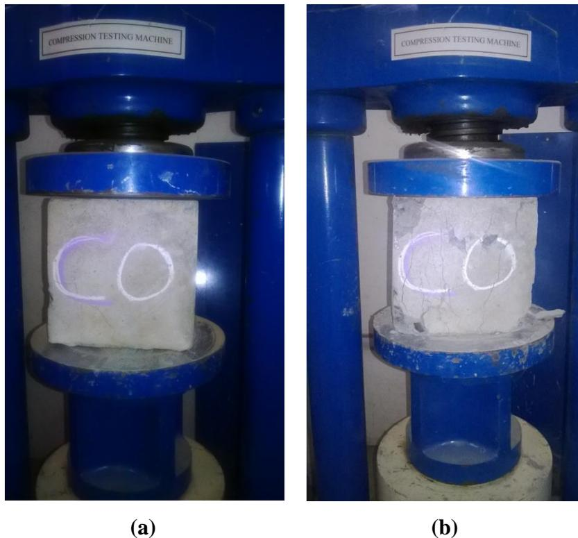
**Fig. 3.9 (a) and (b)** Concrete cubes kept in CTM before and after testing
