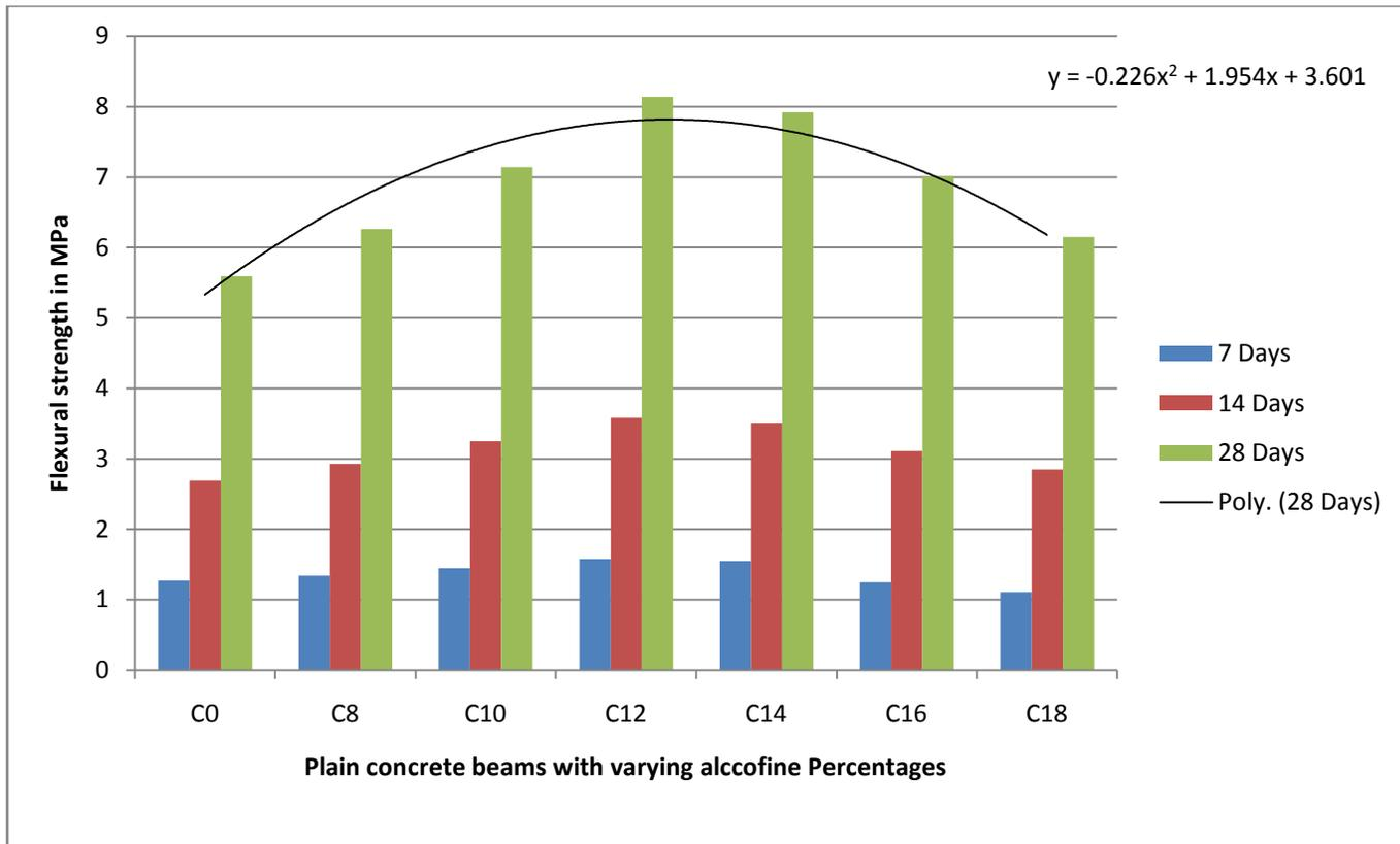
**Fig. 4.2:** Variation of Flexural strength of plain concrete beams with different % of alccofine
