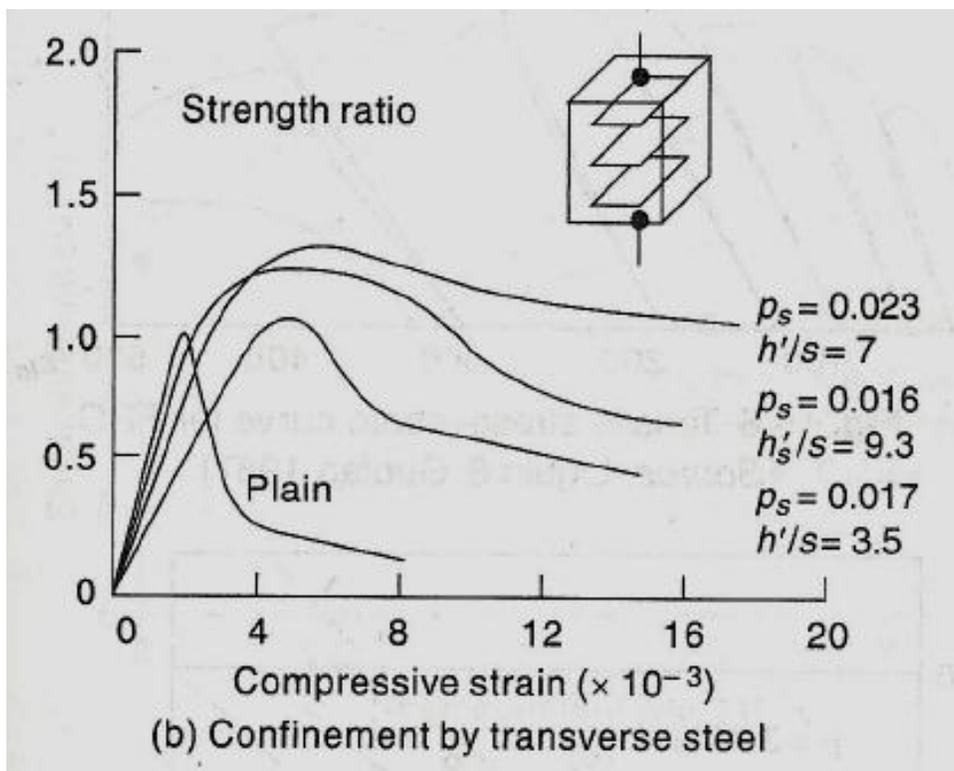
**Fig. 2.23:** Effect of fiber reinforcement and containment by transverse steel on compressive behavior of concrete (Source: V. Ramkrishna [120])
