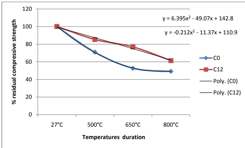
**Fig. 4.13:** Variation of % Residual compressive strength with varying temperature at 7days of curing
