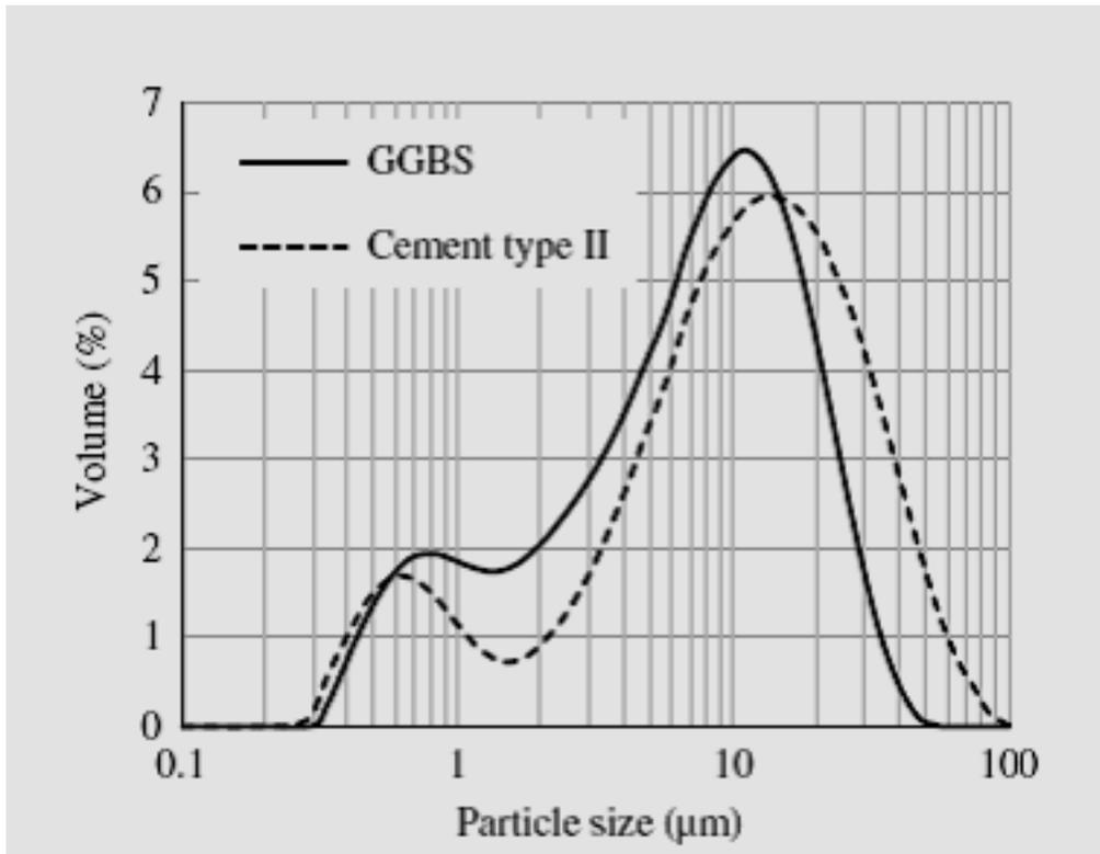
**Fig. 2.15:** (a) Particle size distribution of GGBS and cement
