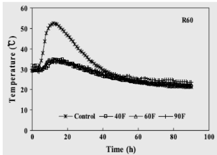
**Fig. 2.2:** Variation of temperature rise with fly ash (Source: Se Jin choi et al [25])
