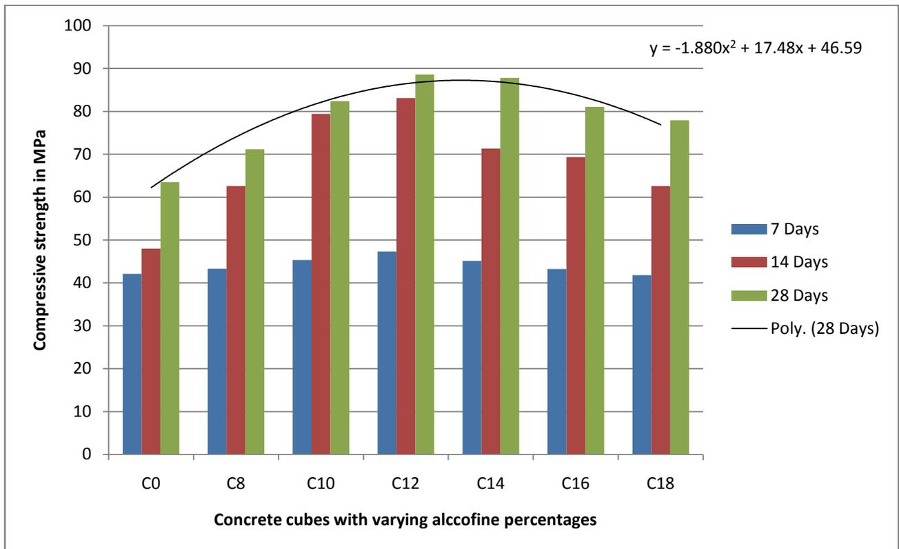
**Fig. 4.1:** Comparison of compressive strength of concrete cubes at 7, 14 and 28 days
