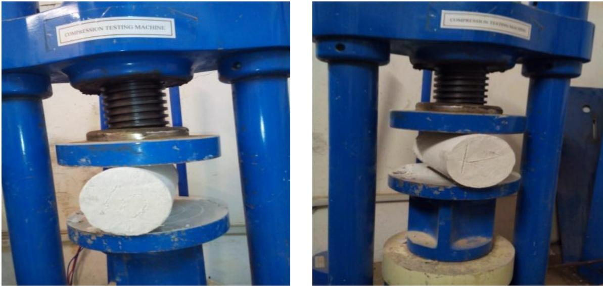
**Fig: 4.8:** Splitting tensile tests of cylindrical specimen
