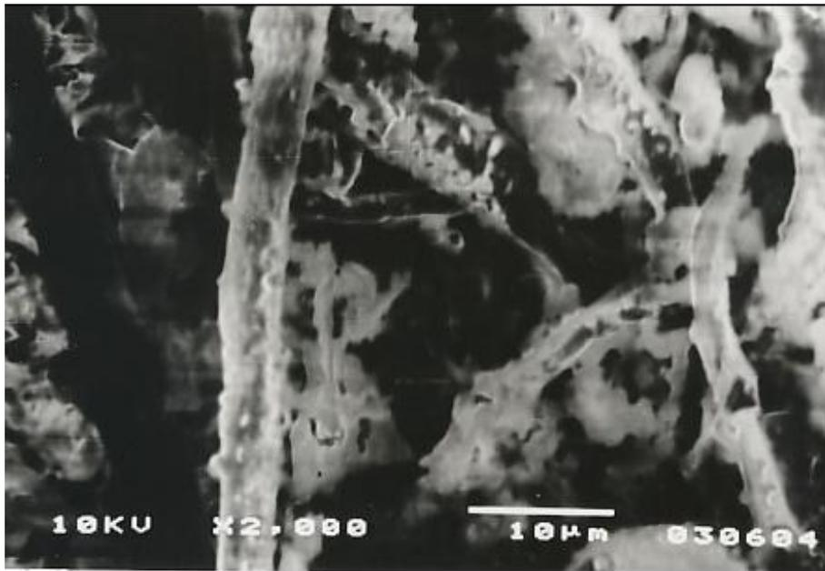
**Fig. 2.20:** SEM of Concrete with Hyper 2000 (Source: R.N. Krishna [152])
