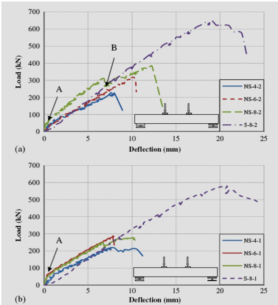
Fig. 2.8: Load-deflections of the beams: (a) HVFAC; (b) CC (Source: M. Arezoumandi et al [21])
