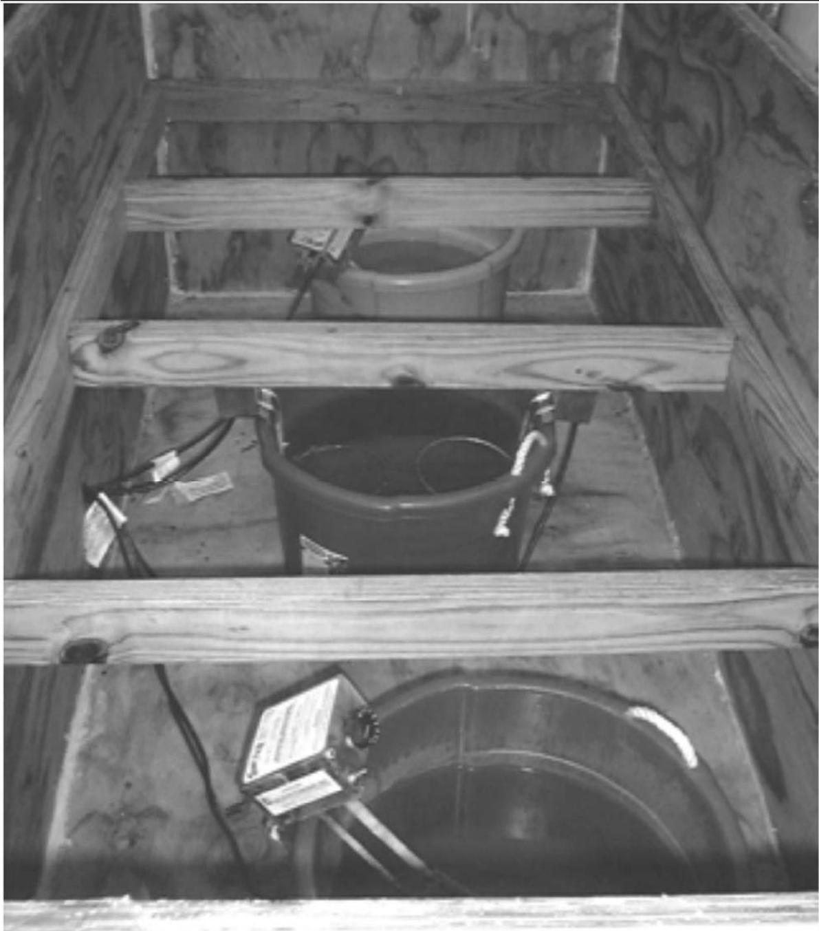
**Fig. 2.12:** Setup of heaters inside steam-curing chamber (Source: N. Yazdani et al [63])
