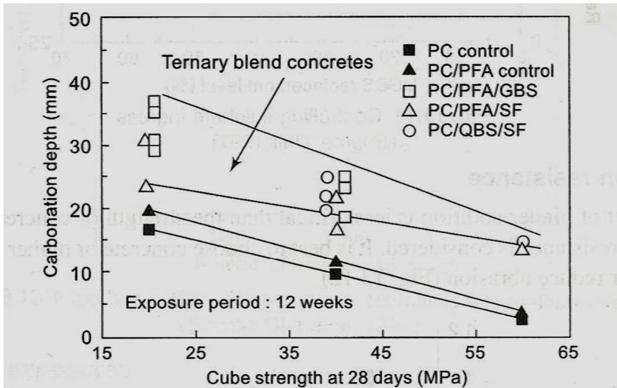
Fig. 2.30: Importance of concrete strength in controlling carbonation depth (Source: R. Jones et al [134])
