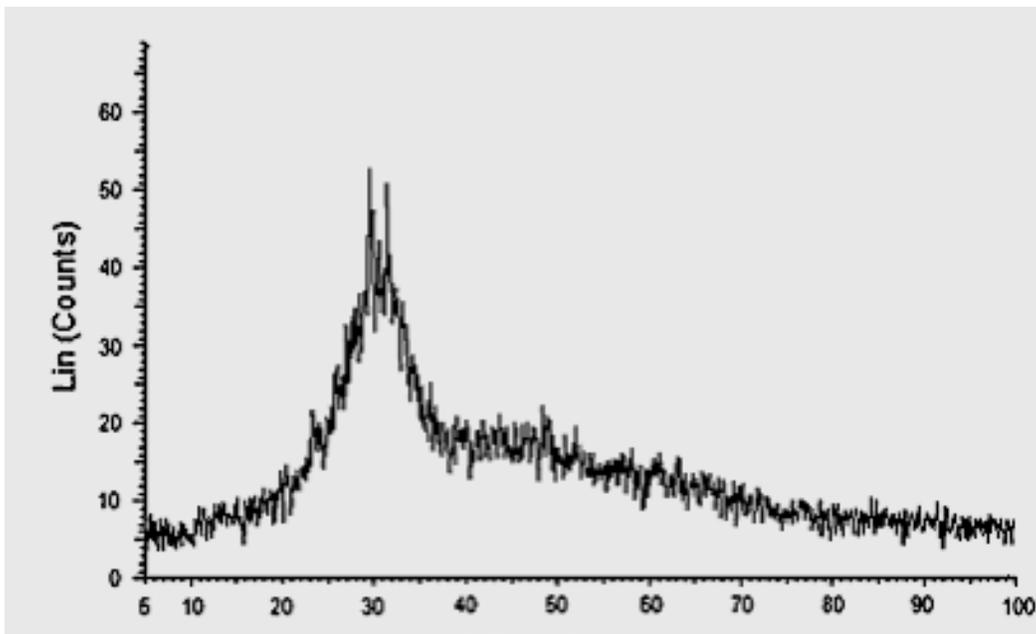
**Fig. 2.15:** (b) X-ray diffraction test on GGBS.
