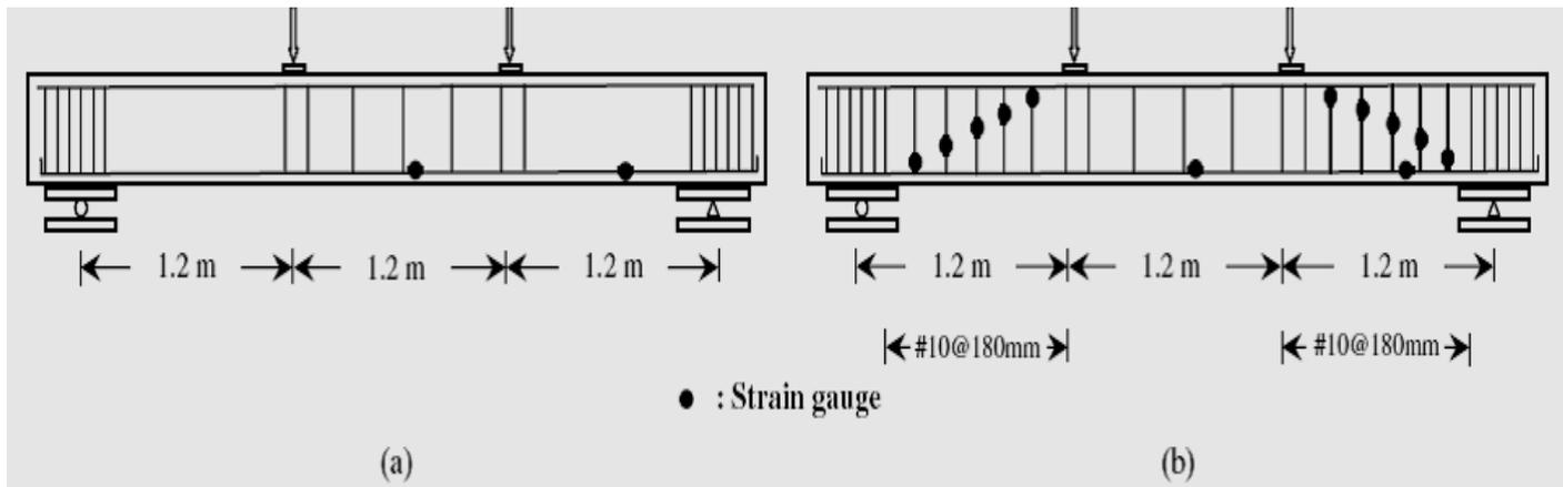
**Fig. 2.7:** Location of strain gauges on the test beams (a) Without stirrups on test region (b) with stirrups on test region (Source: M. Arezoumandi et al [21])
