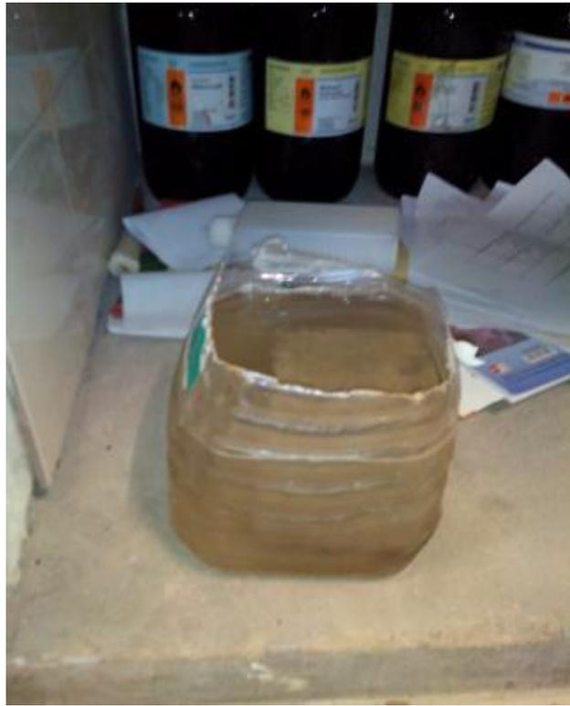
**Fig. 4.16:** Concrete cubes kept for curing in 100% H<sub>2</sub>O
