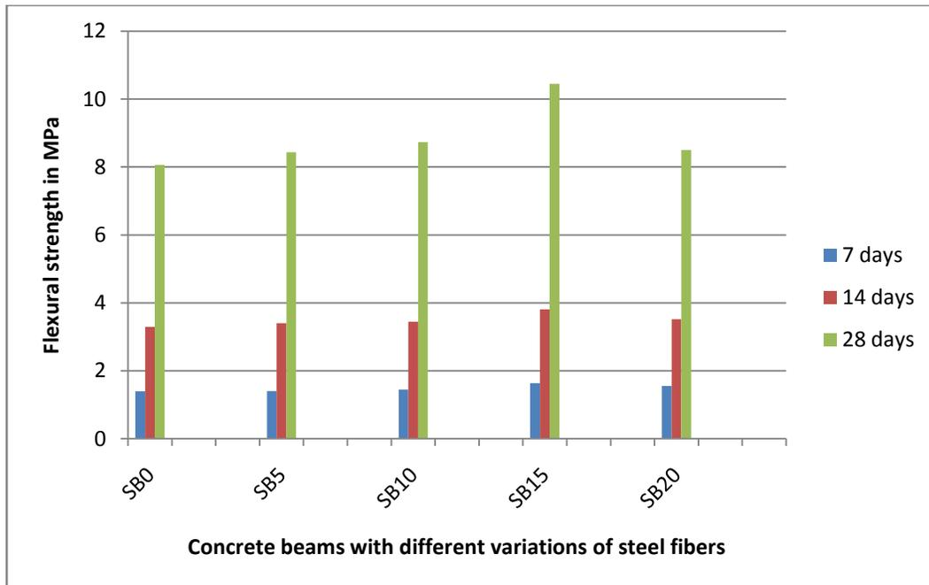
**Fig. 4.10:** Comparison of flexural strength of concrete beams with different variations of steel fibers.
