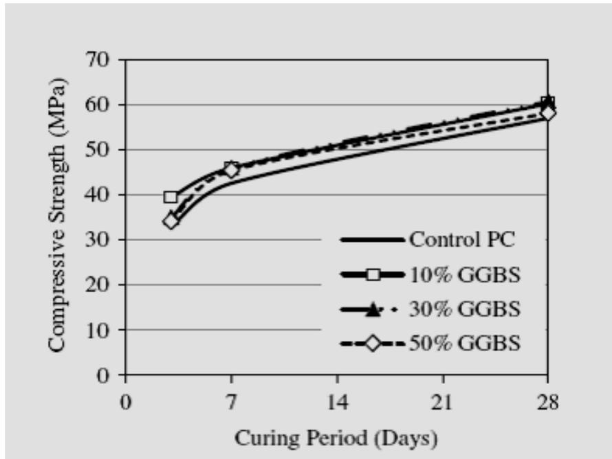
**Fig. 2.16:** Effect of GGBS replacement on compressive strength (Source: B.S. Divsholi et al [5])
