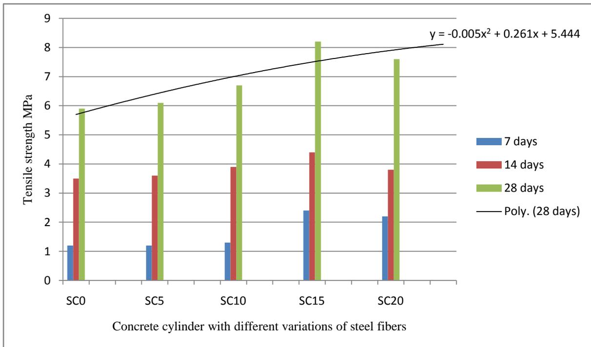
**Fig. 4.7:** Concrete comparison of tensile strength of concrete cylinders with different variations of steel fibers.
