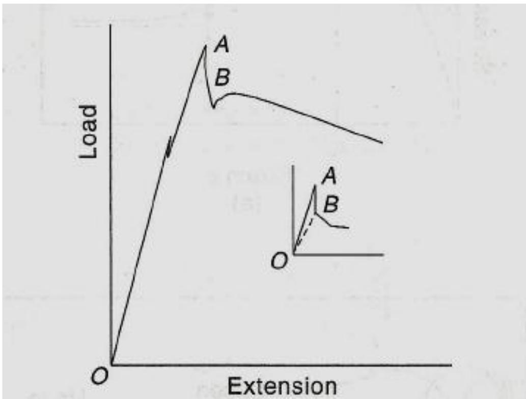
**Fig. 2.22:** Typical load extension curve for fiber pull out test (Source: A. Kelly [130] )
