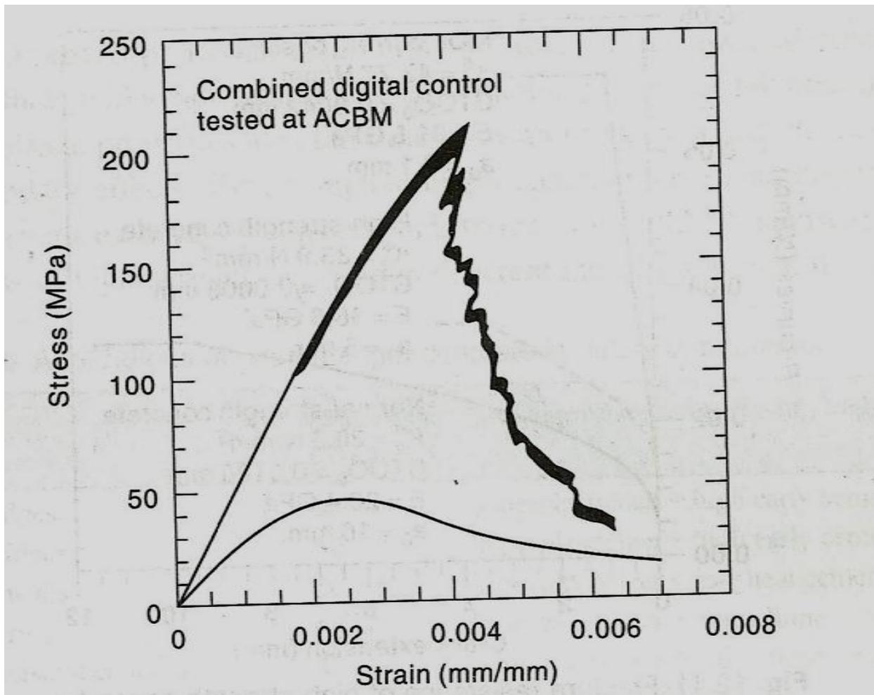
**Fig. 2.28:** Stress strain curve for ultra high strength concrete. (Source: S.P. Shah and S.H. Ahmed [155] )
