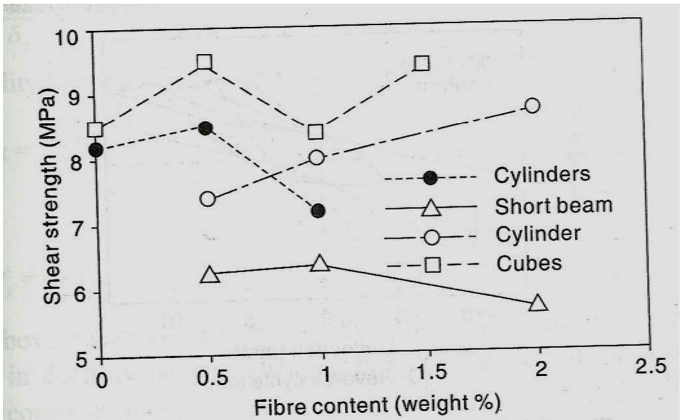
Fig. 2.25: Shear strength of SFRC (Source: B. Barr [121])
