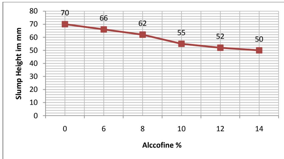
**Fig. 3.6:** Graphical variation of slump with variable percentages of alccofine
