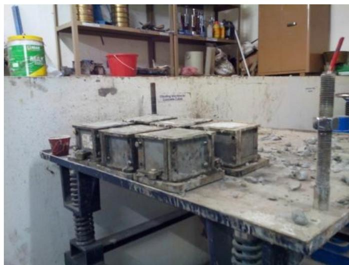
**Fig. 3.4:** Sample of cubes kept on vibration table for compaction
