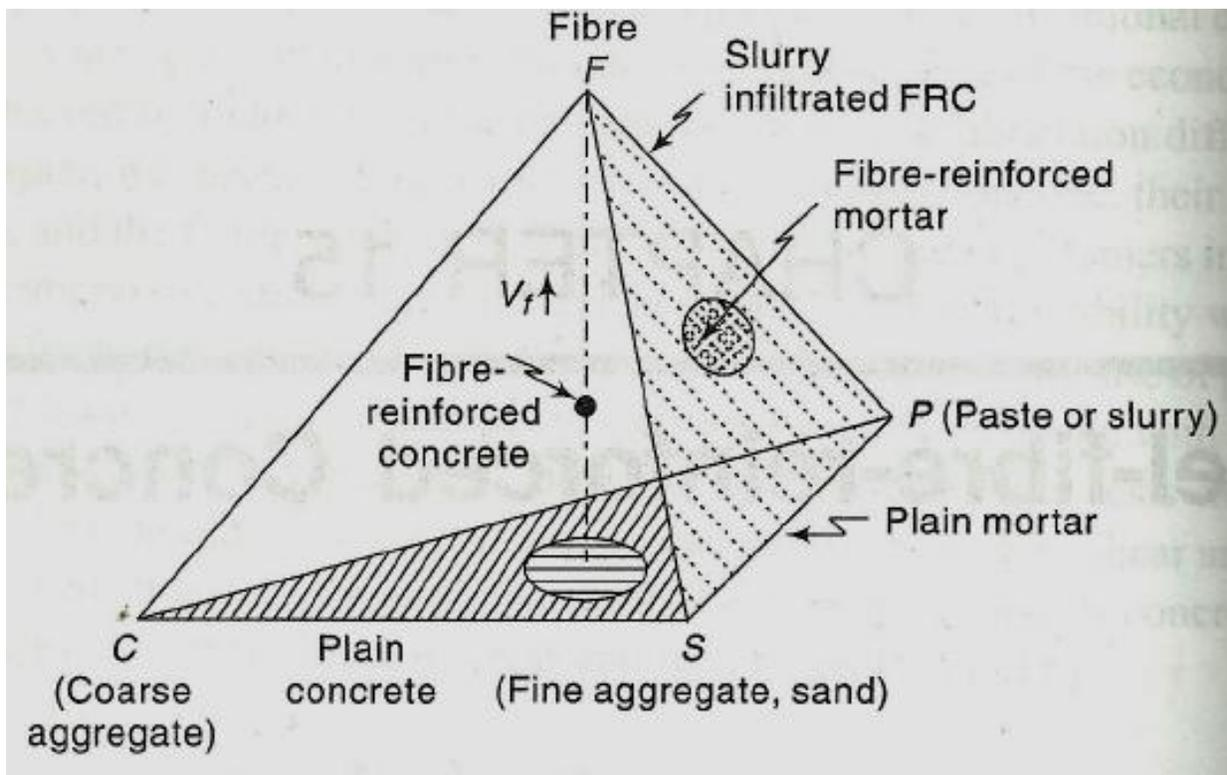
**Fig. 2.21:** Four phase representation of FRC (Source: A. R. Shantakumar [137])
