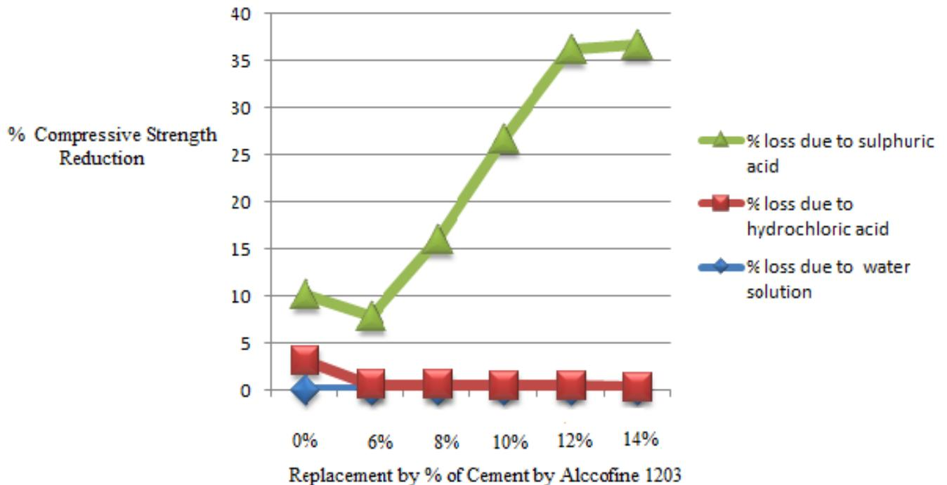
Fig. 4.17: Reduction in compressive strength of concrete cubes cured under different solutions
