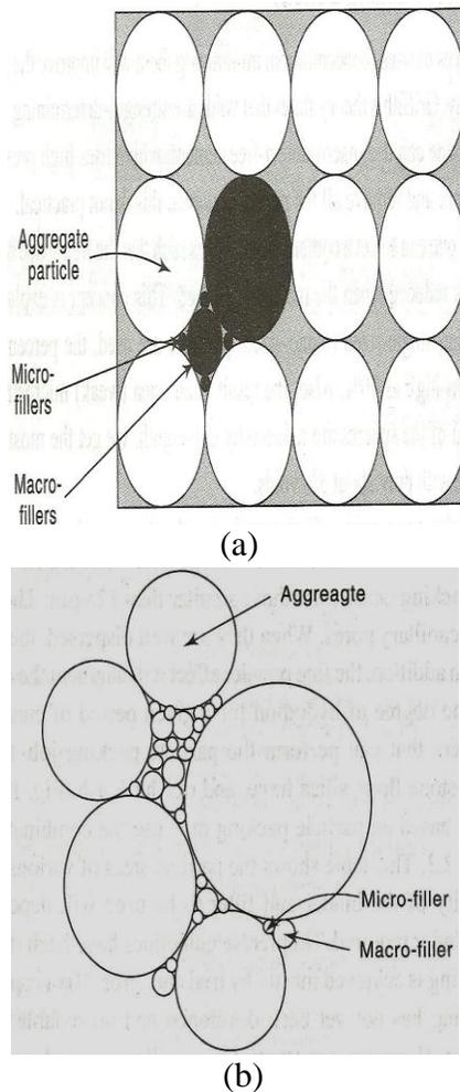
**Fig. 1.5:** (a) Concept of particle packing, (b) effect of fillers between aggregate particles (Source: A.R. Santhakumar [137])
