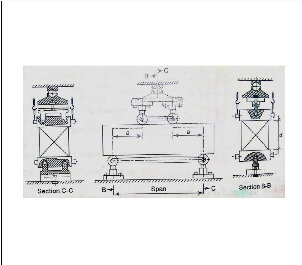
**Fig. 3.10:** Arrangement for loading of flexural test specimen
