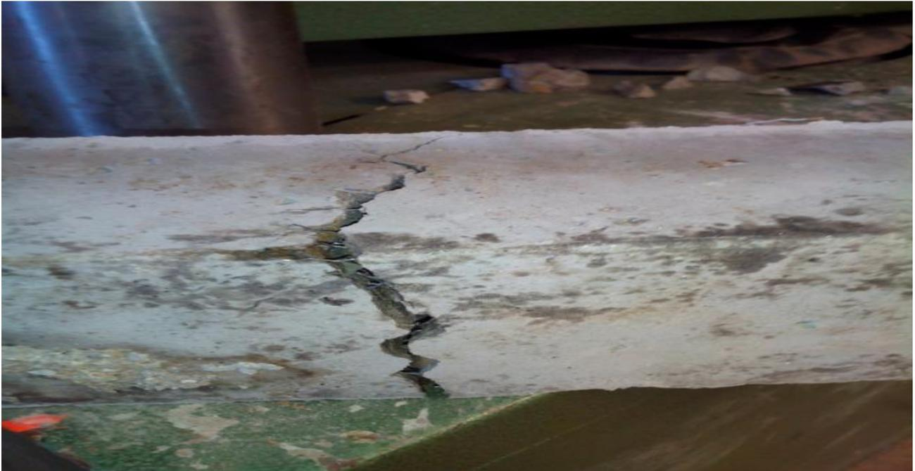
**Fig. 4.9:** SFRC beam after flexural testing
