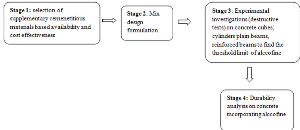
Fig. 3.3: Layout of experimental program
