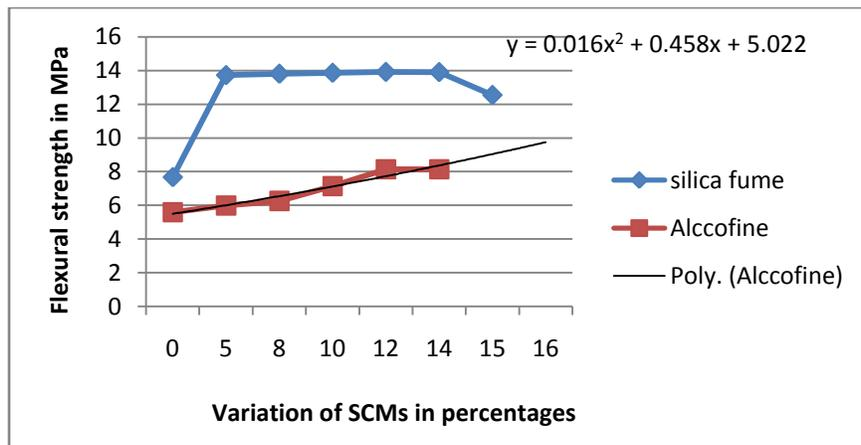
**Fig. 4.19:** Comparison of Flexural strength results
