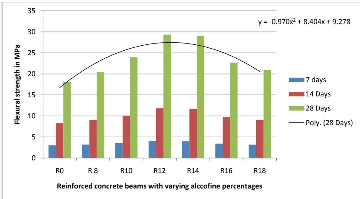
**Fig. 4.3(b):** Variation of Flexural strength of Reinforced concrete beams with different % of alccofine
