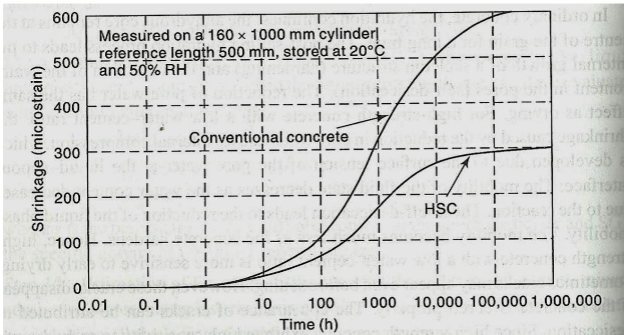
**Fig. 2.27:** Shrinkage of high strength concrete (Source: R.K. Dhir [110])
