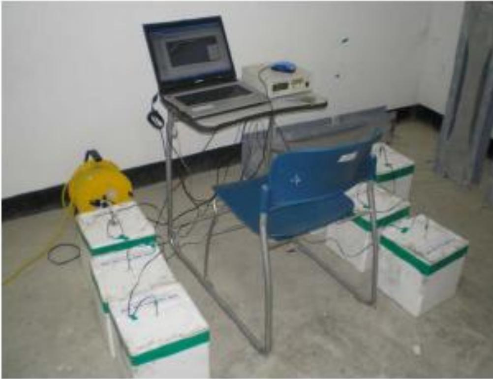
**Fig. 2.1:** Test of measuring temperature change of mortars (Source: S. J. Choi et al [25])
