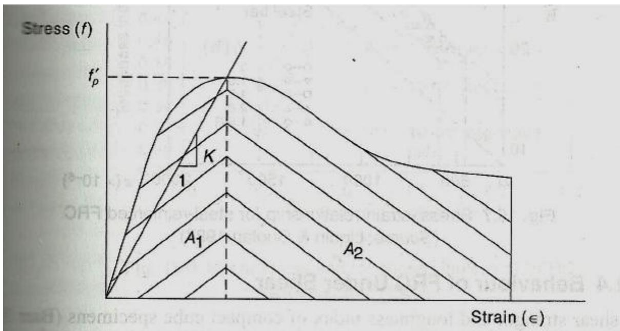
**Fig. 2.24:** Characteristics of compressive stress strain relationship of concrete and fiber reinforced concrete (Source: V. Ramkrishna [120])
