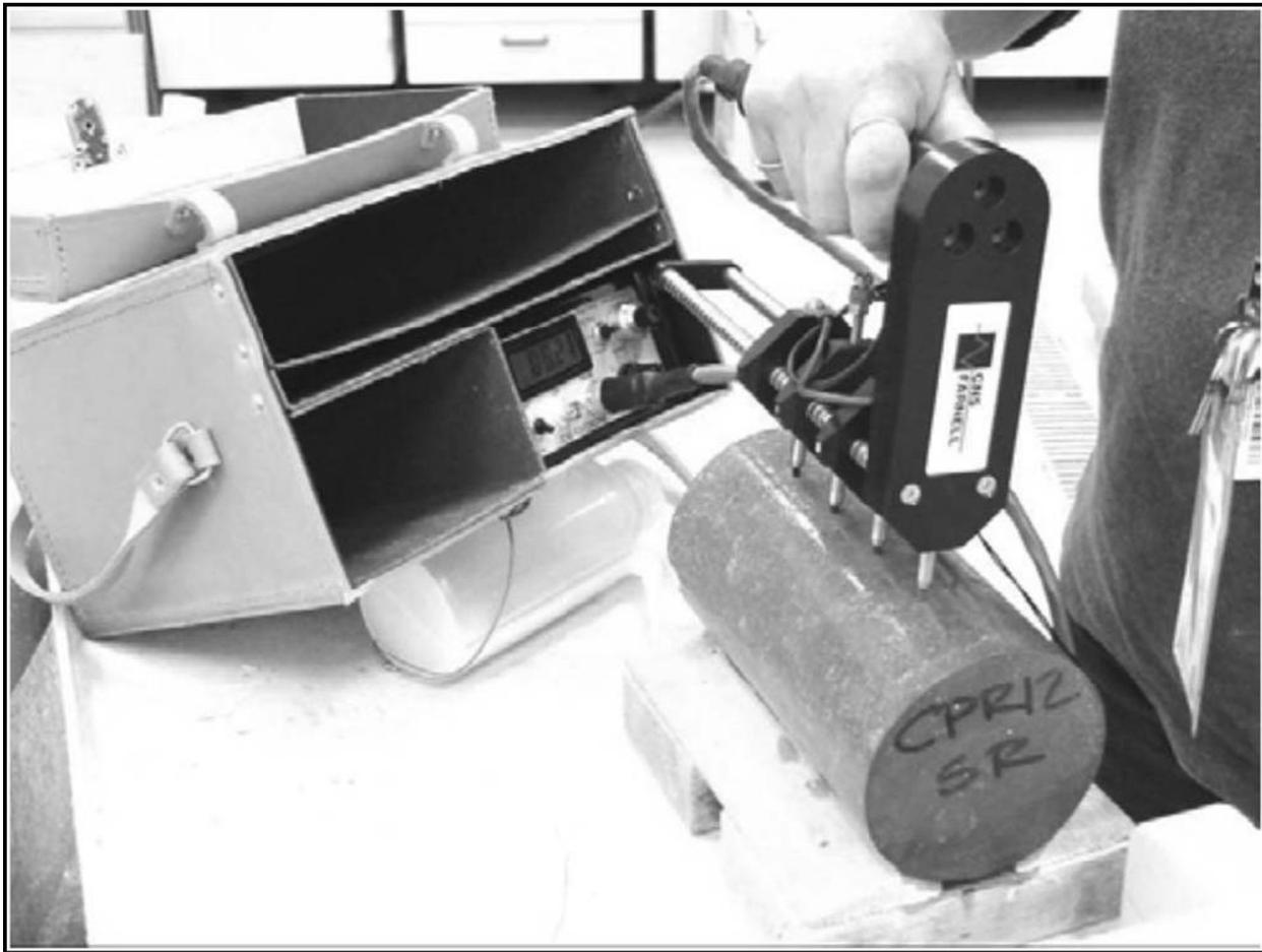
**Fig. 2.13:** Surface resistivity test using Wenner array (Source: N. Yazdami et al [63])
