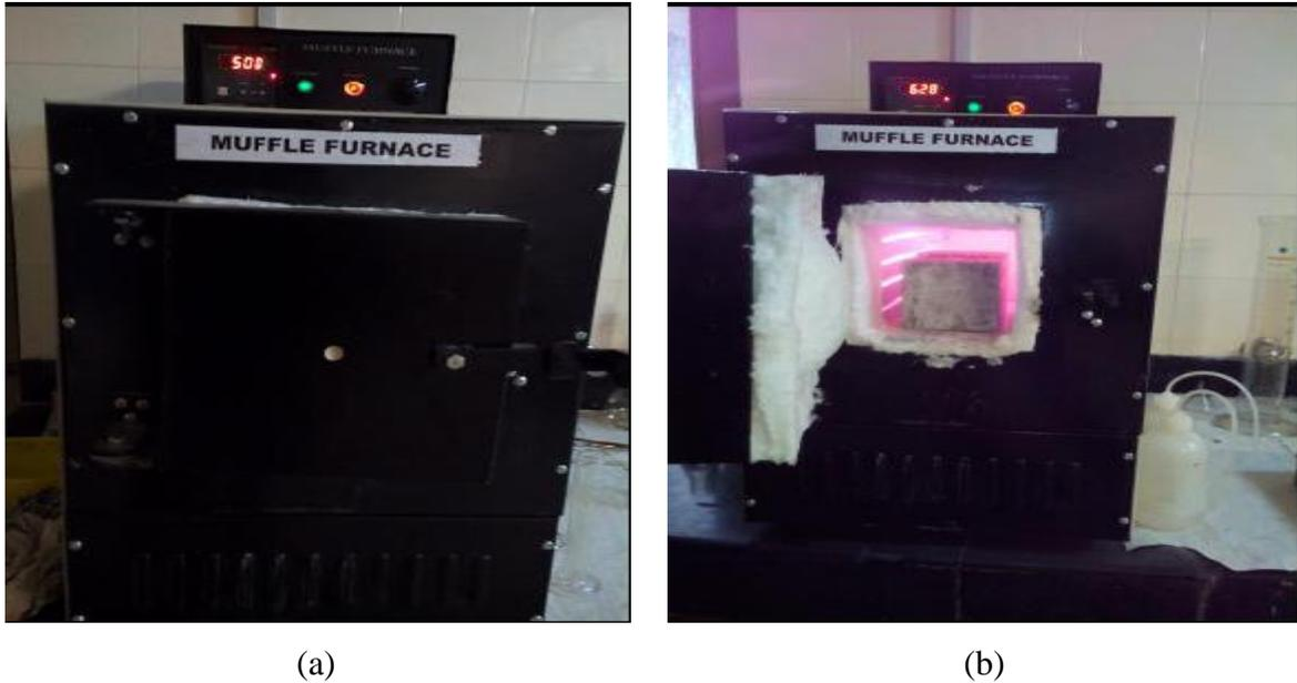
**Fig. 3.12:** Cubes incorporating ultrafine slag at varying temperatures placed in muffle furnace
