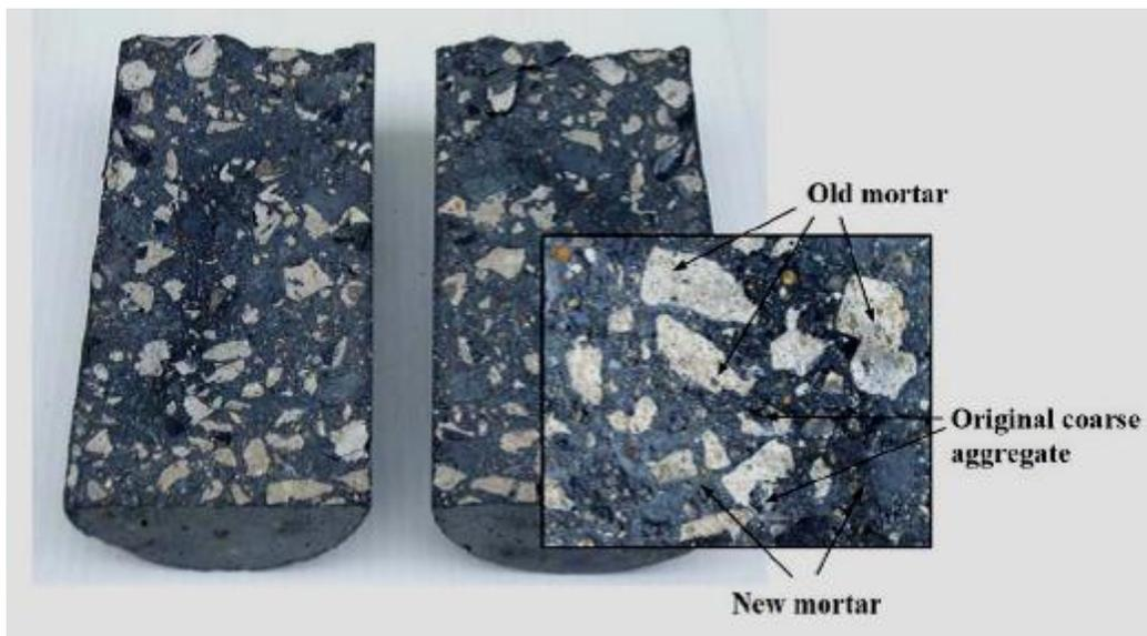
**Fig. 2.6:** Failure of recycled aggregate concrete after Splitting tensile test (Source: W. Tangchirapat et al [12])
