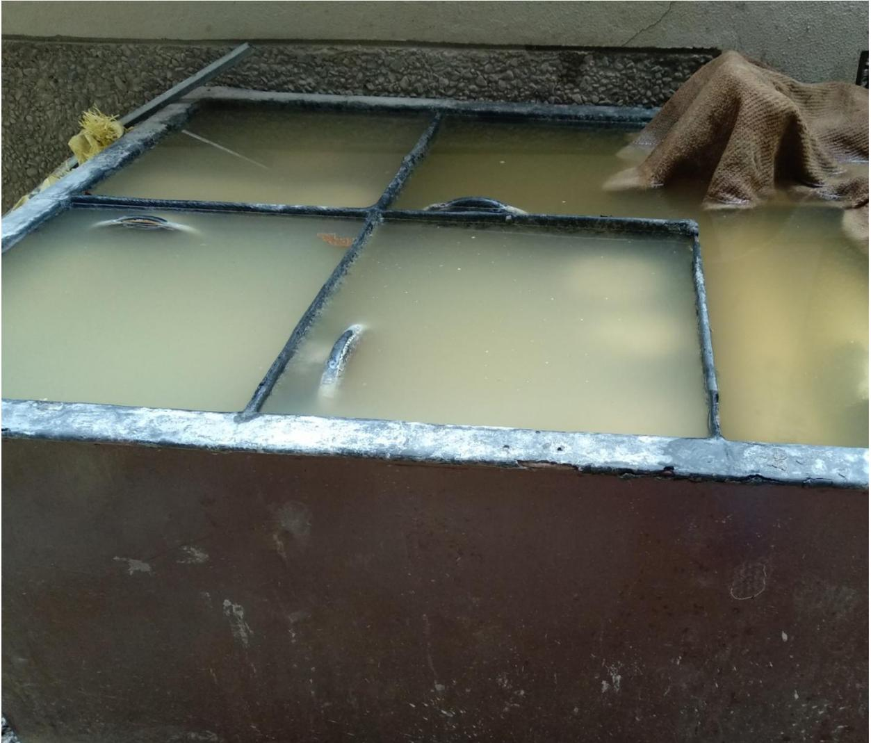
**Fig. 3.5:** Curing of specimens
