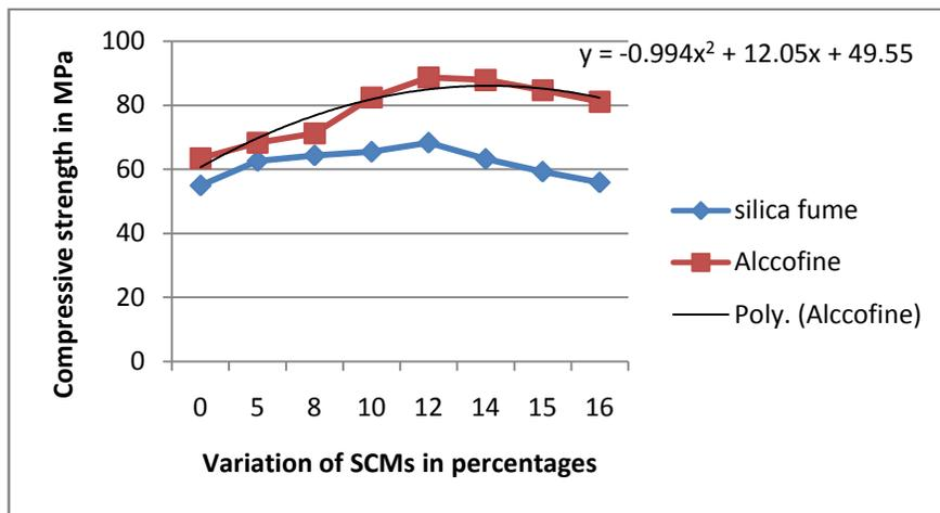
**Fig. 4.18:** Comparison of compressive strength results
