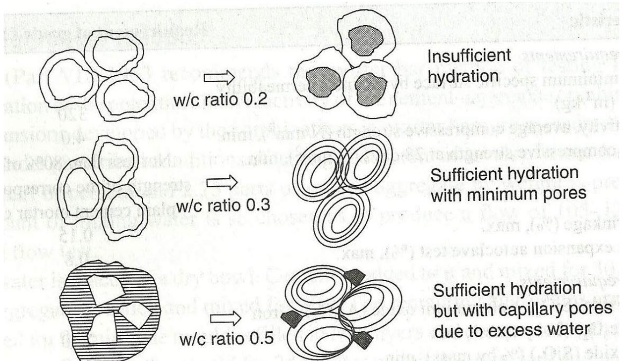
**Fig. 3.2:** Schematic representation of insufficient, sufficient and excess water for hydration
