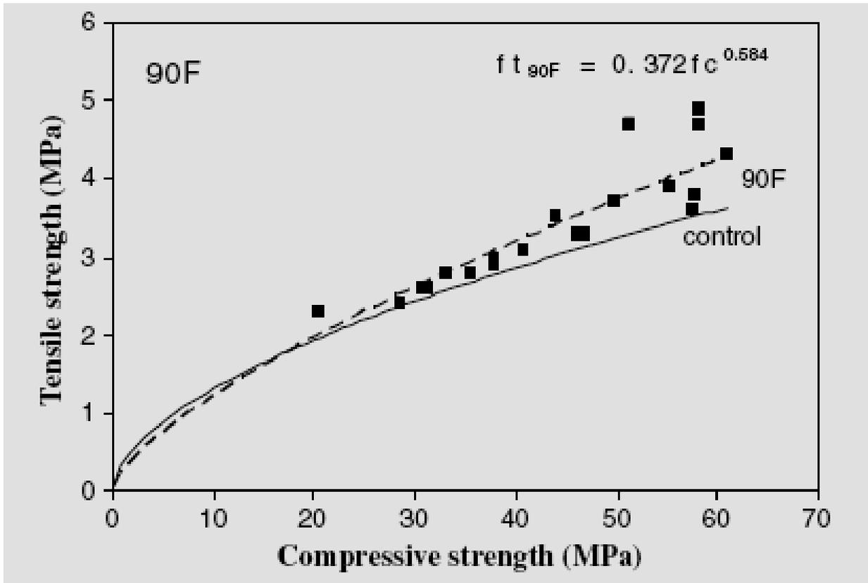
Fig. 2.4: Relation between compressive strength and tensile strength (Source: S. J. Choi et al [25])
