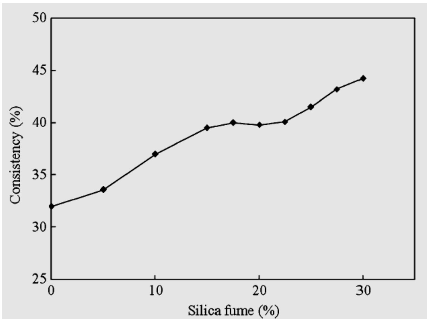
**Fig. 2.14:** Variation of consistency of cement pastes containing different percentages of silica fume
