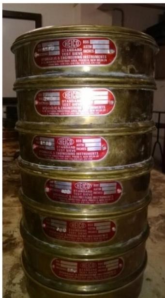
**Fig. 3.1:** IS sieves for sieve analysis
