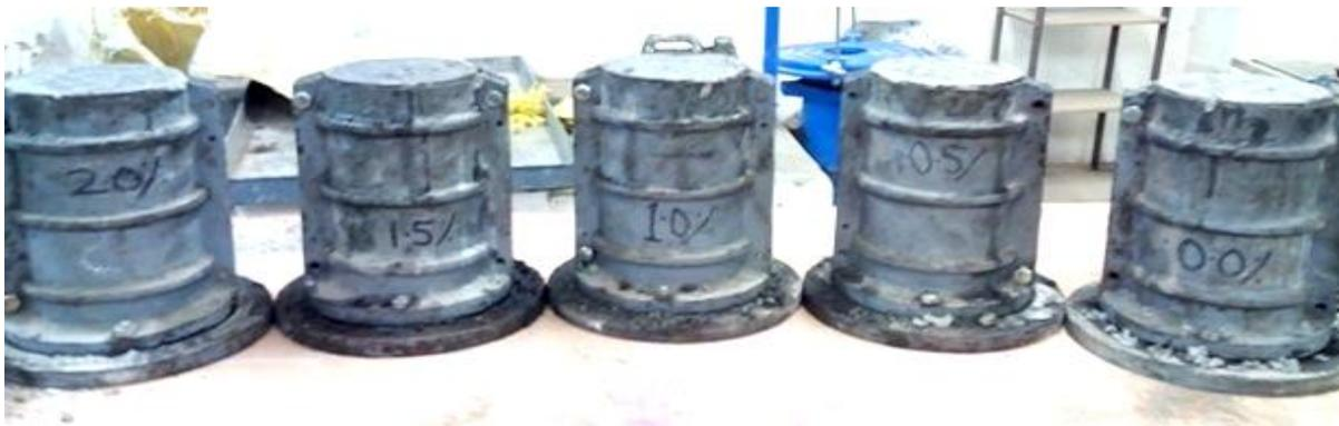
**Fig. 4.5:** Concrete cylinders with varying % of steel fibers.
