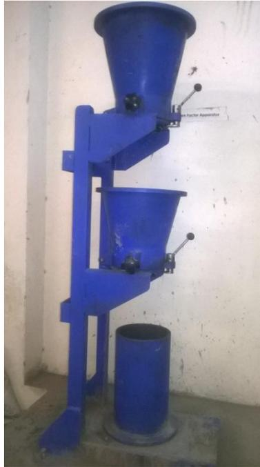
**Fig. 3.7:** Compacting Factor apparatus
