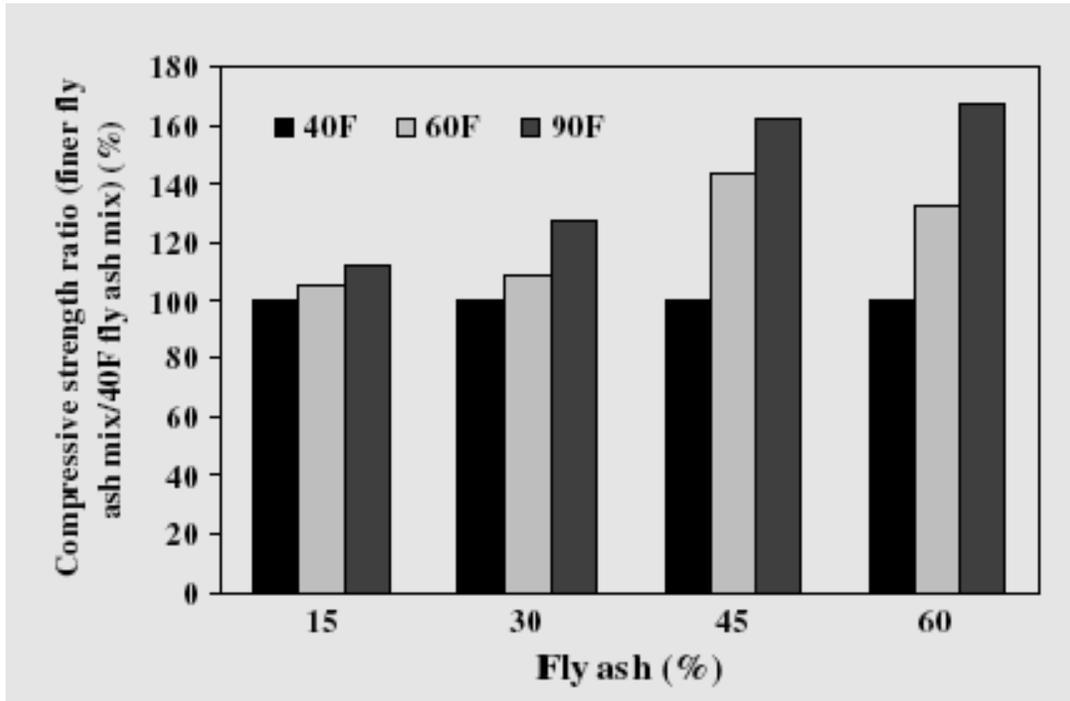
Fig. 2.3: Compressive strength ratio with fly ash fineness at 28 days (Source: Se Jin choi et al [25])
