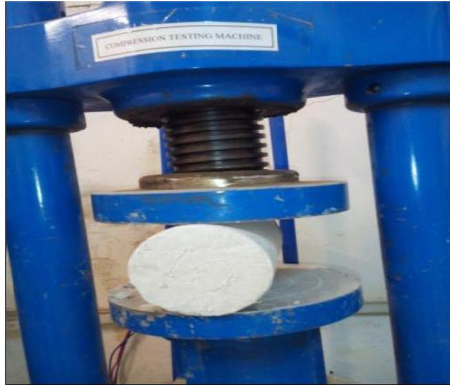
**Fig. 3.11:** Splitting tensile test
