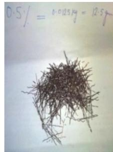
(a) 0.5% steel fibers of total volume fraction of concrete
