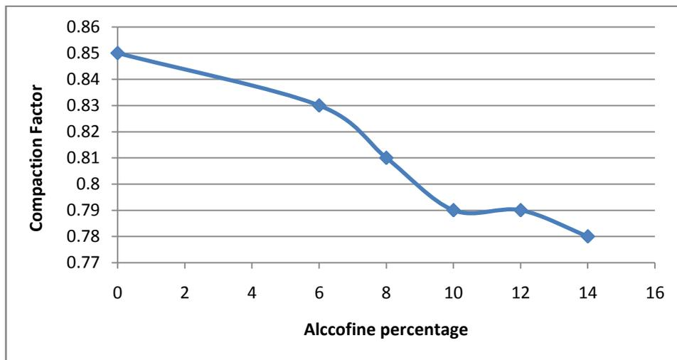
**Fig. 3.8:** Compaction factor test result
