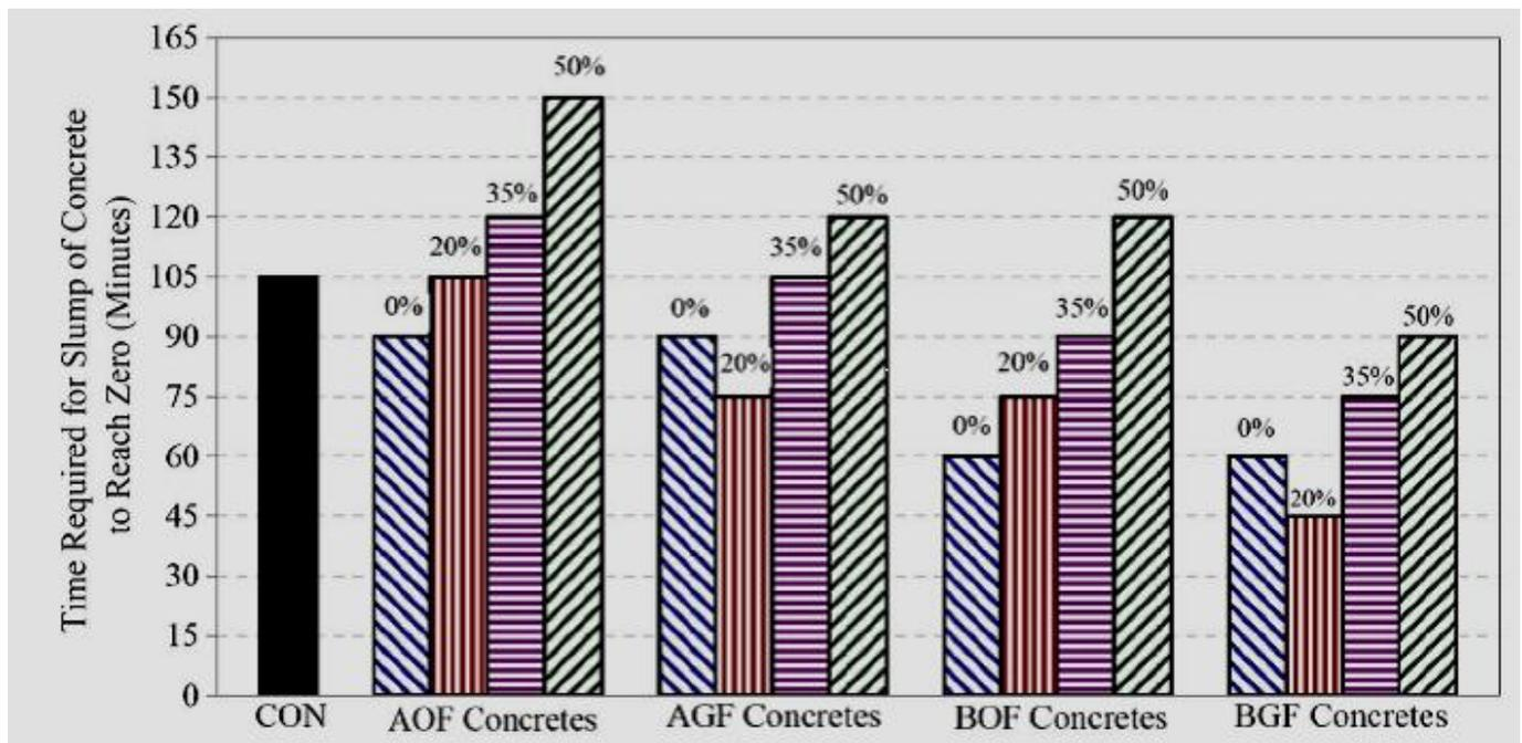
**Fig. 2.5:** Slump loss concrete containing recycled aggregates (Source: W. Tangchirapat et al [12])
