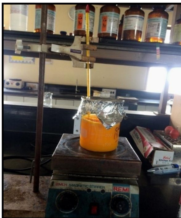
Figure 2.1: Experimental setup used to synthesize CdSe QDs
