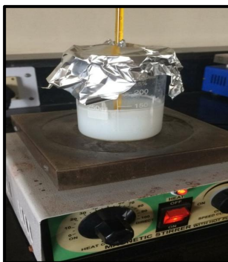
Figure 2.4: Experimental setup used to synthesize ZnS QDs
