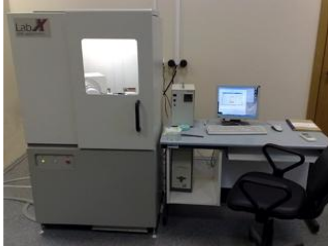
Figure 2.7: Shimadzu (XRD 6000) X-Ray diffractometer employed for XRD experiments
