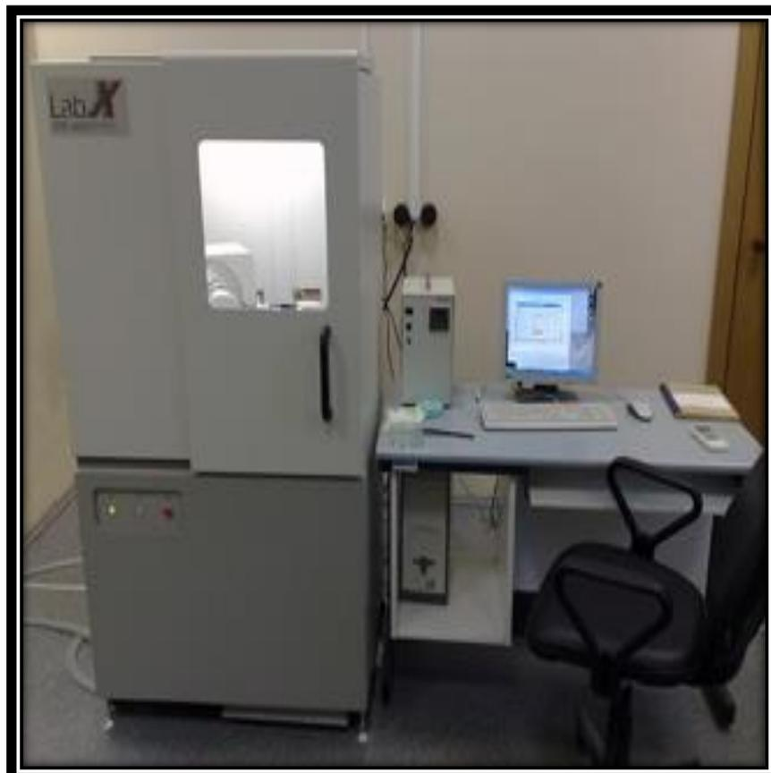
**Figure 2.3:** SHIMADZU analytical: XRD 6000 diffractometer.
