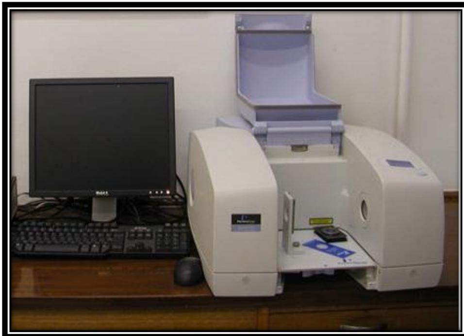
**Figure 2.4:** Perkin Elmer spectrophotometer (model-65).
