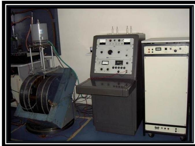
**Figure 2.6:** Vibrating sample magnetometer (PAR-155).
