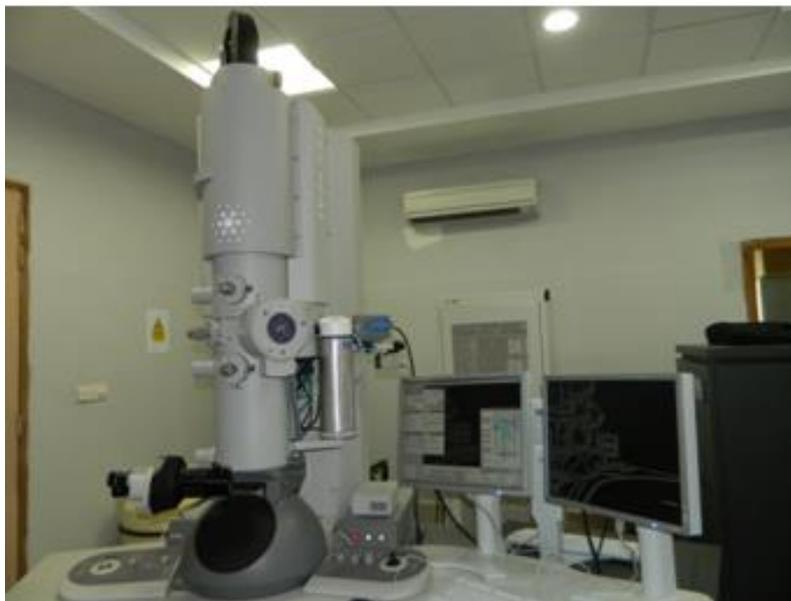
**Figure 2.8:** Transmission electron microscope used for morphology analysis.
