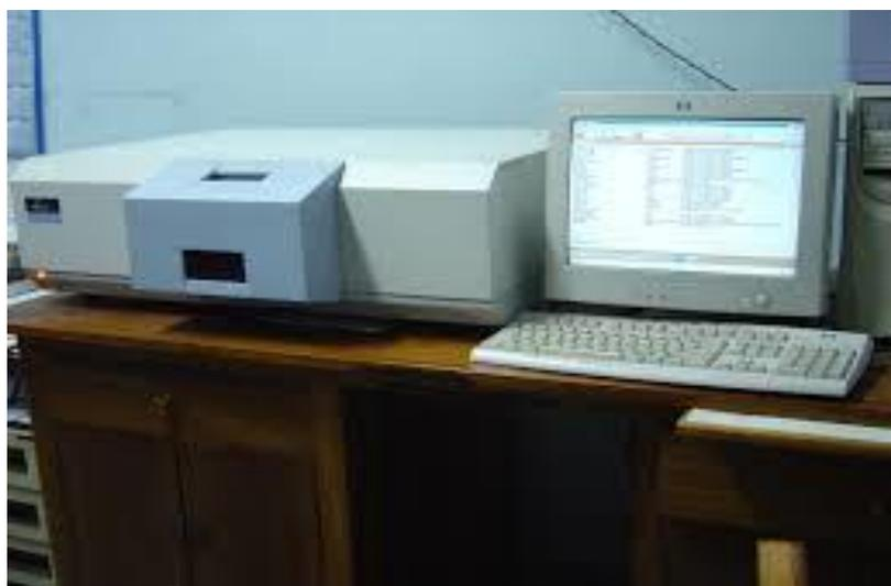
**Figure 2.11:** FTIR photograph used for the analysis of QDs.
