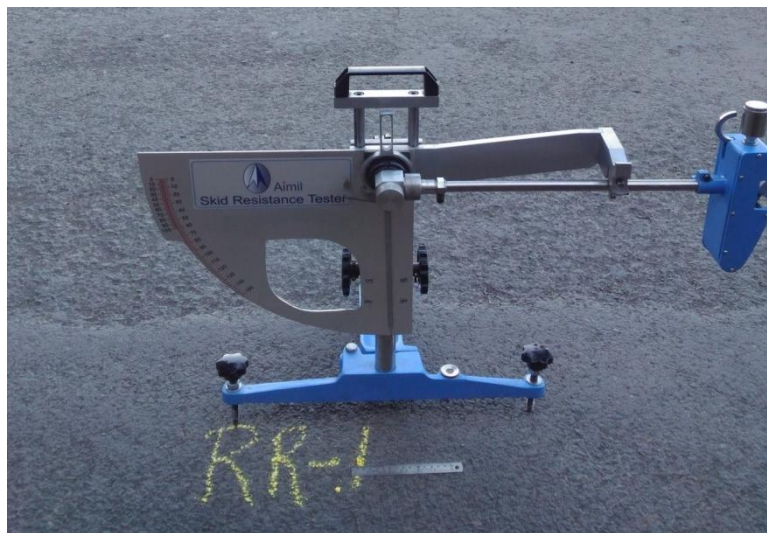
Figure 3.12 Skid Resistance Test conducted on RR-1
