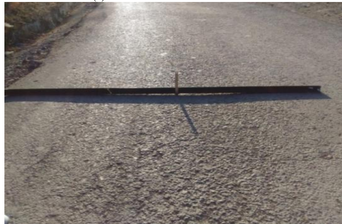
(b) Measurement of Rutting using straight edge
