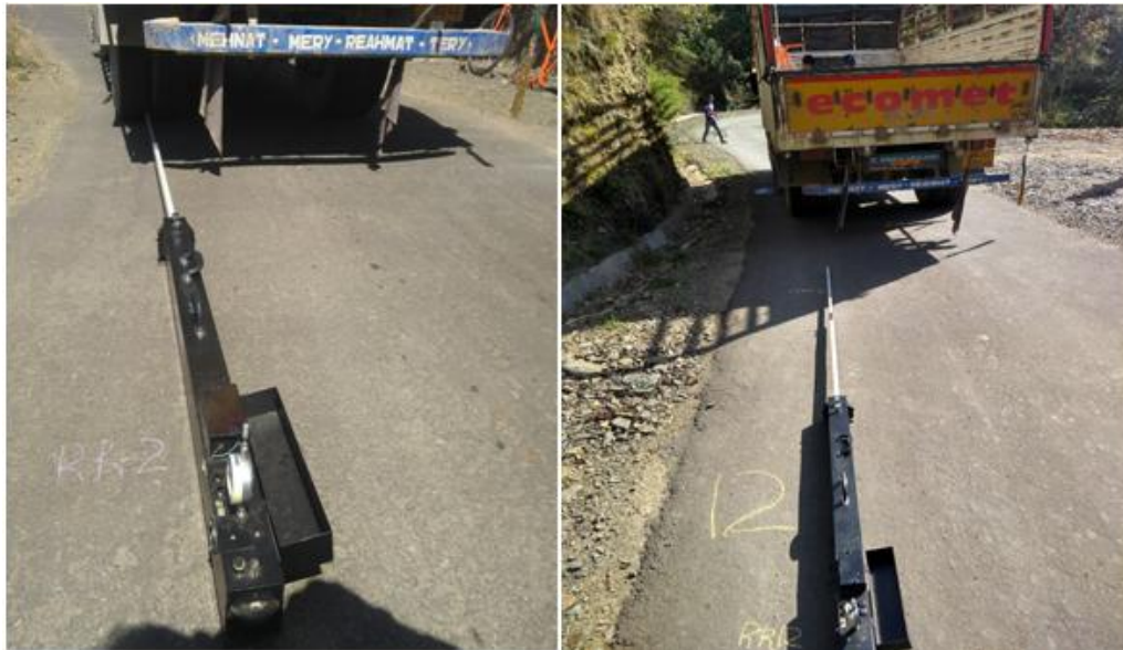
Figure 3.13 Benkelman Beam Deflection study on selected stretches (RR-2 and RR-12)
