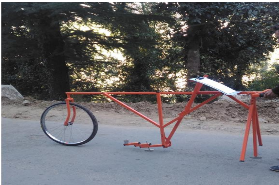
Figure 3.5 MERLIN test conducted on RR-6
