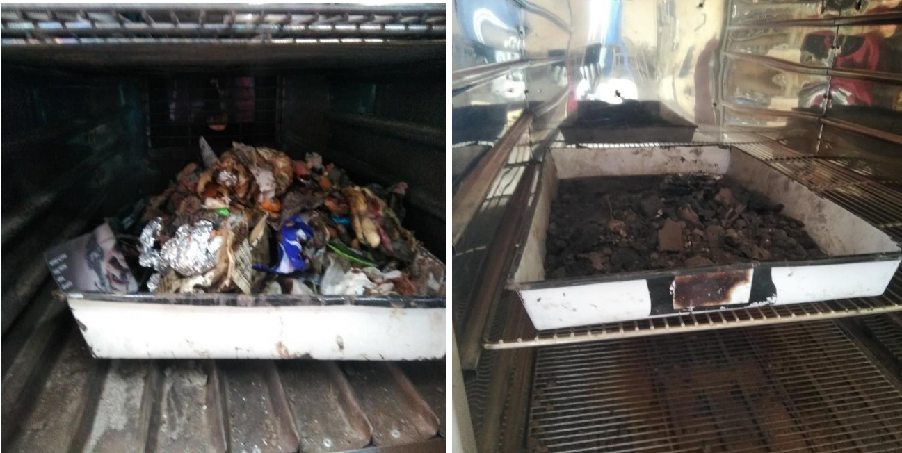
Figure 5.2: Moisture content determination of fresh and degraded MSW.
