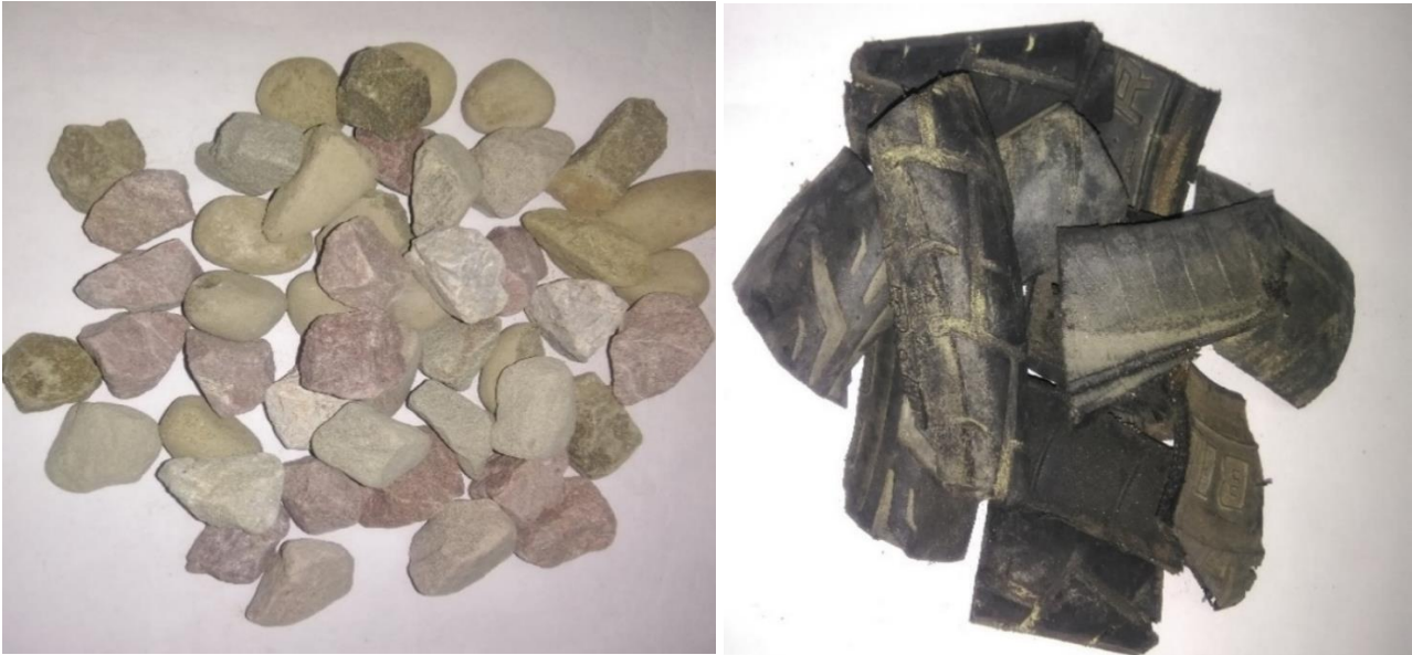
Figure 8.4: Drainage layer material: Gravel (avg. dia 20mm) and Tire derived aggregates (Avg. dimension 20-25mm).
