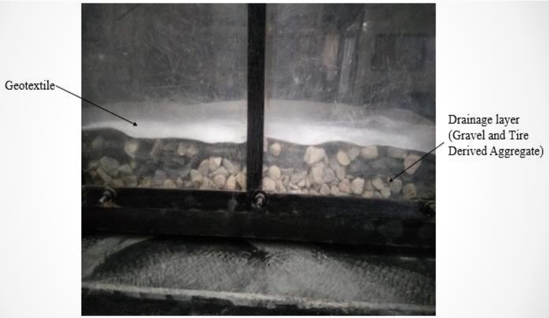
Figure 8.5: Placement of drainage and filter layers in reactor.
