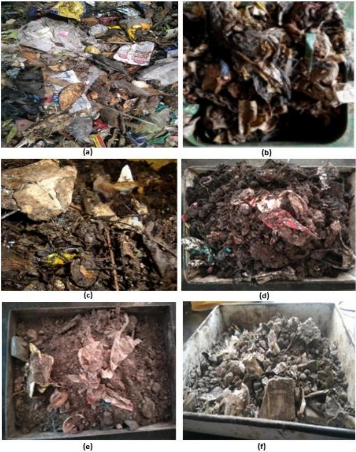
Figure 6.3: Municipal Solid Waste samples a) Fresh Waste b) 0.5-year c) 1-year d) 2 years, e) 4 years and f) 6 years.
