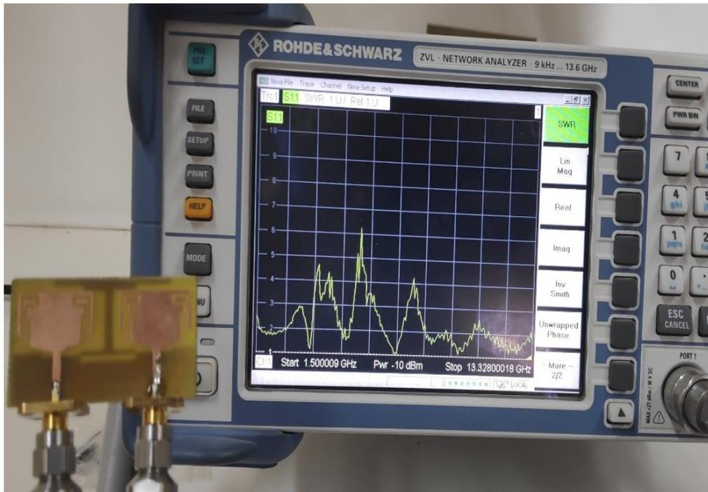
**Figure 3. 11:** Photograph of the VSWR of the proposed antennas measured using a VNA
