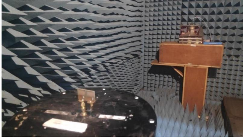
**Figure A.2** Anechoic chamber
