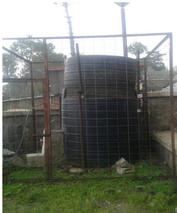
Figure 3.2: Photo view of an outdoor 3,000L Anaerobic continuous reactor at the Jaypee University of Information Technology in Himachal Pradesh
