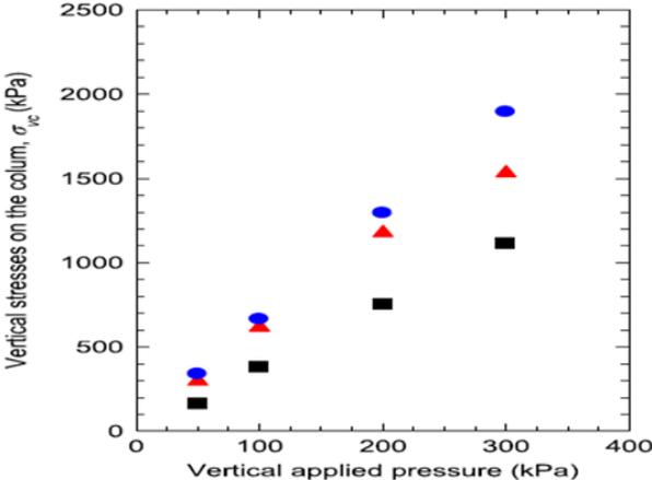
Figure 2.28 (b) Representation of vertical stresses on column under drained conditions [205]
