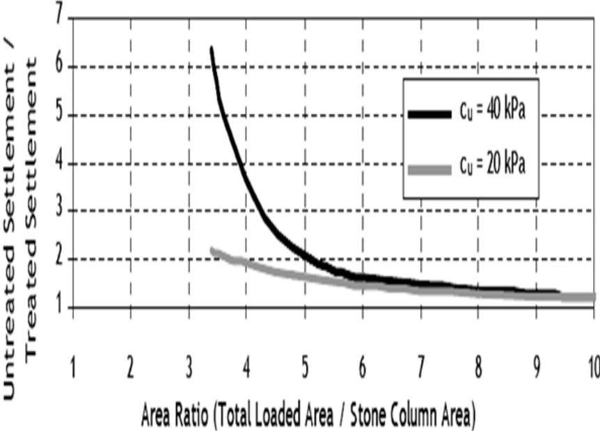
Figure 2.18 Modified Greenwood curves (plot of settlement vs. area ratio) [156]
