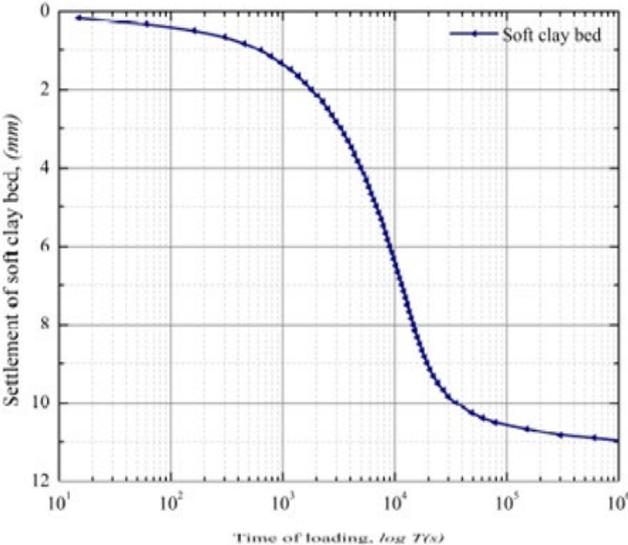
**Figure 2.7 (a)** Settlement vs. Loading Time for Soft Clay Different Bed [104]
