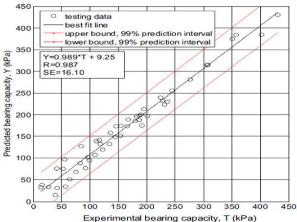
**Figure 2.41 (b)** Graph of experimental bearing capacity against predicted bearing capacity for experimental set: SVR-RBF model [253]
