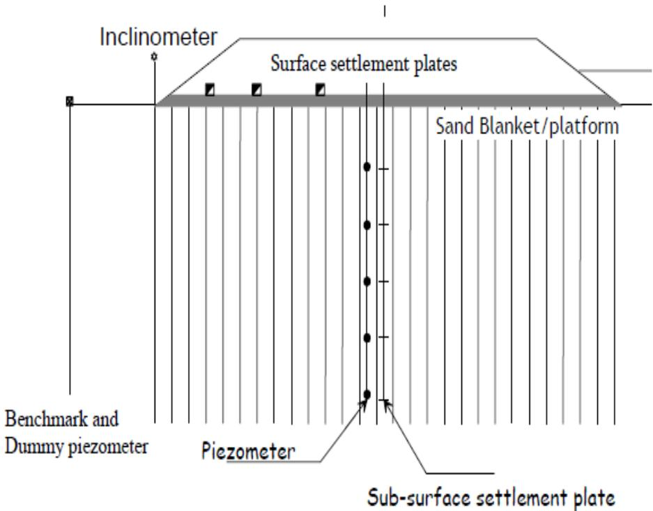
**Figure 1.1** Vertical Drain system with preloading [23]
