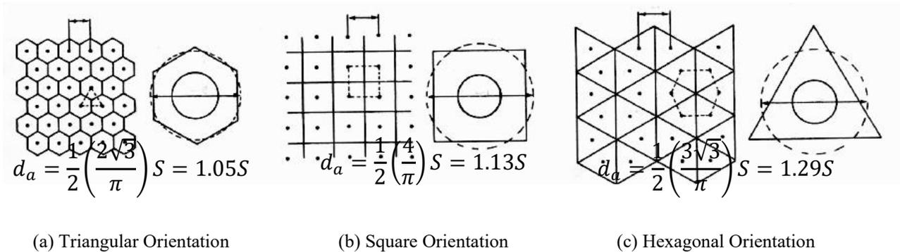
**Figure 2.1** Pattern for the Installation of Stone Columns [68]
