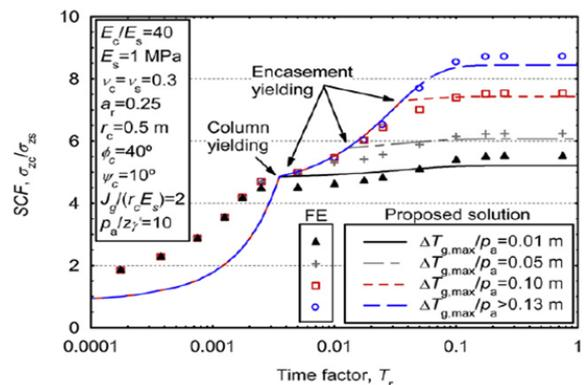
Figure 2.39 (c) Time Plastic columns Influence of the tensile strength of the encasement with Stress concentration factor [227].
