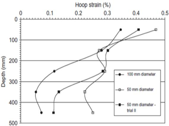
Figure 2.37 (a) Variation in geosynthetic encasement hoop strain (nonwoven geotextile)[182]
