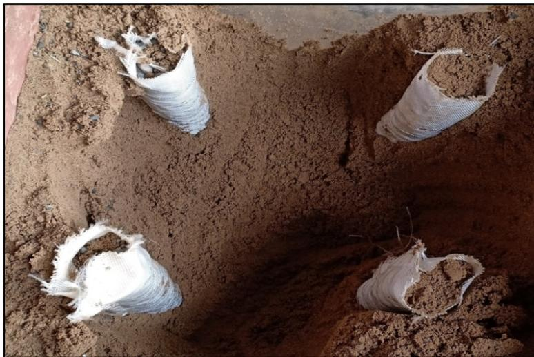
**Figure 4.12 (c)** 4 stone columns with bulging necks were excavated.
