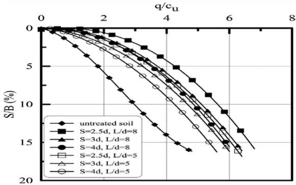
**Figure 2.25 (a)** For a 200.0 mm high embankment model residing on soft soil reinforced to ESCs [201] bearing ratio Vs settlement ratio plot
