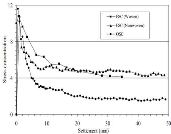
**Figure 2.22 (c)** Effect of stress concentration columns made up of stones with settlement (load test on set of columns-75.0 mm diameter) [184]
