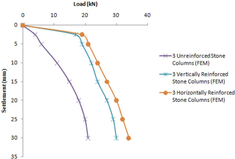
Figure 5.2 Variation in load settlement for three stone columns
