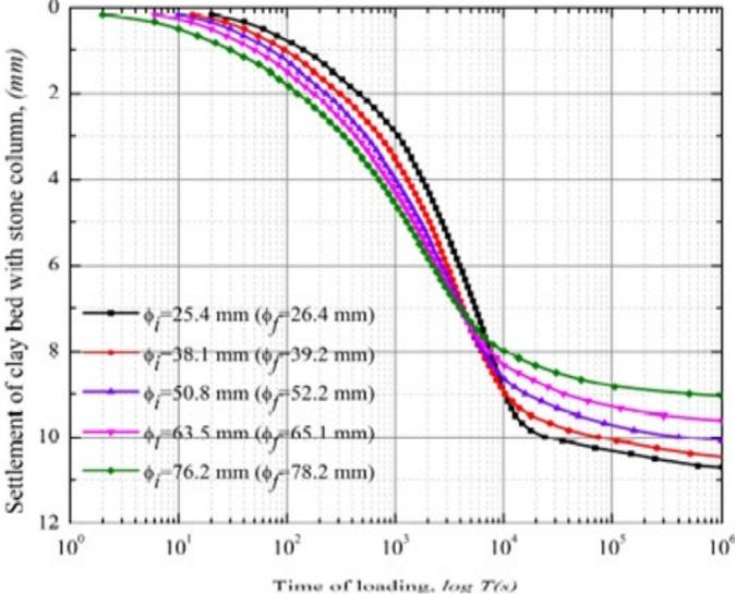
**Figure 2.7 (b)** Settlement vs. Loading Time for 5 dia. of Stone Columns (RP-MC Method) [104]
