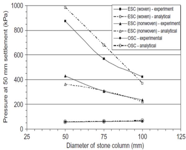
**Figure 2.21 (a)** changes described in pressure correlated to 50.0 mm settlement along with diameter of stone column [182]
