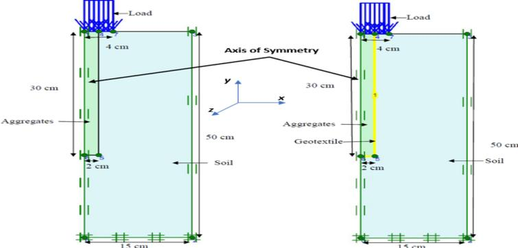
**Figure 3.19** Axisymmetric model of unreinforced and vertically reinforced stone columns
