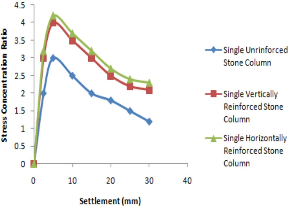
Figure 4.8 Variation of Stress concentration ratio versus settlement for Single stone columns
