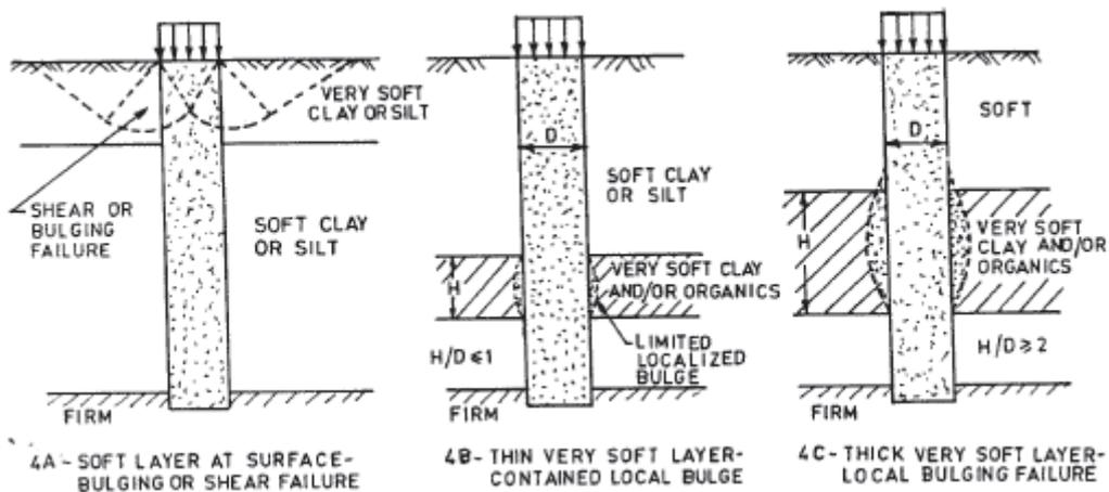
Figure 1.6 Different modes of column failures in non-homogeneous cohesive soil [37]
