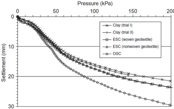
Figure 2.37 (c) Response of experiments with full area-unit cell loading resulting in pressure settlement cell [182]
