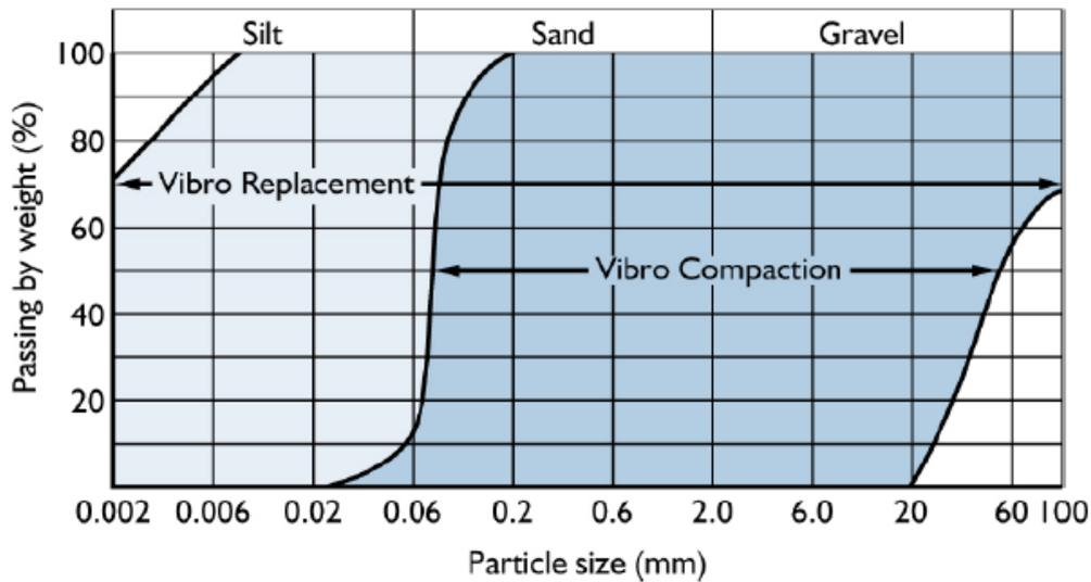
**Figure 1.7** Installation methods for different types of soil types
