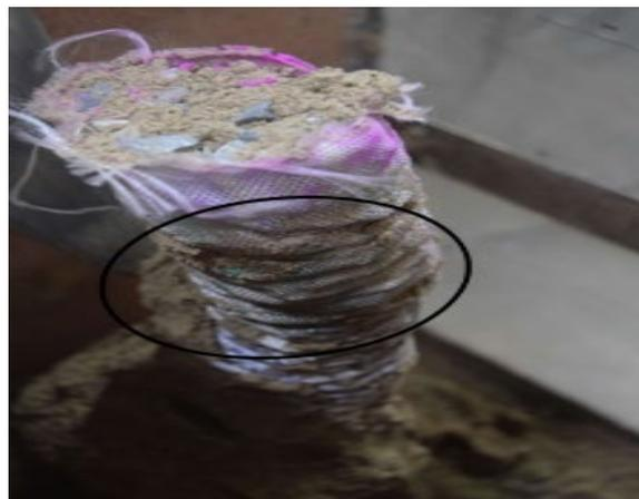
**Figure 4.12 (a)** Excavated Single stone column with bulging at the neck
