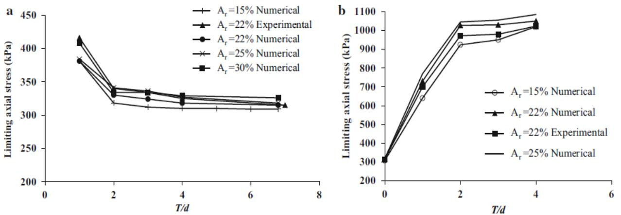
**Figure 2.11** Limiting axial-stress of stone columns vs Top clay thickness of single stone column loading (a)  $L_1$  where  $L_1$ = Soft clay overlapping over rigid clay layering arrangement (b)  $L_2$  where  $L_2$ =Layering system rigid clay overlying loose clay [112]
