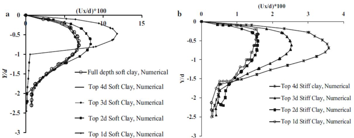
**Figure 2.11** Lateral displacement along the length of stone column for stone column area loading (c)  $L_1$  (d)  $L_2$  [112]
