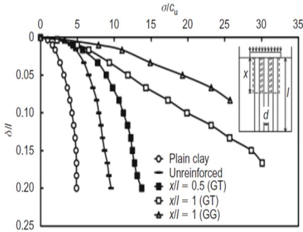
**Figure 2.23 (c)** Consequences of encasement in case of synthesized ground upgraded with set of end-bearing columns ( $d=30.0$  mm,  $l=300.0$  mm,  $Dr = 50.0$  Percent,  $Ar = 25.0$  Percent) [10]
