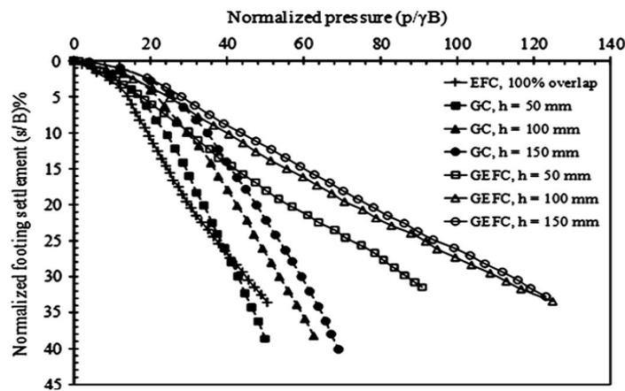
**Figure 2.30 (c)** Footing showing Pressure-settlement responds throughout various composite systems (GC, EFC, and GEFC) in soft clay [207]
