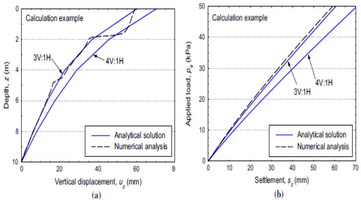
**Figure 2.14** Various load grouping: (a) vertical displacement along with depth; (b) load–settlement curve [125]
