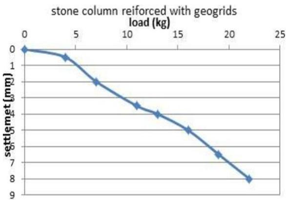
**Figure 2.33 (a)** Soil with stone column reinforced with Geogrids showing load settlement curve [212]
