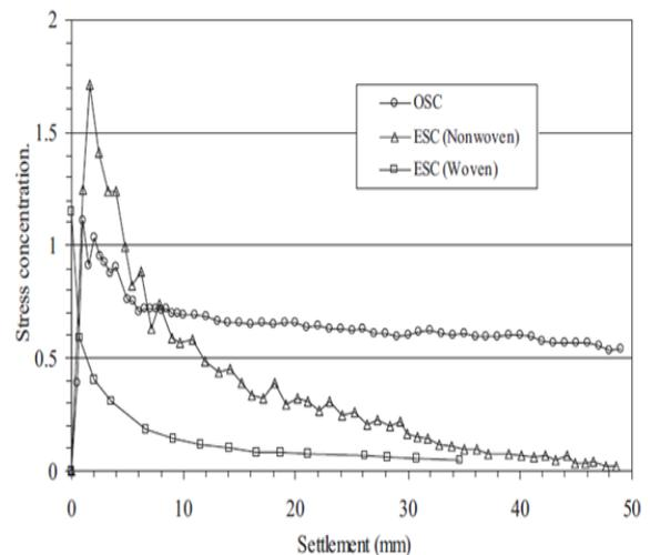
**Figure 2.22 (d)** Concentration of stress on clay surface with settlement [184]
