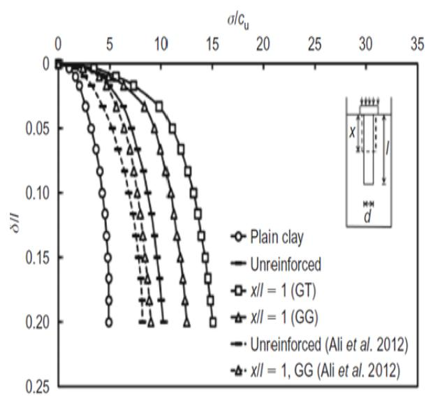
**Figure 2.23 (a)** The effect of geosynthetic form with encasement length over composite ground failure stress was enhanced with even a set of encased floating columns of stones ( $d=30.0$  mm,  $l = 300.0$  mm,  $Dr =50.0$  %,  $Ar =25.0$  %). [10]
