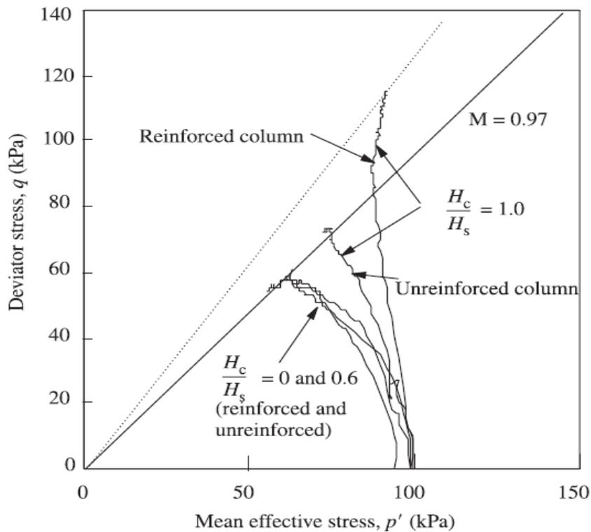
**Figure 2.8 (b)** Stress path: differentiation intermediate to reinforced and unreinforced columns (At consistent loading) [110]
