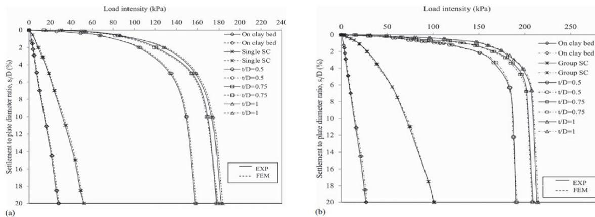
**Figure 2.35** Load settlement graph of (a) Individual Column; and (b) set stone columns for various  $t/D$  ratio [215]
