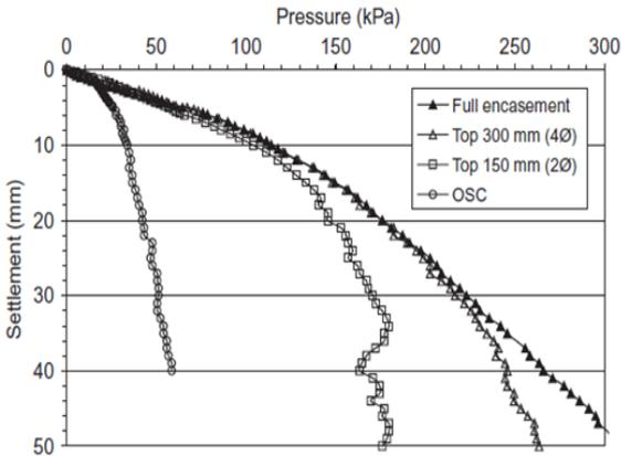
Figure 2.37 (b) Quality of partially encased stone columns (75.0 mm diameter encased for nonwoven geotextile)[182]
