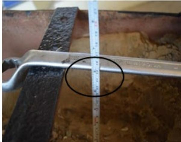
**Figure 4.11 (c)** The distance seen between the end of the column and the model tank's wall.
