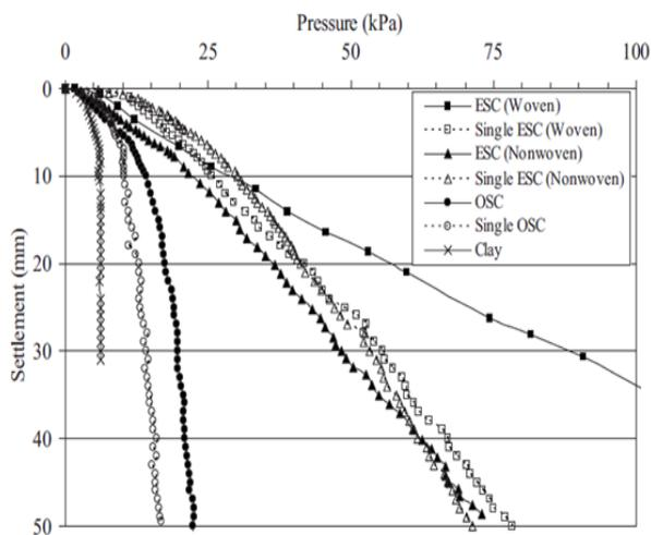
**Figure 2.22 (a)** Comparison between correlated responds from tests on isolated columns pressure-settlement respond to set of stone columns [184]
