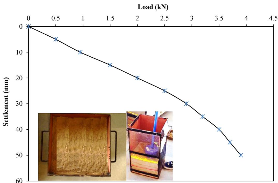
**Figure 4.1** Variation in load – settlement for Sand Bed
