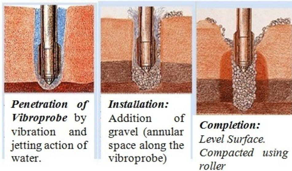
**Figure 1.2** Installation of stone column by vibro – replacement method [30]
