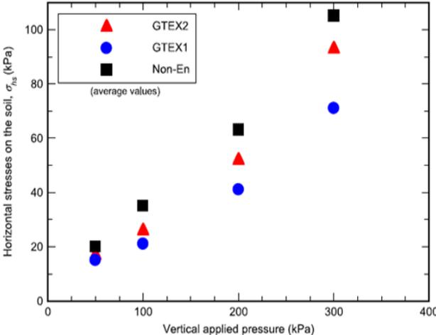
Figure 2.28 (c) Soil having horizontal stresses under drained conditions [205]
