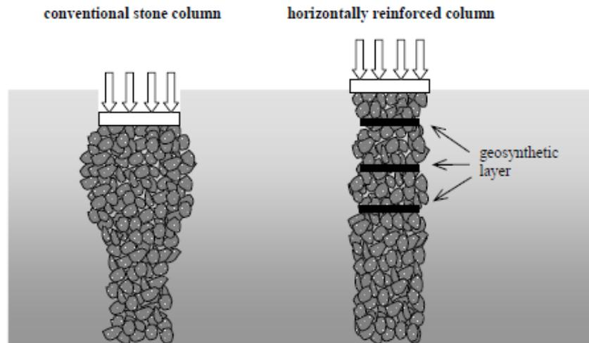
**Figure 1.11** Geosynthetic layering of ordinary stone columns
