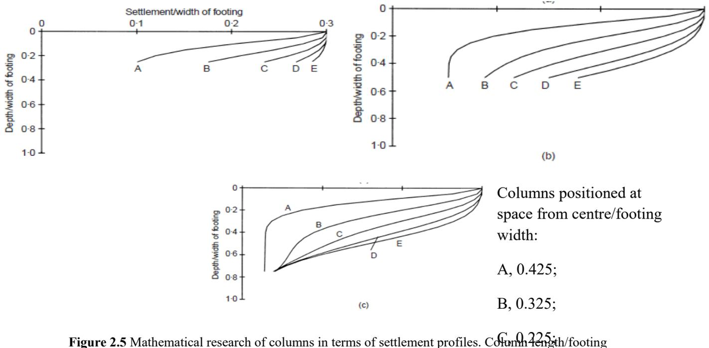
**Figure 2.5** Mathematical research of columns in terms of settlement profiles. Column length/footing width: (a) 0.250; (b) 0.500; (c) 0.750.
