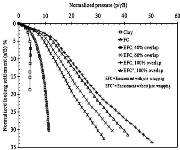
**Figure 2.30 (a)** Footing depicting pressure-settlement responses across fly-ash columns of full-length encasements formulated along differing lap over percentages (.40.0, 60.0, & 100.0 %) throughout plastic bottle cells. [207]
