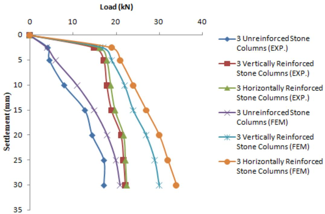
Figure 5.9 Variation in load settlement for three stone columns
