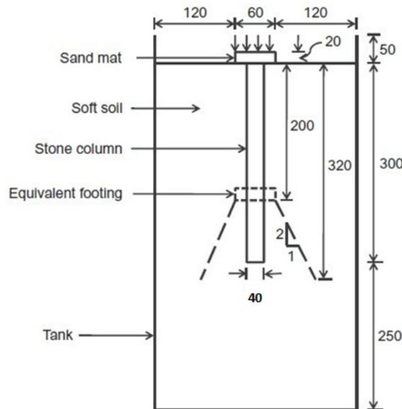
Figure 3.9 Schematic views of modeled Single stone columns
