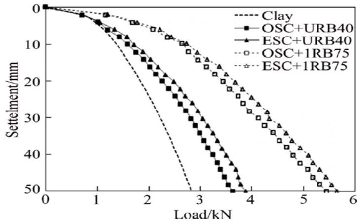
**Figure 2.32** Variation of load settlement in combined form of granular blankets and stone columns [211]
