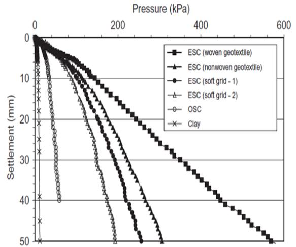
**Figure 2.21 (b)** Pressure–settlement curves for 75.0 mm diameter columns encased in various kinds of geosynthetics [182]
