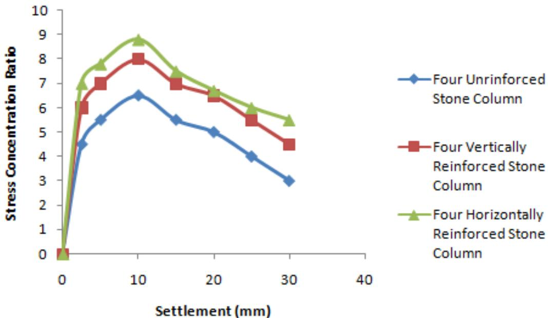
Figure 4.10 Variation of Stress concentration ratio versus settlement for 4 stone columns
