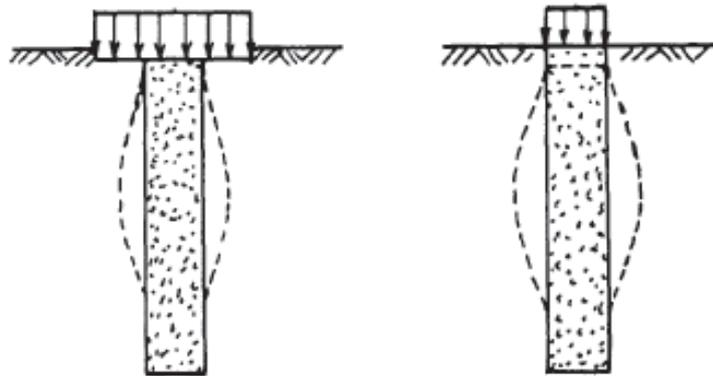
Figure 1.5 Load applied to the stone columns [37]
