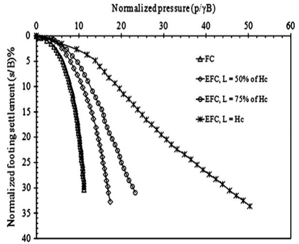
**Figure 2.30 (b)** Footing showing pressure-settlement responds in column of encased fly-ash columns having different lengths (100.0 % lap over) [207]
