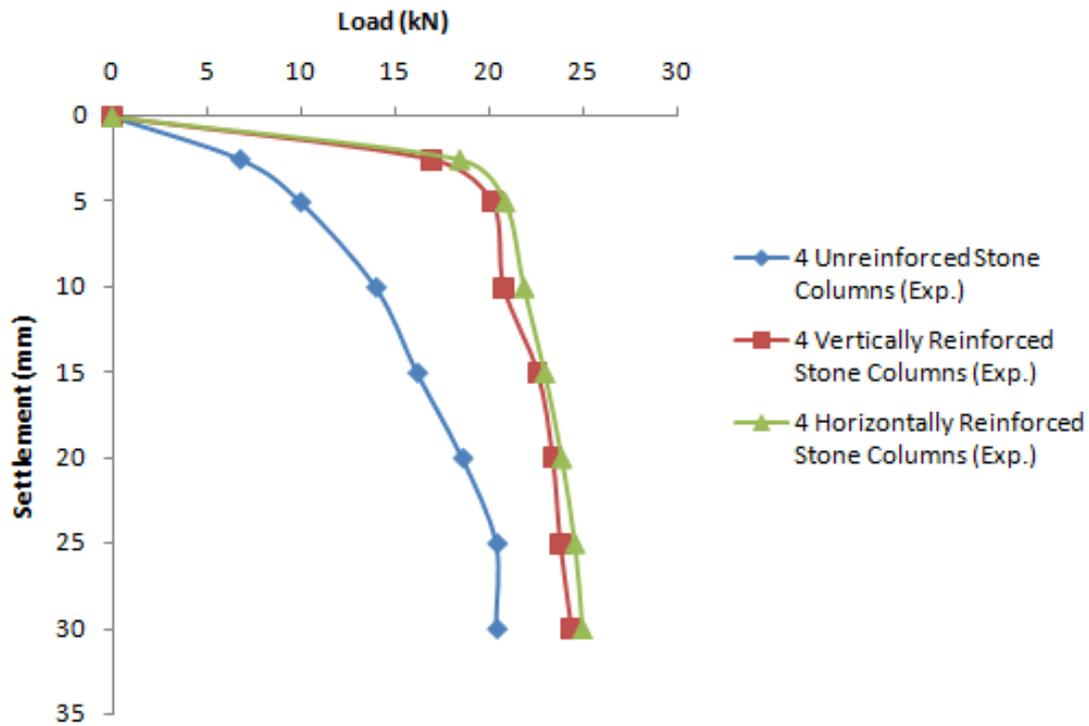
**Figure 4.4** Variation in load – settlement for a group of four stone columns
