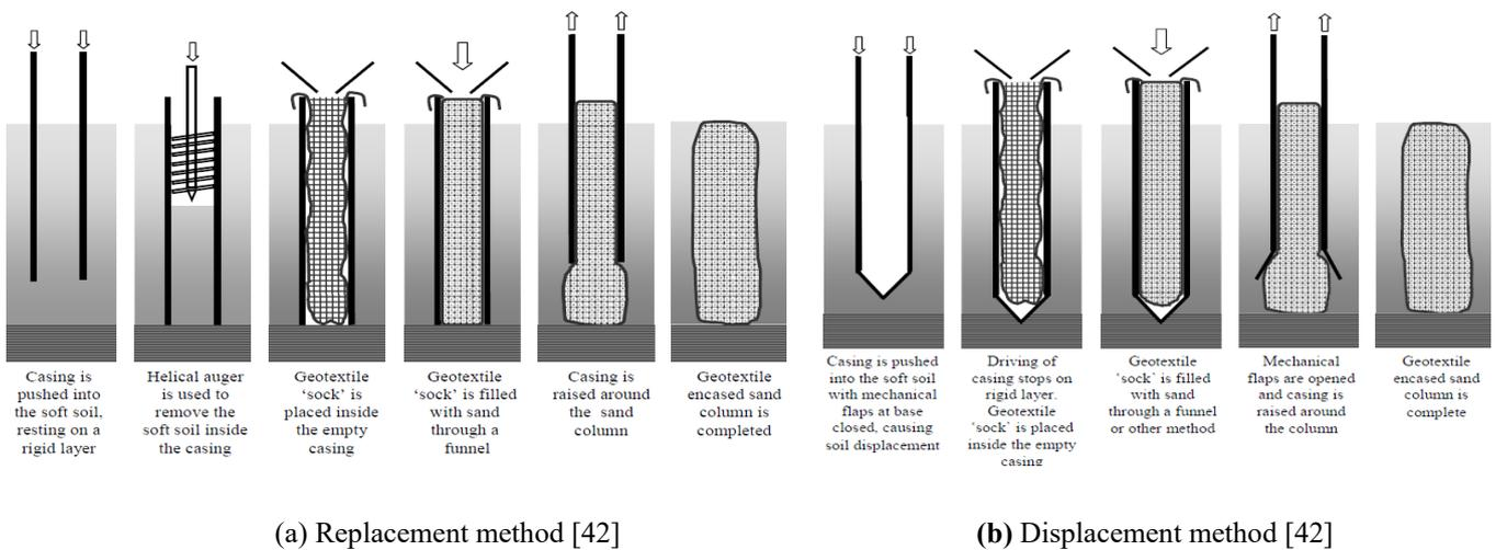
Figure. 1.10 Construction of GECs
