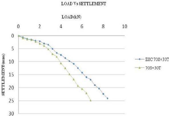
Figure 2.29 (b) Comparison of floating columns with and without encasement [206]
