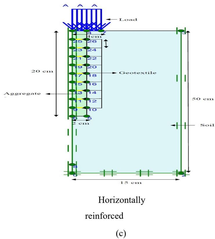
Figure 3.22 Geometry Model with all structural elements
