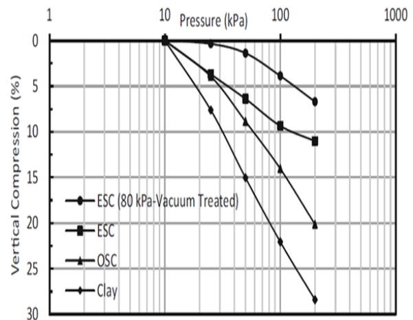
**Figure 2.31 (b)** Pressure Response – Vertical Compression comparison chart for various systems [210]
