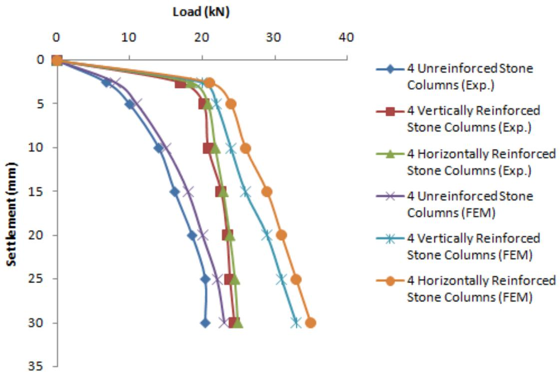
Figure 5.10 Variation in load settlement for four stone columns
