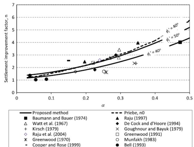
Figure 2.16(b) Comparison of End-bearing results [148]
