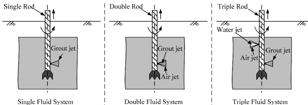
**Figure 1.3** Jet grouting [35]
