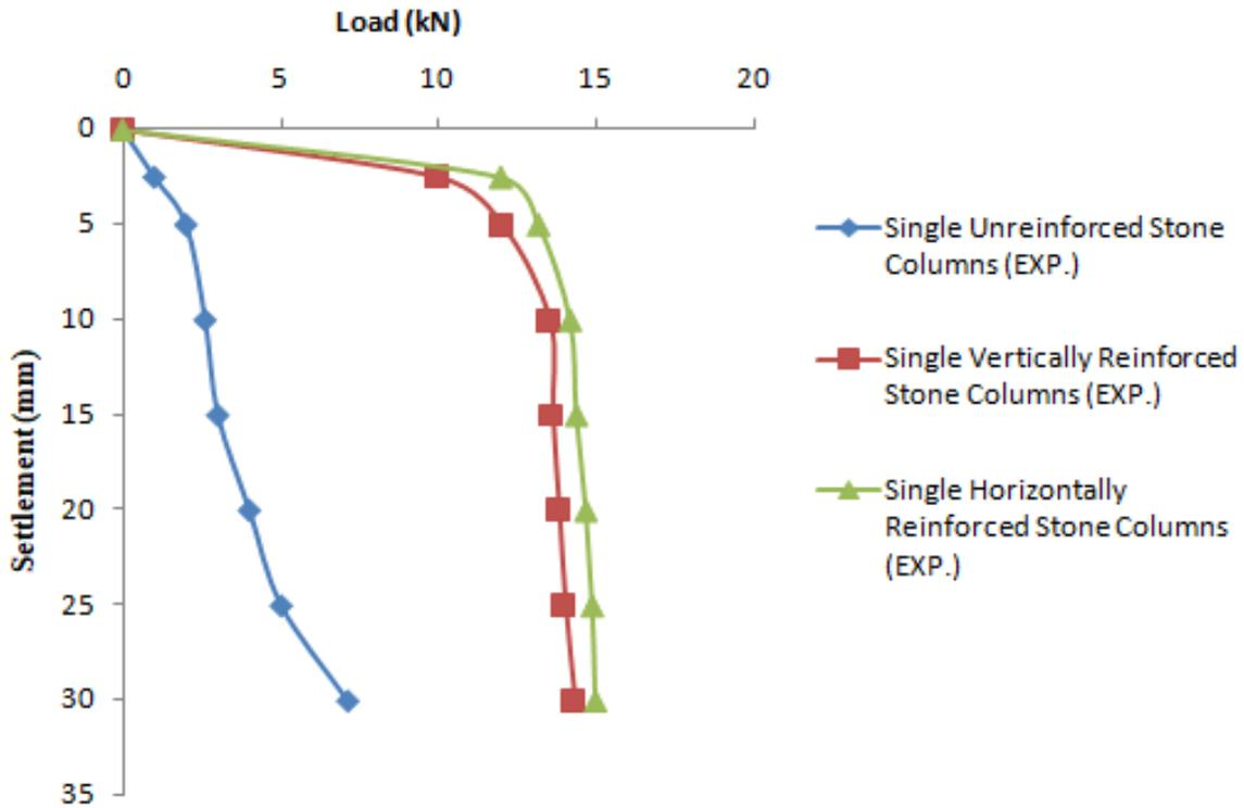
Figure 4.2 Load – settlement variation for single stone column
