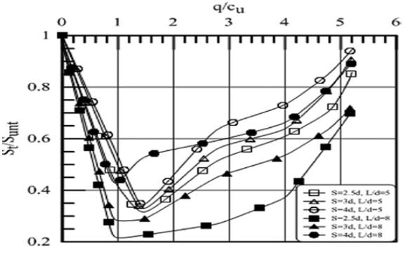
**Figure 2.25 (b)** Bearing ratio for a 200.0 mm large embankment lying on loose soil reinforced on ESCs versus Settlement improvement ratio [201] representation
