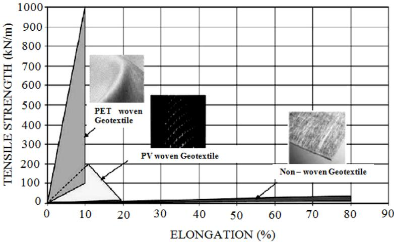
**Figure 1.9** Tensile strength vs. elongation curve for woven and nonwoven geotextiles [39]
