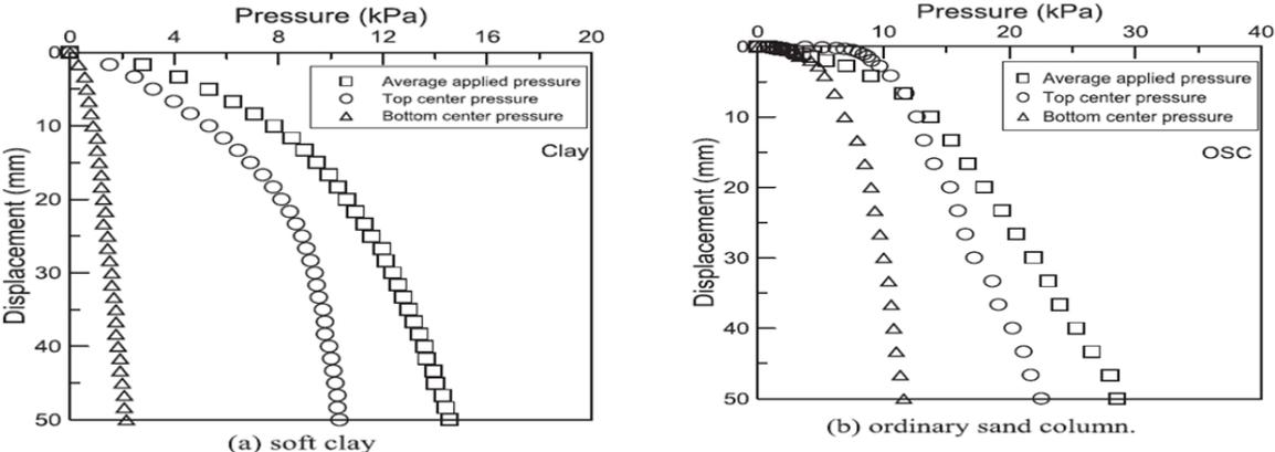
**Figure 2.26** Representation of vertical pressure-displacement association with ordinary sand column as well as soft: **(a)** soft clay; **(b)** ordinary sand column [202]
