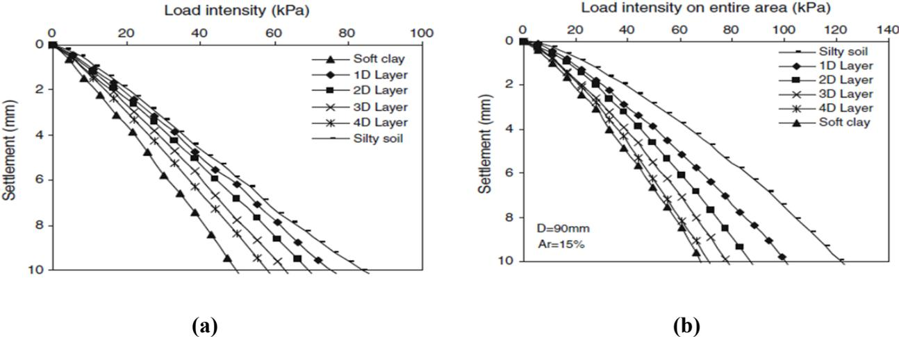
**Figure 2.6 (a)** Load-settlement action of untreated layered soils and **(b)** The thickness of the upper weak layer has an influence on the load settlement action of composite land. [101].
