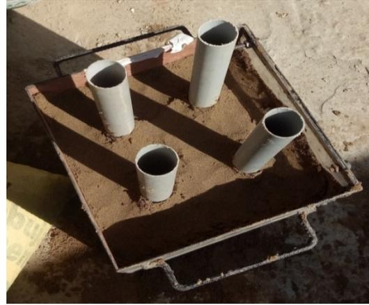
**Figure 3.14 (b)** Un-reinforced group of 4 columns
