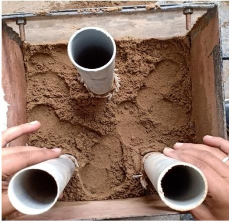
**Figure 3.14 (a)** Un-reinforced group of 3 columns
