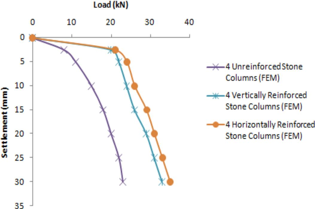
Figure 5.3 Variation in load settlement for group of four columns
