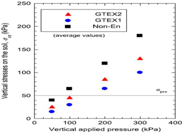
Figure 2.28 (a) Representation of vertical stresses on soil under drained conditions [205]
