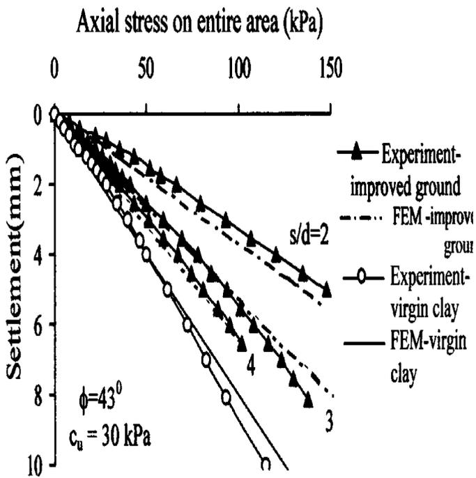
Figure 2.2 (c)  $s/d$  effect on stress /settlement behavior entire area loaded [87]
