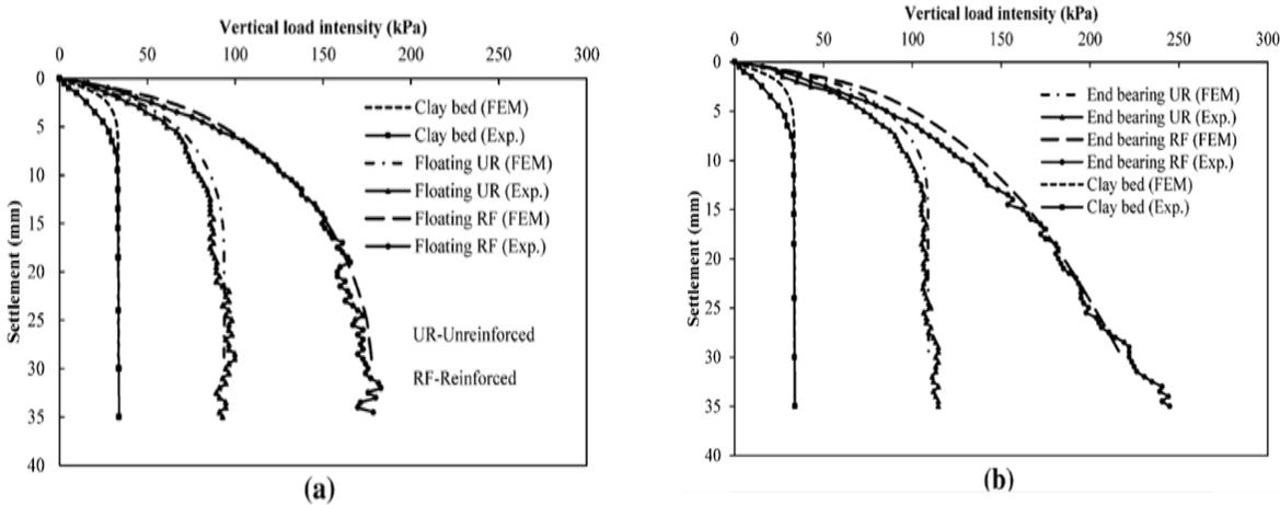
Figure 2.34 Granular piles' vertical load intensity settlement reactions; (a) Floating, (b) End bearing [200]
