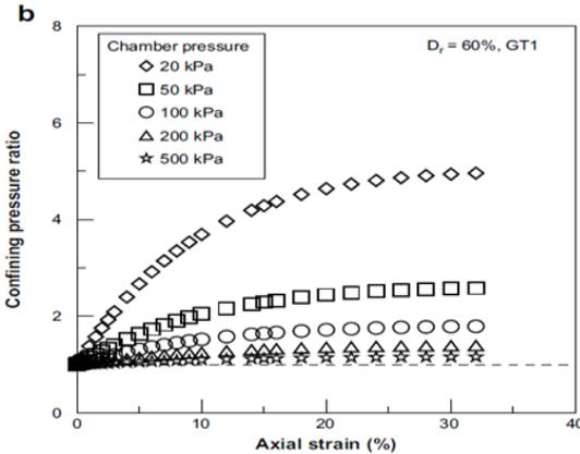
Figure 2.40(c) Inspired confining pressure for reinforced samples with variable chamber pressures ( $D_r = 60.0\%$ , GT1 geotextile). (a) Inspired confining pressure, (b) confining pressure ratio [245]
