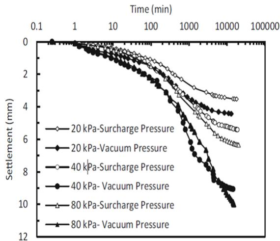
**Figure 2.31 (a)** Vacuum and surcharge differentiation preloading time-settlement graph [210]
