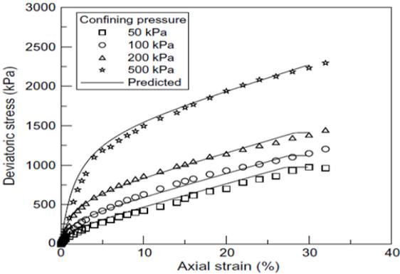
Figure 2.40 (b) Reinforced sand specimens experimental and analytical results [244]
