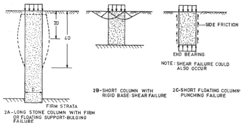
**Figure 1.4** Modes of failure for stone columns in homogeneous soils [37]
