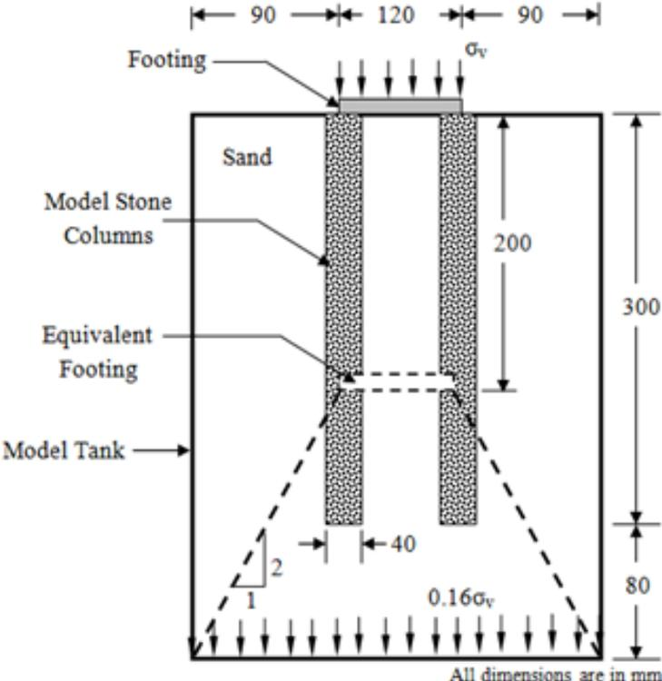
Figure 3.10 Schematic view of modeled group stone columns (3 & 4).
