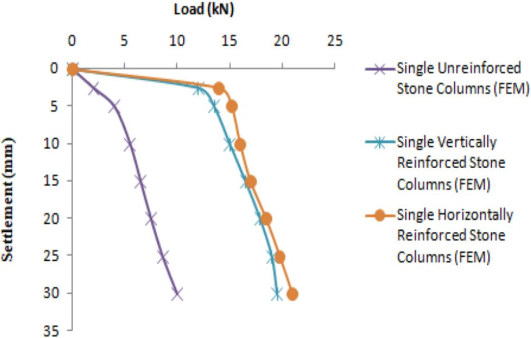
**Figure 5.1** Load – settlement variation for Single stone column
