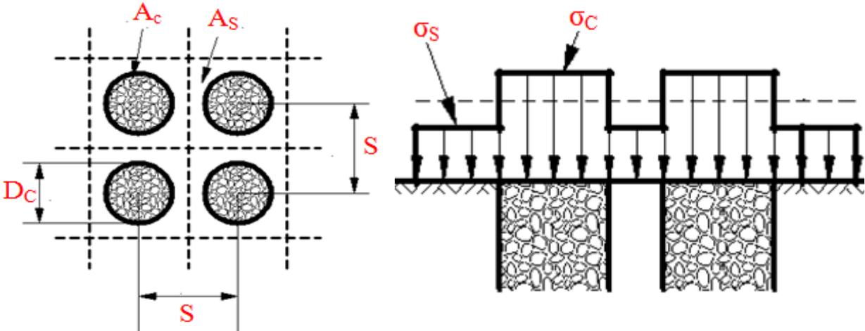
**Figure 2.4** Diagram of composite ground [89]
