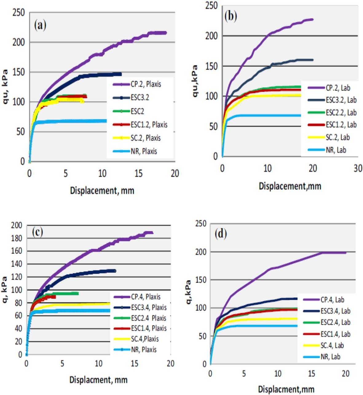
**Figure 2.12** Rigidity effects on displacement due to load variation of multiple positioning of column a, b  $s/D=2.0$  also for c, d  $s/D=4.0$  [113]
