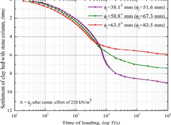
**Figure 2.7 (d)** Settlement vs. Loading Time for 38.1, 50.8, 63.5 mm dia. of Stone Columns (DP-HC Method) [104]
