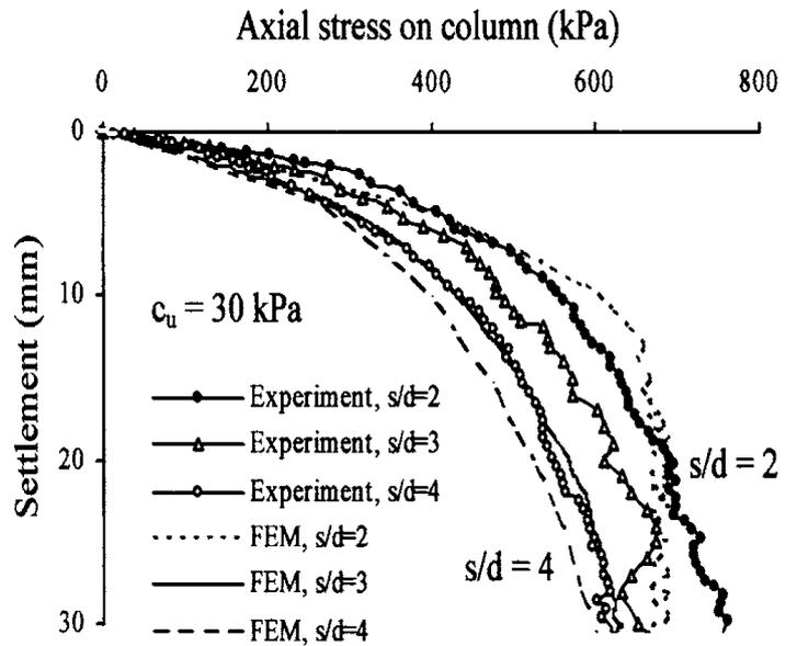
Figure 2.2 (b) Effect of  $s/d$  on behavior of stone column [87]
