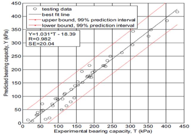
**Figure 2.41 (d)** Graph of experimental bearing capacity against predicted bearing capacity for observation set: SVR-POLY model [253]
