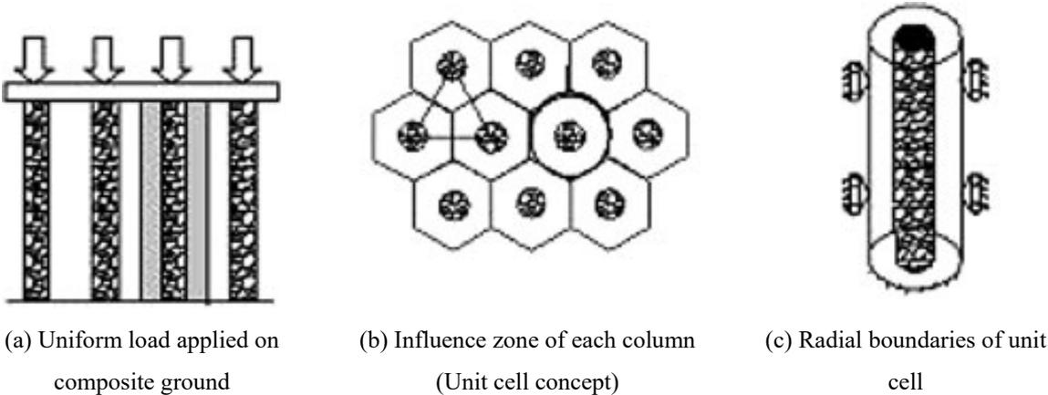
**Figure 2.3** Concept of unit cell
