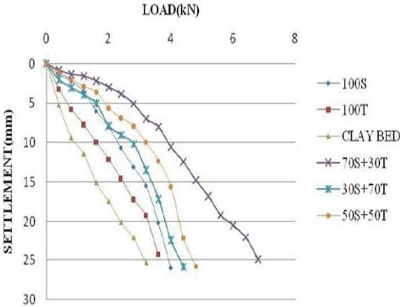
Figure 2.29 (a) Test results for floating columns [206]
