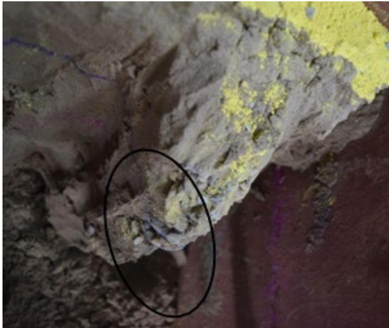
**Figure 4.13 (b)** Side view of the column after exhumation depicting bulging at neck
