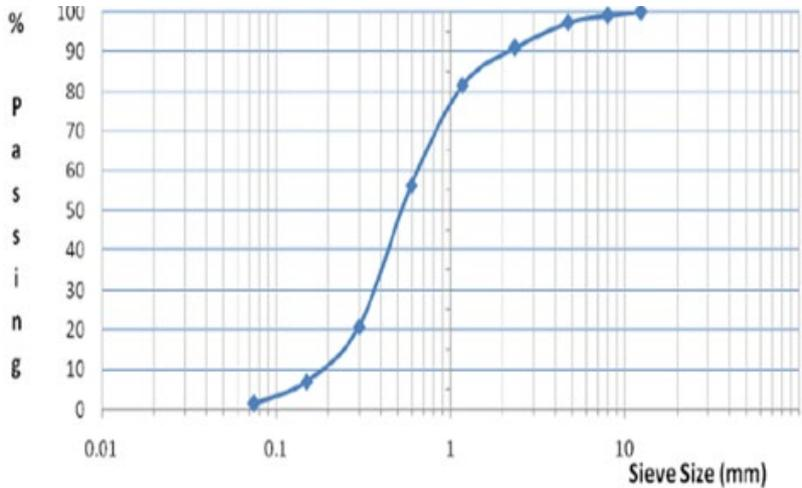
**Figure 3.4** Distribution curve for the particle size of the aggregates
