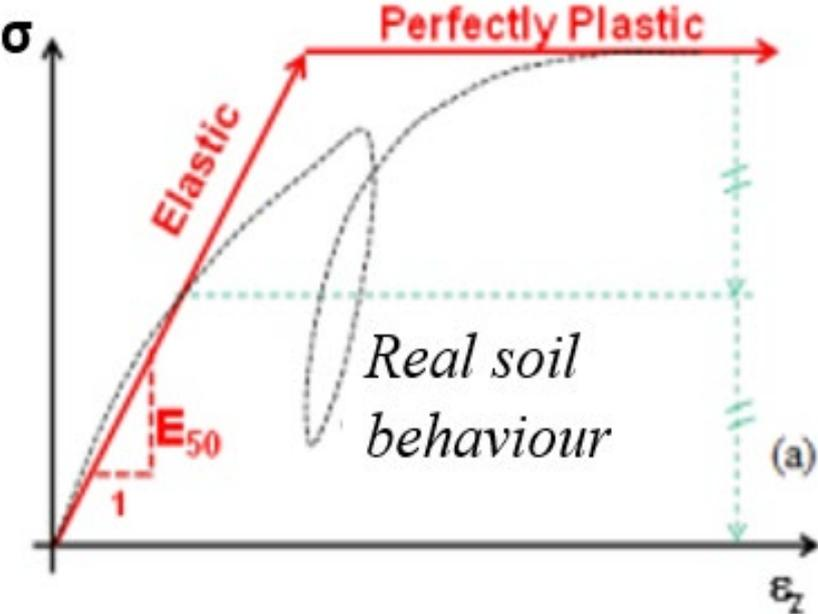
**Figure. 3.20** Simplification of real soil behavior by Mohr – Coulomb model
