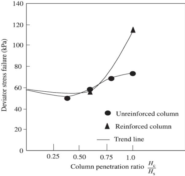
**Figure 2.8 (a)** Deviator stress at collapse: contrast intermediate to reinforced and unreinforced columns (At consistent loading) [110]
