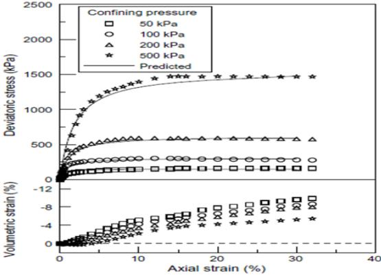
Figure 2.40 (a) un-reinforced sand specimens tri axial test results [244]
