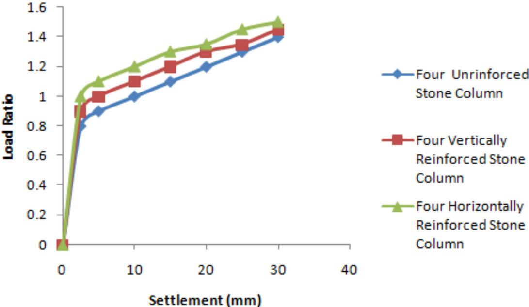
Figure 4.7 Variation of load ratio versus settlement for 4 stone columns
