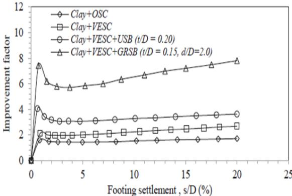
**Figure 2.36 (a)** Change of improvement factor with different combinations of reinforcement [229]
