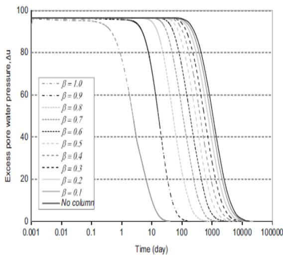
Figure 2.16(a) Excess pore water pressure distribution for  $\beta=0.0$  to -1 [148]
