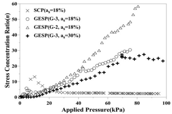
**Figure 2.24 (b)** differentiation of Stress Concentration Ratio from Experimental Findings [198]
