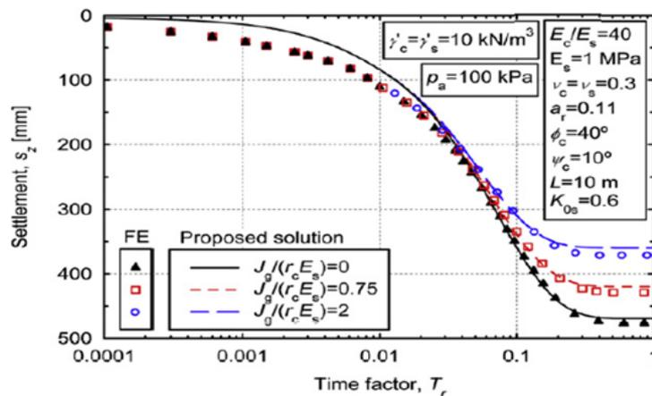
Figure 2.39 (a) for Common encasement stiffness's with time-settlement curves [227]
