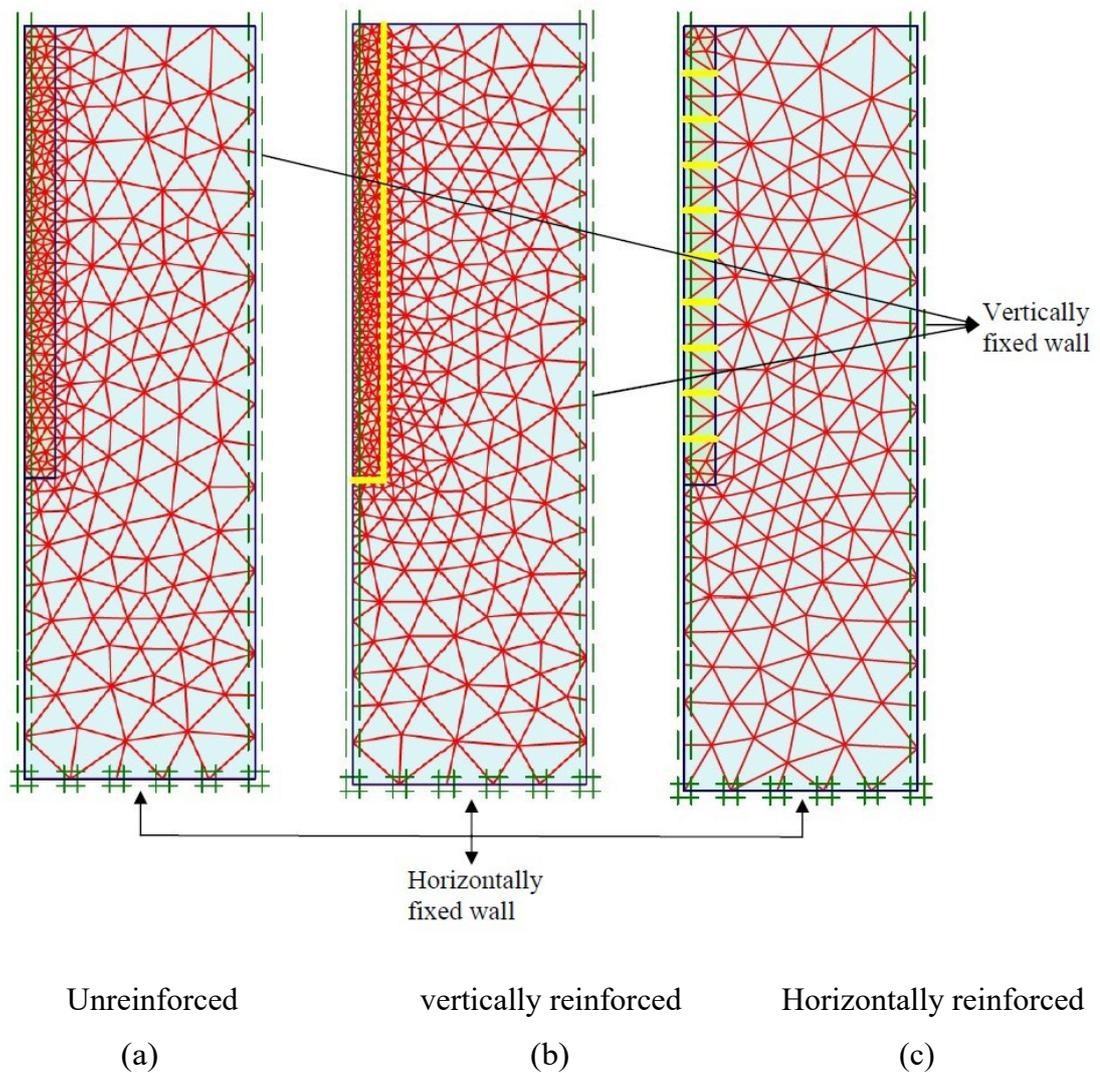
Figure 3.23 Initial Mesh Generated
