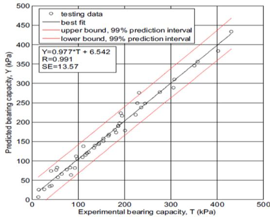
**Figure 2.41 (c)** Graph of experimental bearing capacity against predicted bearing capacity for experimental set: ANFIS model [253]
