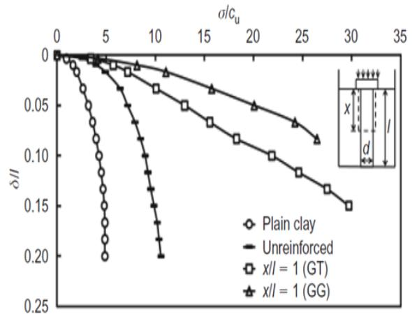
**Figure 2.23 (d)** Consequences of encasement in case of synthesized ground upgraded with only end-bearing columns ( $d=30.0$  mm,  $l=300.0$  mm,  $Dr = 50.0$  %,  $Ar = 25.0\%$ ) [10]
