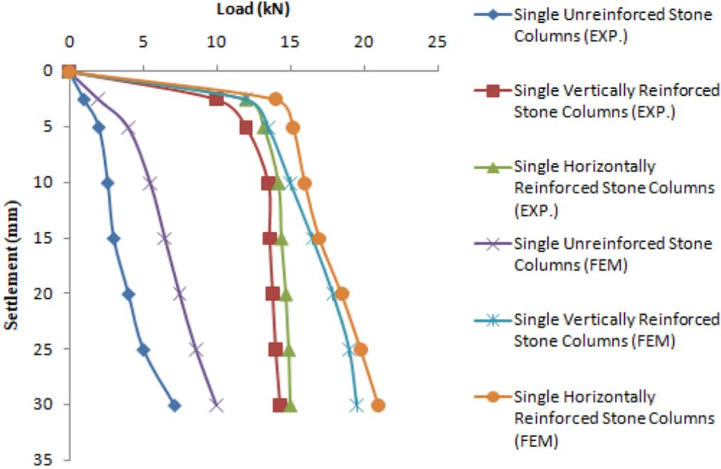
Figure 5.8 Variation in load settlement for single stone columns
