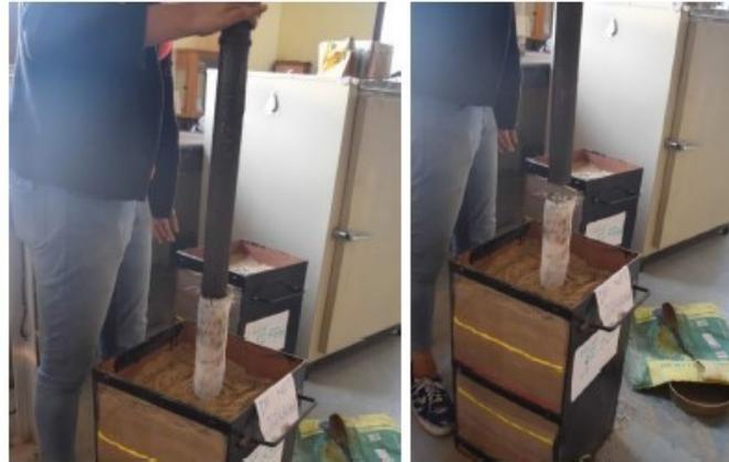
**Figure 3.15** Vertical encasement
