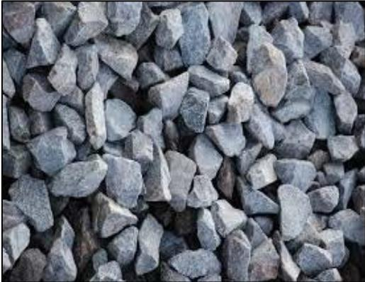
**Figure 3.3** Stone Columns are made out of crushed stones.
