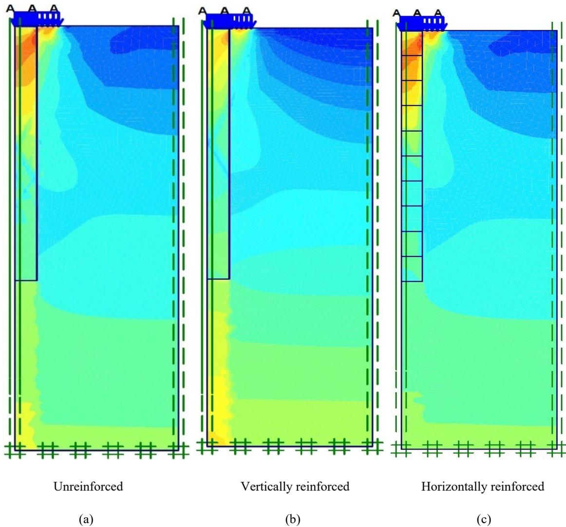
**Figure 5.4** Deformed mesh for Single stone columns
