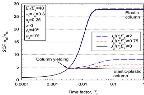
Figure 2.39 (b) Time Influence of the encasement stiffness with stress concentration factor [227]
