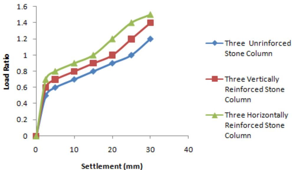
Figure 4.6 Variation of load ratio versus settlement for 3 stone columns
