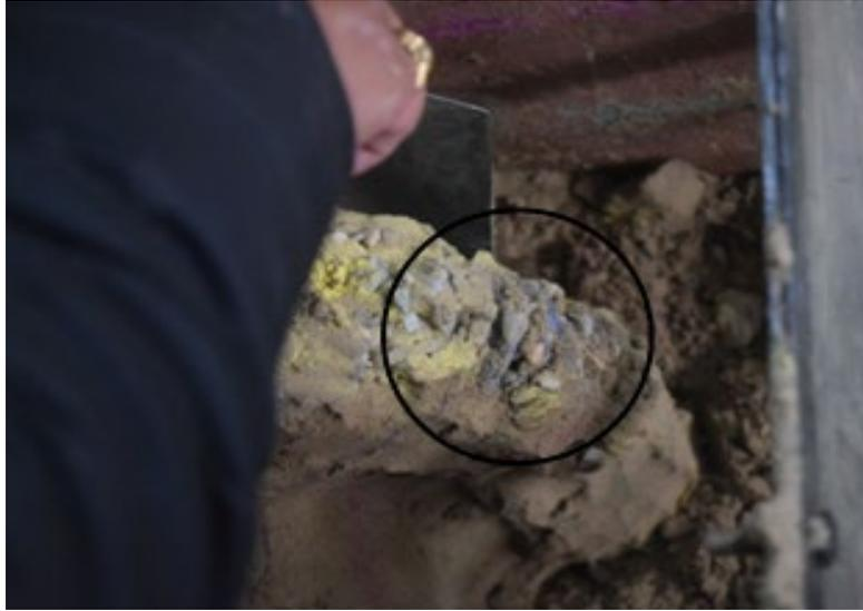
**Figure 4.13 (a)** Top view of the column during exhumation
