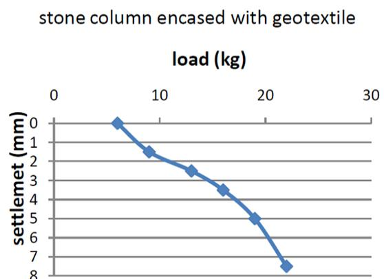
**Figure 2.33 (b)** Representation of load settlement curve of soil bed with stone column encased with geotextile [212]
