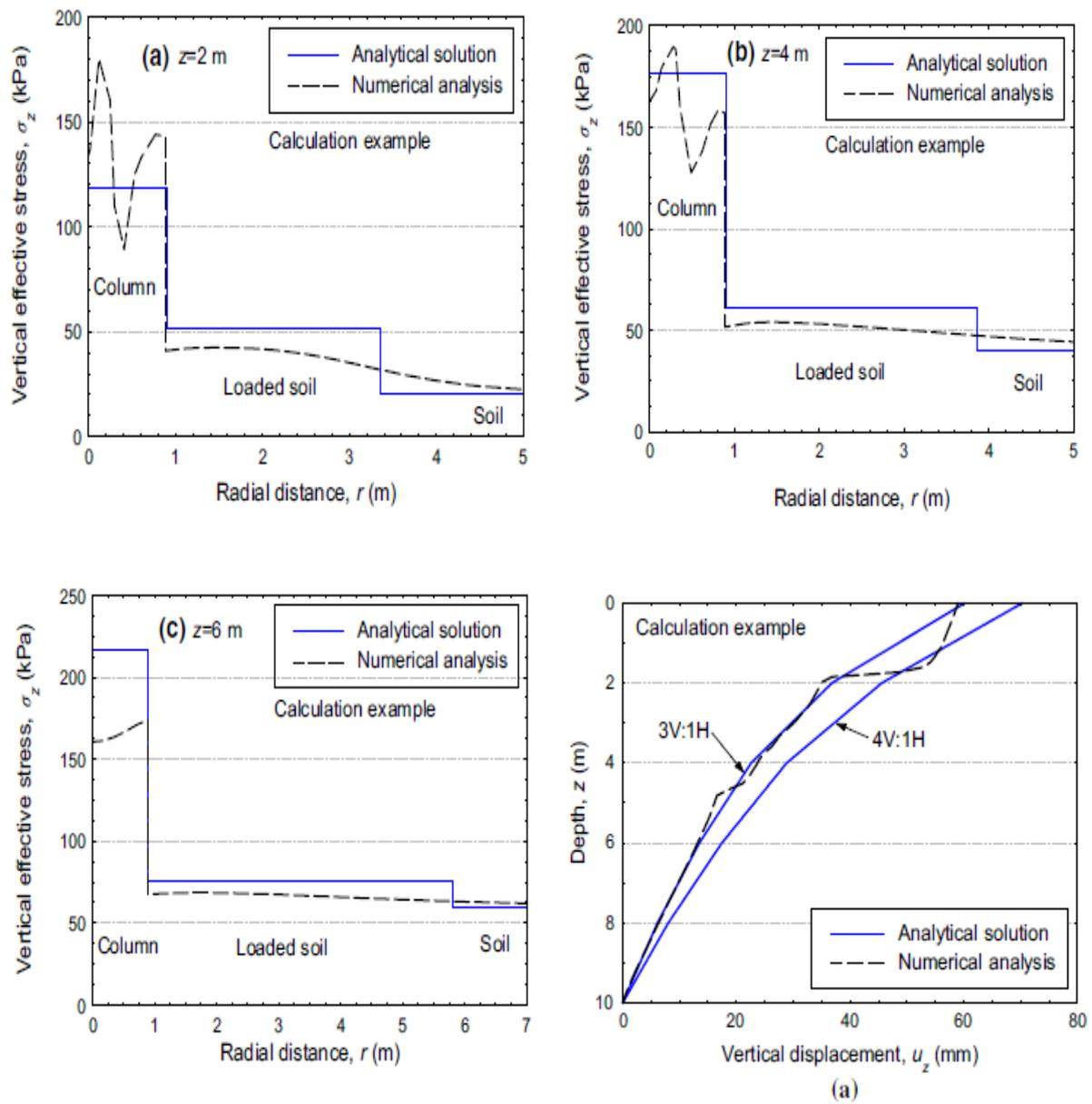
Figure 2.13 Vertical stresses at several depths [125]
