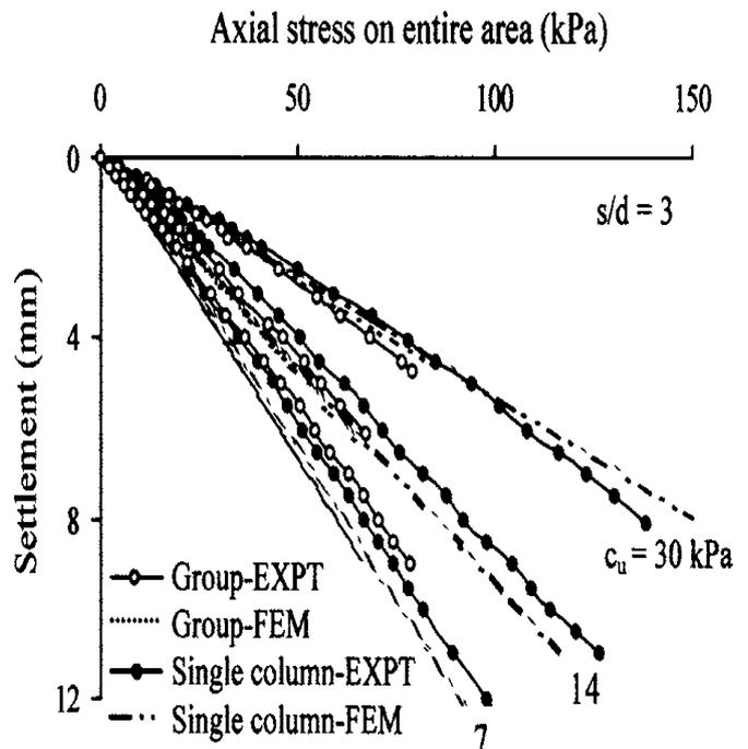
Figure 2.2 (d) Comparison btw group and single column test [87]
