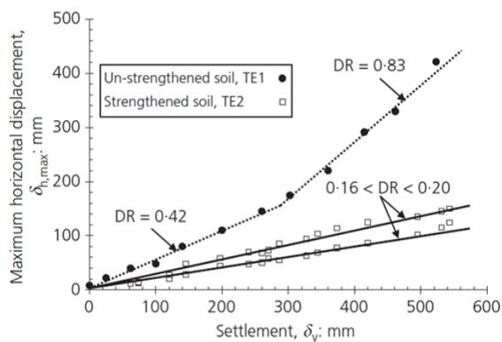
**Figure 2.27 (a)** Graph showing Co-relation between soil horizontal deformation for TE1 and TE2 and settlement [203]
