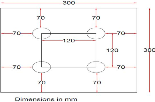
**Figure 3.13 (b)** Square Arrangement of Stone Columns
