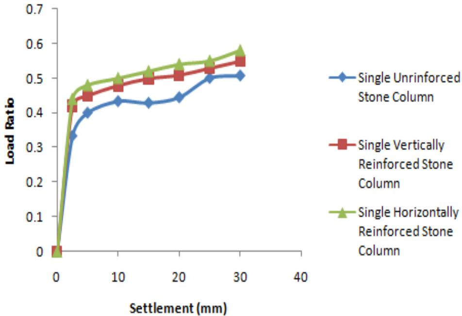
Figure 4.5 Variation of load ratio versus settlement for single stone column
