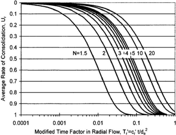
Figure 2.20(b) Consolidation rate in Radial Flow [160].
