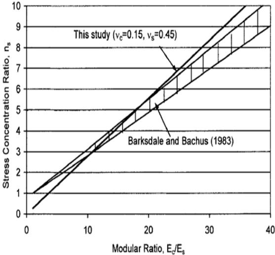
Figure 2.20 (a) Stress Concentration Ratio and Modular Ratio relationship [160]
