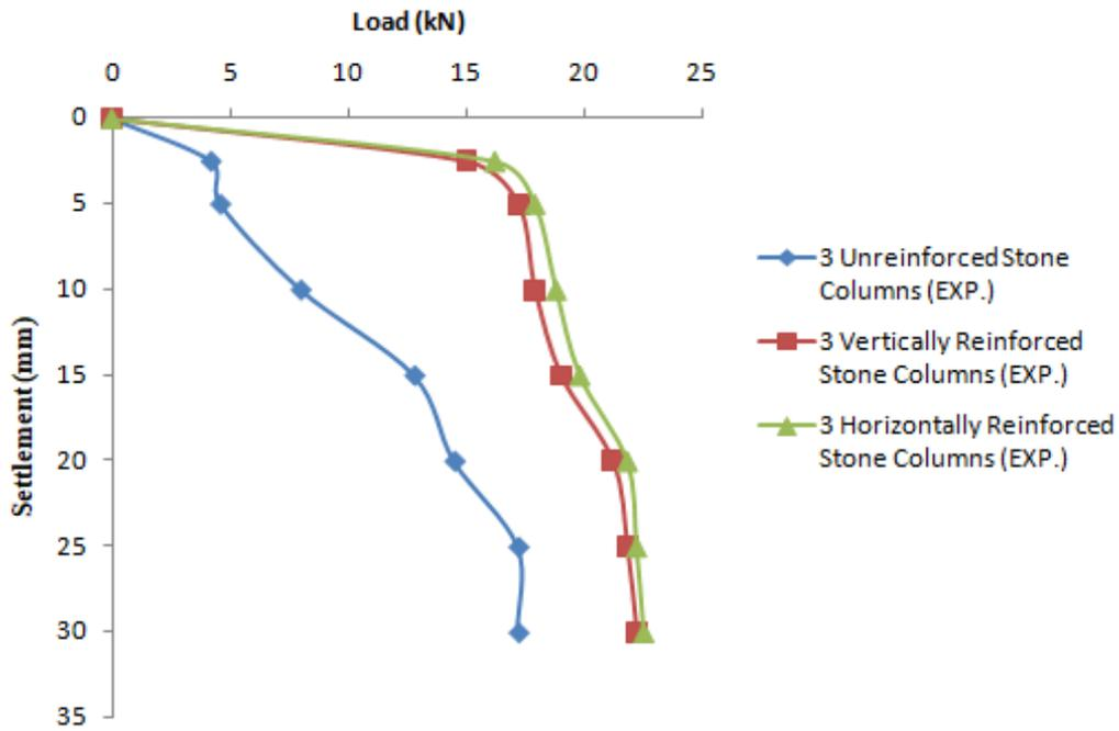
**Figure 4.3** Variation in load settlement for three stone columns in group.
