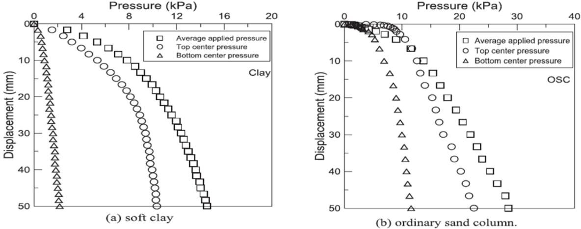
Figure 2.38 (b) Relationship between vertical pressure-displacement for soft clay and the ordinary sand column: (a) soft clay; (b) ordinary sand column [202]
