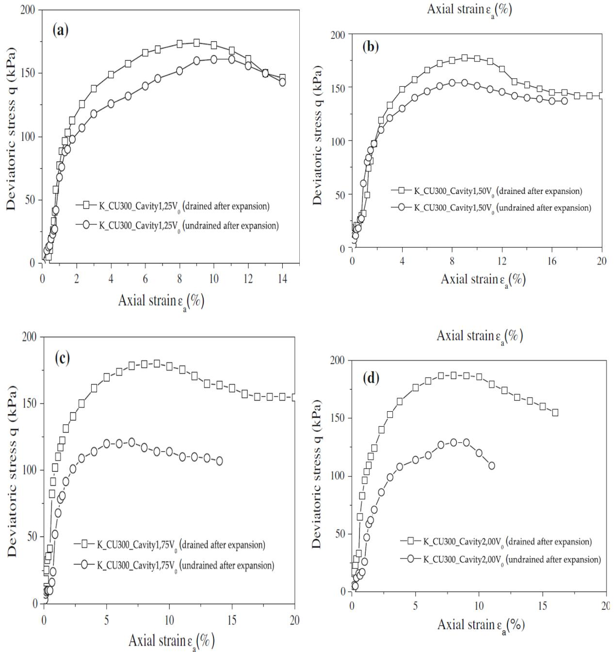
**Figure 2.10** Axial stress–strain relationship (triaxial shear loading = 300.0 kPa) for samples of drained along with undrained ;Distinct cavity expansion proportion  $V/V_0$  post cavity expansion (a) 1.250, (b) 1.50, (c) 1.750 and (d) 2.0 [114]
