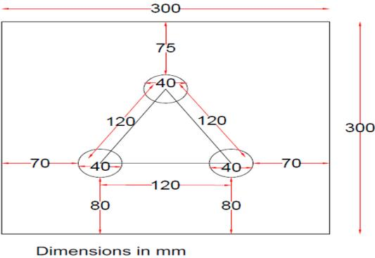
**Figure 3.13 (a)** Triangular Arrangement of Stone Columns
