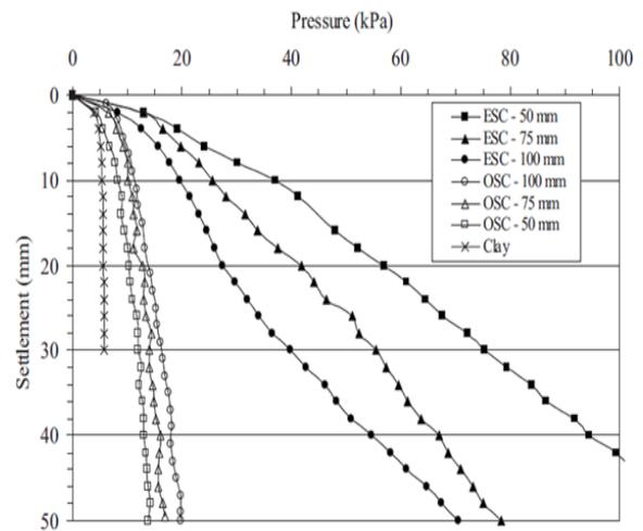
**Figure 2.22 (b)** Pressure-settlement responds of solo OSCs and ESCs (woven) [184]
