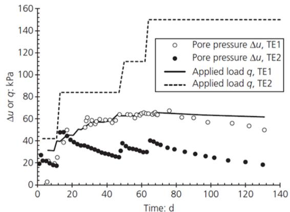
**Figure 2.27 (b)** Discrepancy of extra pore pressure estimated in middle of soft clay with time for TE1 and TE2 [203]
