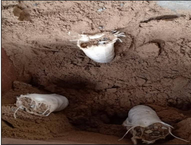
**Figure 4.12 (b)** Excavated 3 stone columns with bulging at neck
