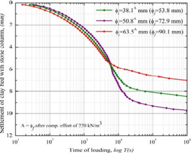
**Figure 2.7 (c)** Settlement vs. Loading Time for 38.1, 50.8, 63.5 mm dia. of Stone Columns (RP-HC Method) [104]
