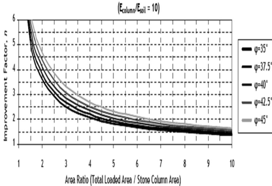
**Figure 2.19** Modified Priebe design curves [157]
