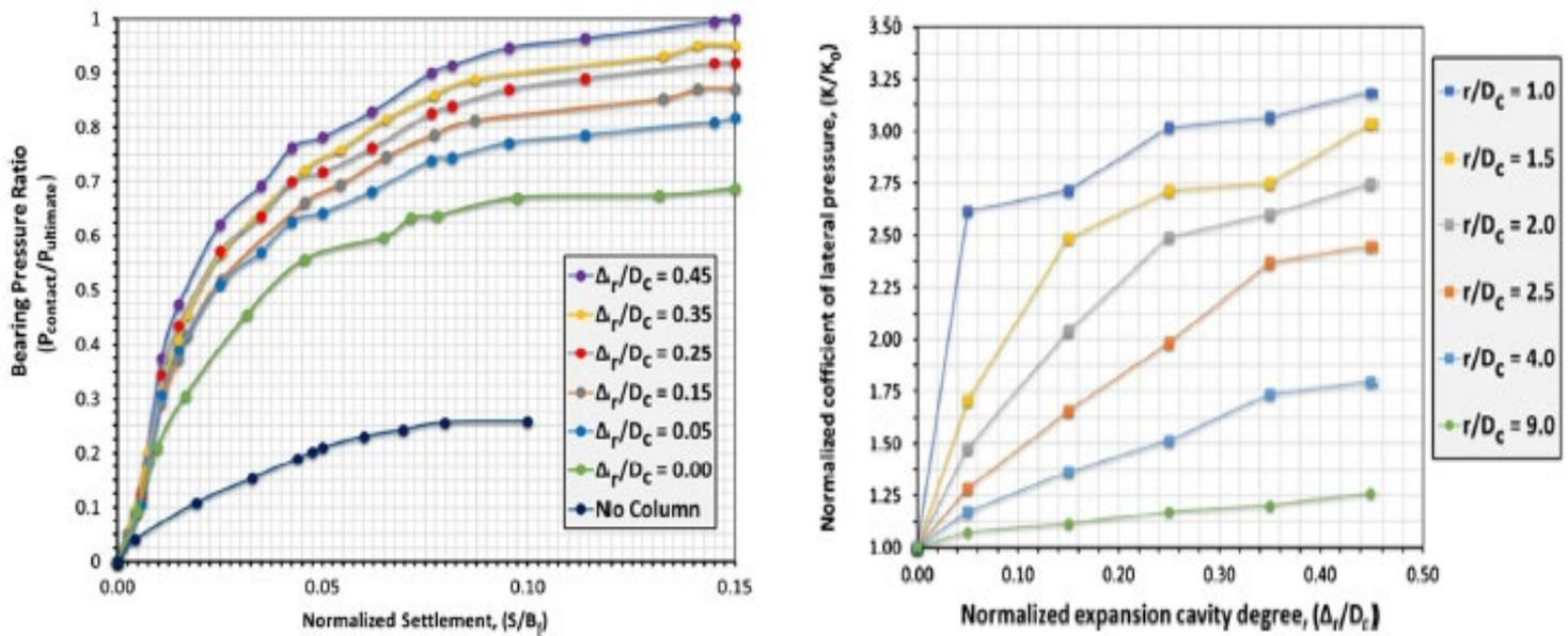
**Figure 2.15 (a)** Linked contact pressure ( $P$ ) and Normalized Settlement relationship **(b)** For inconsistent expansion ratios ( $\Delta_r/D_c$ ) change in lateral pressure parameter ( $K/K_0$ ) along radial distance ( $r/D_c$ ) [143]
