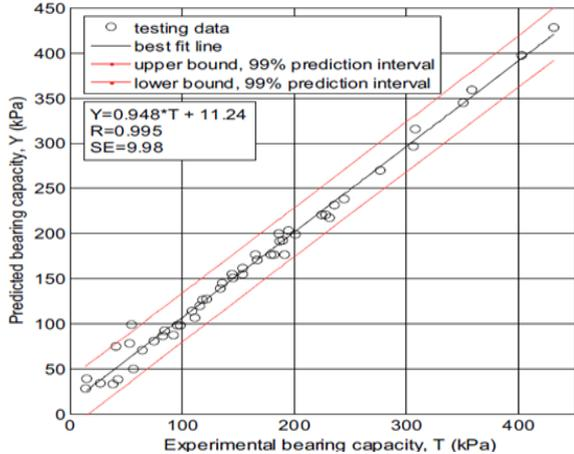
**Figure 2.41 (a)** SVR-ERBF model graph of experimental bearing capacity vs. predicted bearing capacity for research collection [253]
