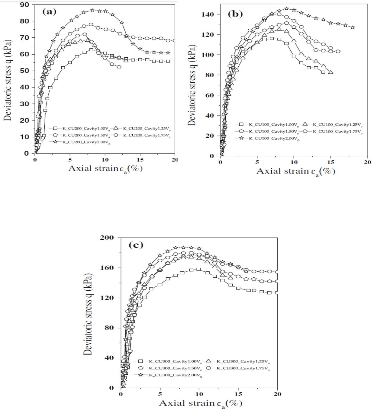
**Figure 2.9** (a) During tri axial shear loading axial shear-strain curves = 100 k Pa, (b) During triaxial shear loading axial stress strain curves =200 k Pa and (c) During tri axial shear loading axial stress–strain curves = 300 k Pa [114]
