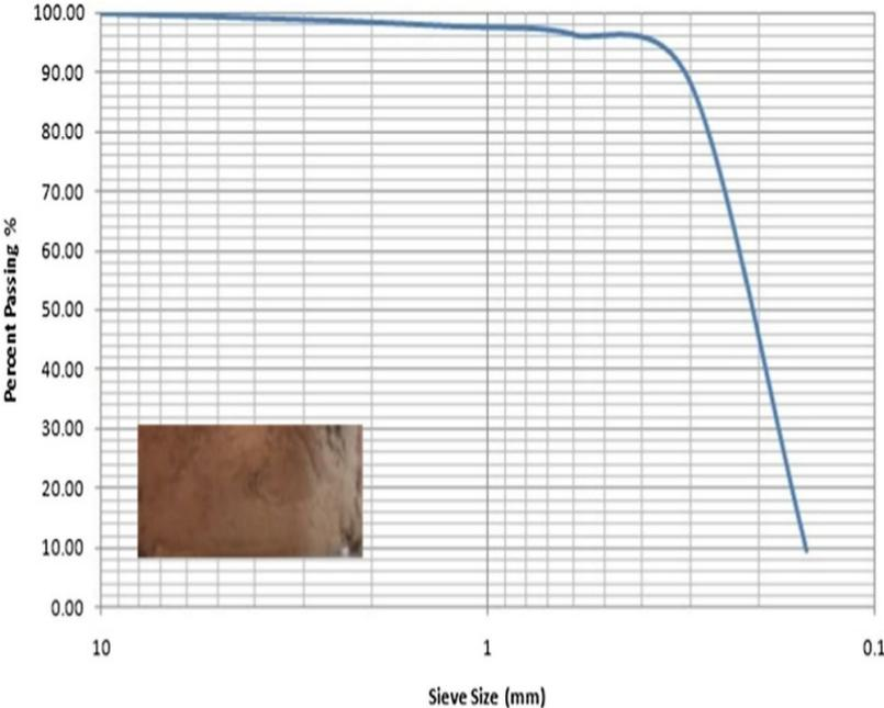
**Figure 3.2** Particle-size distributions for soil
