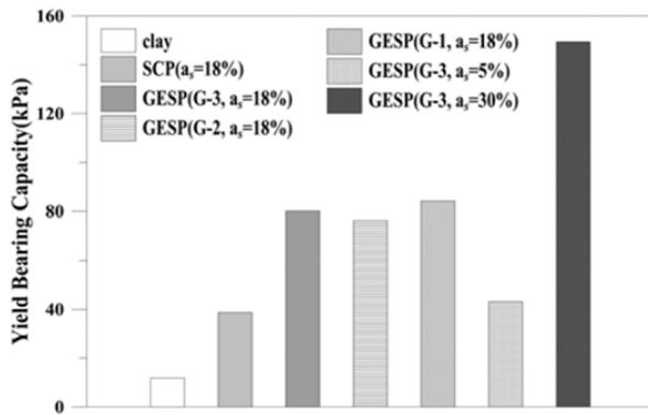
**Figure 2.24 (a)** Comparison of Ultimate Bearing Capacities of Test Cases [198]
