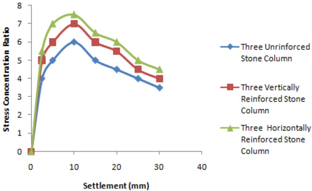
Figure 4.9 Variation of Stress concentration ratio versus settlement for 3 stone columns
