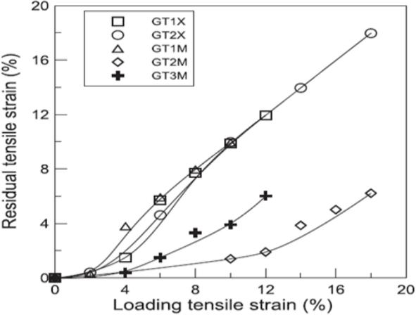
Figure 2.38 (a) Relationship between loading and residual tensile strains for all measurements Geotextiles [202]
