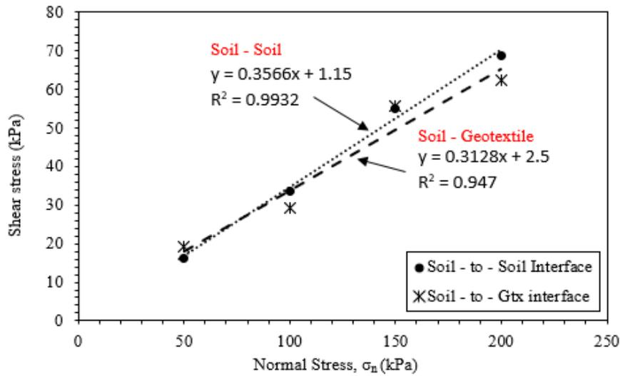
**Figure 3.24** Interface friction angles
