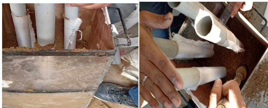
**Figure 3.16** Vertically encased group of stone Column (3 & 4)
