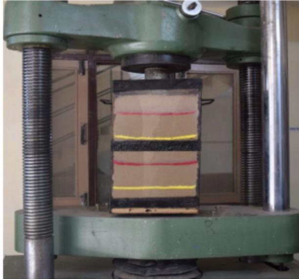
**Figure 3.6** Testing of stone columns.
