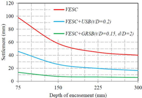
**Figure 2.36 (b)** Alteration of the settlement versus the depth of encasement [229]
