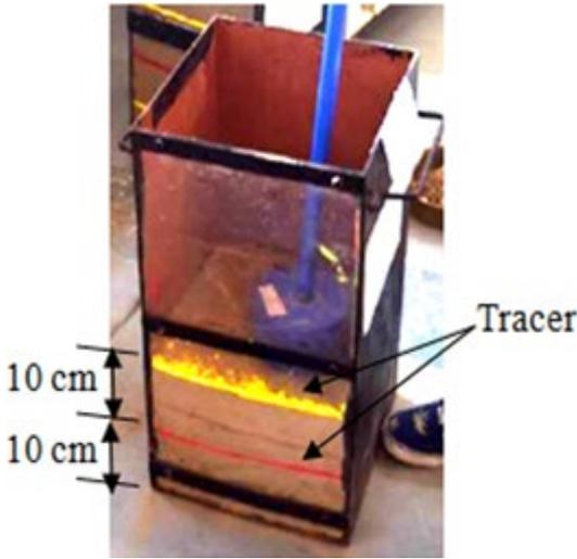
Figure 3.11 (b) Tracers are used to mark 10cm layers.
