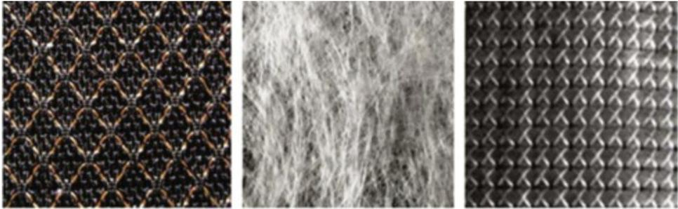
**Figure 1.8** Woven, nonwoven, and knitted geotextiles
