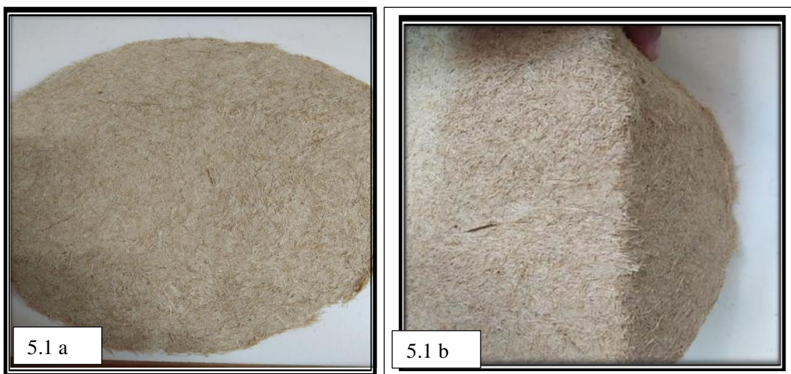
Fig 5.1a: Paper produced from pine needles and Fig5.1 b: shows breaks in paper
