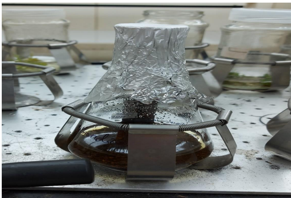
Figure 4.1 Incubation on shaking incubator for extract preparation.
