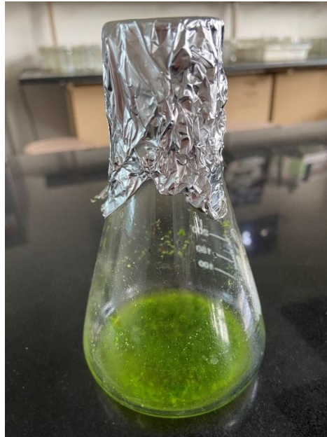
Fig.4.8- Extract in flask after removing from shaker
