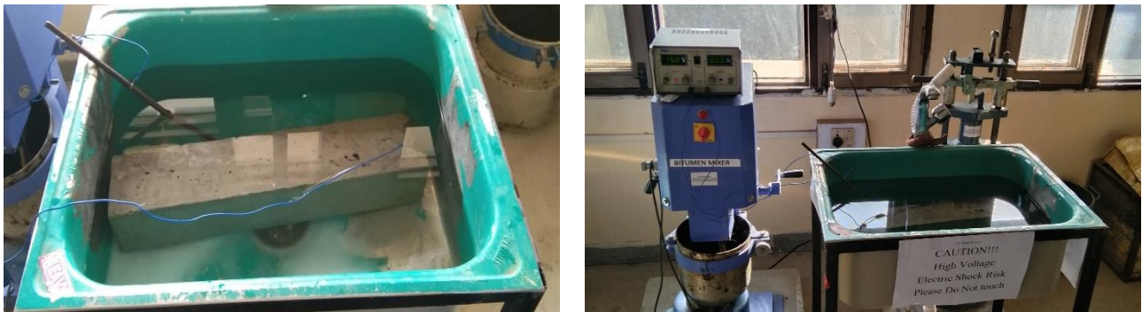
Figure 3.13. Accelerating Corrosion Setup
