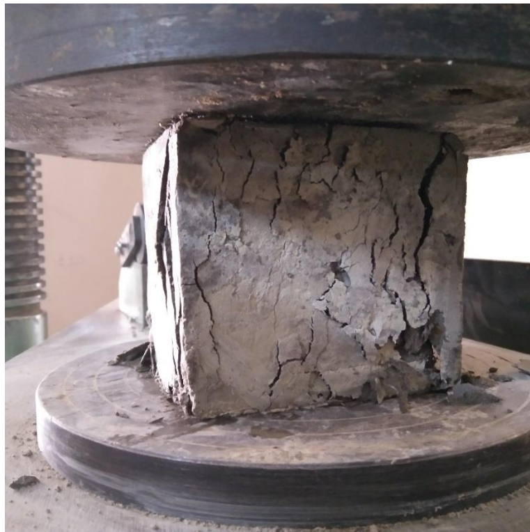
Figure 3.10 Testing cubes under compression test
