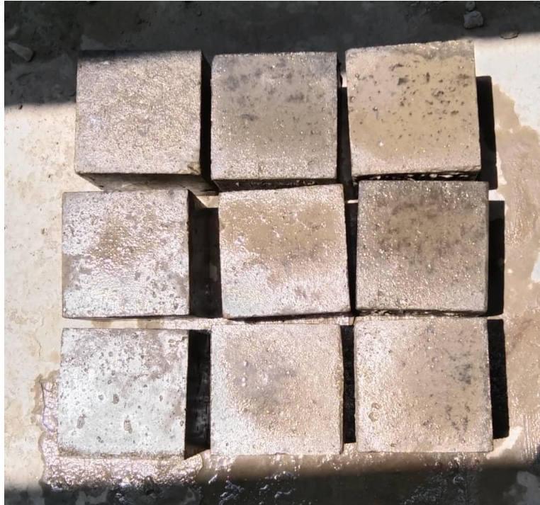
Figure 3.9 Concrete Test Cubes
