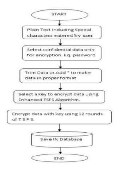
When dealing with sensitive data such as passwords, addresses, marks, and so on, the TSFS algorithm is used. It processes data using three keys, each of which is divided into 12 subkeys. The given keys are kept in a 4 X 4 matrix, therefore the length of the key must be 16 digits, and if the user supplies fewer than 16, padding is applied to the matrix. After that, we'll relocate the rows in order to conduct four operations on them: key expansion, key.
