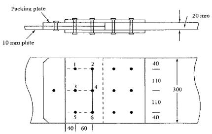
Q2. A bracket plate connected to a column flange transmits a load of 100 kN as shown in the figure. Find the maximum force for which the bolts should be designed? [5 Marks]
