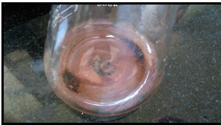
Figure 4.2: Copper layer formed at the bottom of vessel.
