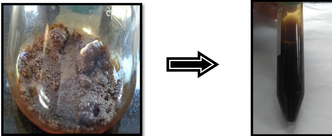
Figure 4.1: Water added to brown colored layer at the bottom, giving us the nanoparticle solution.
