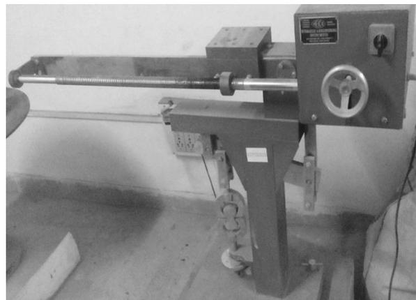
Figure 4.6 - Tensile testing machine
