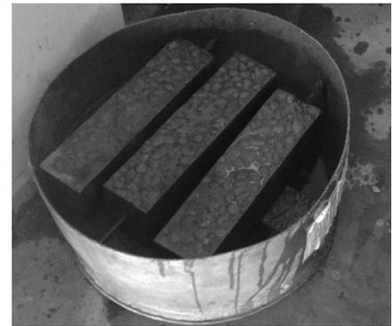
Figure 4.16 - Curing of specimens
