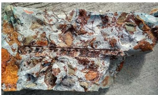
Figure 4.24 – Corrosion of steel fibers in SF specimen
