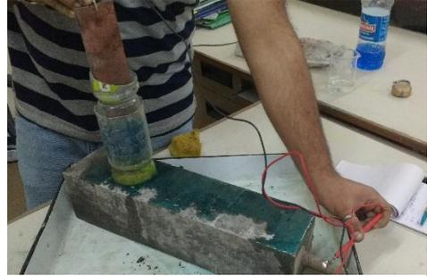
Figure 5.1 - Half-cell potential setup
