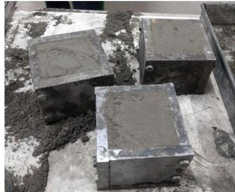
Figure 4.5 - Casting of cubes
