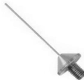
Figure 4.2 - Needle used for finding initial setting time of cement
