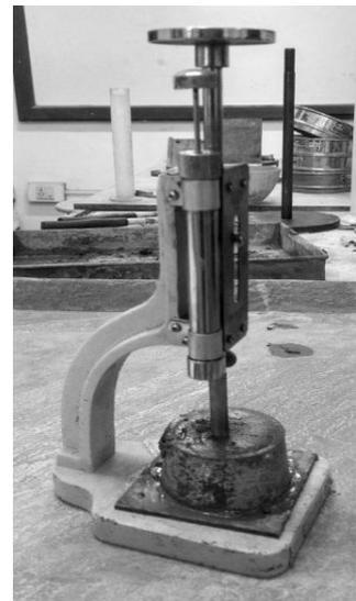
Figure 4.1 - Vicat's apparatus
