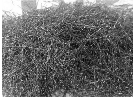
Figure 4.13 - Crimped steel fibers
