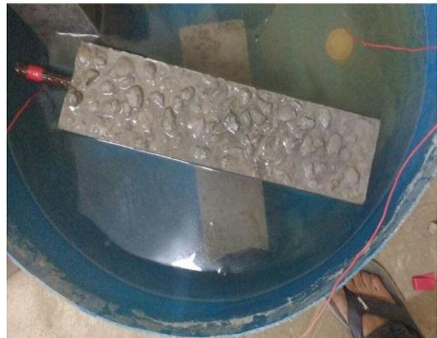
Figure 4.18 - Specimen placed in 3% NaCl solution
