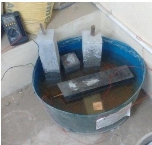
Figure 4.19 - Setup for accelerated corrosion
