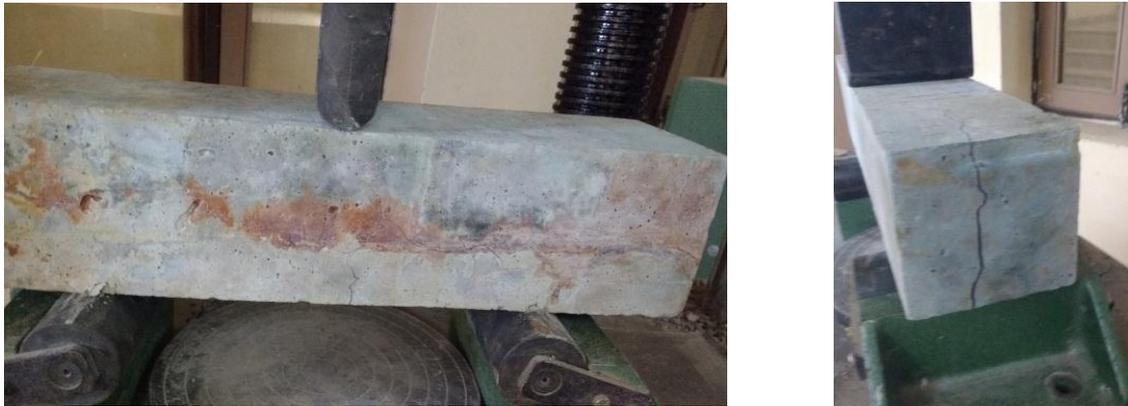
Figure 5.2 - Crack pattern at failure for flexure strength
