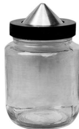
Figure 4.9 - Pycnometer
