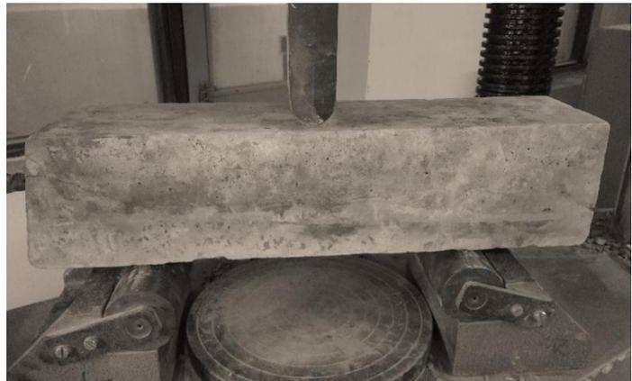
Figure 3.2 - Center point loading for calculation of Flexural strength
