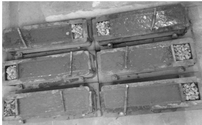
Figure 4.15 - Casting of specimens
