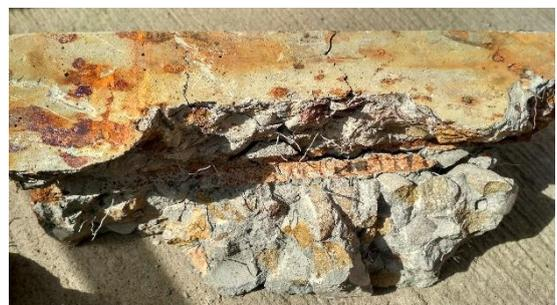
Figure 4.23 - Corrosion of steel fibers in SF+A specimen
