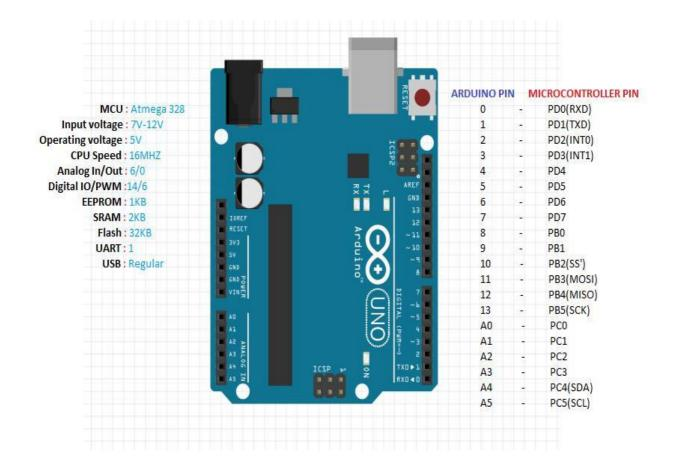
The Uno is equipped with the Atmega16U2 (Atmega8U2 up to version R2) that has the facility to be programmed as a USB-to-serial converter, which makes it easy to develop extensive circuits without the need of a large paraphernalia of debugging tools. Revision 3 of the board has the following new features a stronger RESET circuitry, hence it's a more reliable platform than its predecessors.
