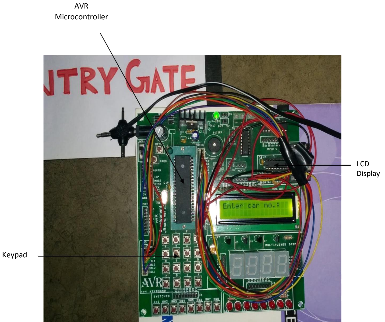
Figure 3.14: Photo of smart parking area control board (at Entry Gate)
