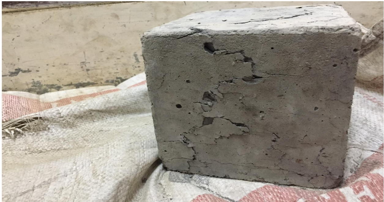
Figure 3.2 Compression test failure
