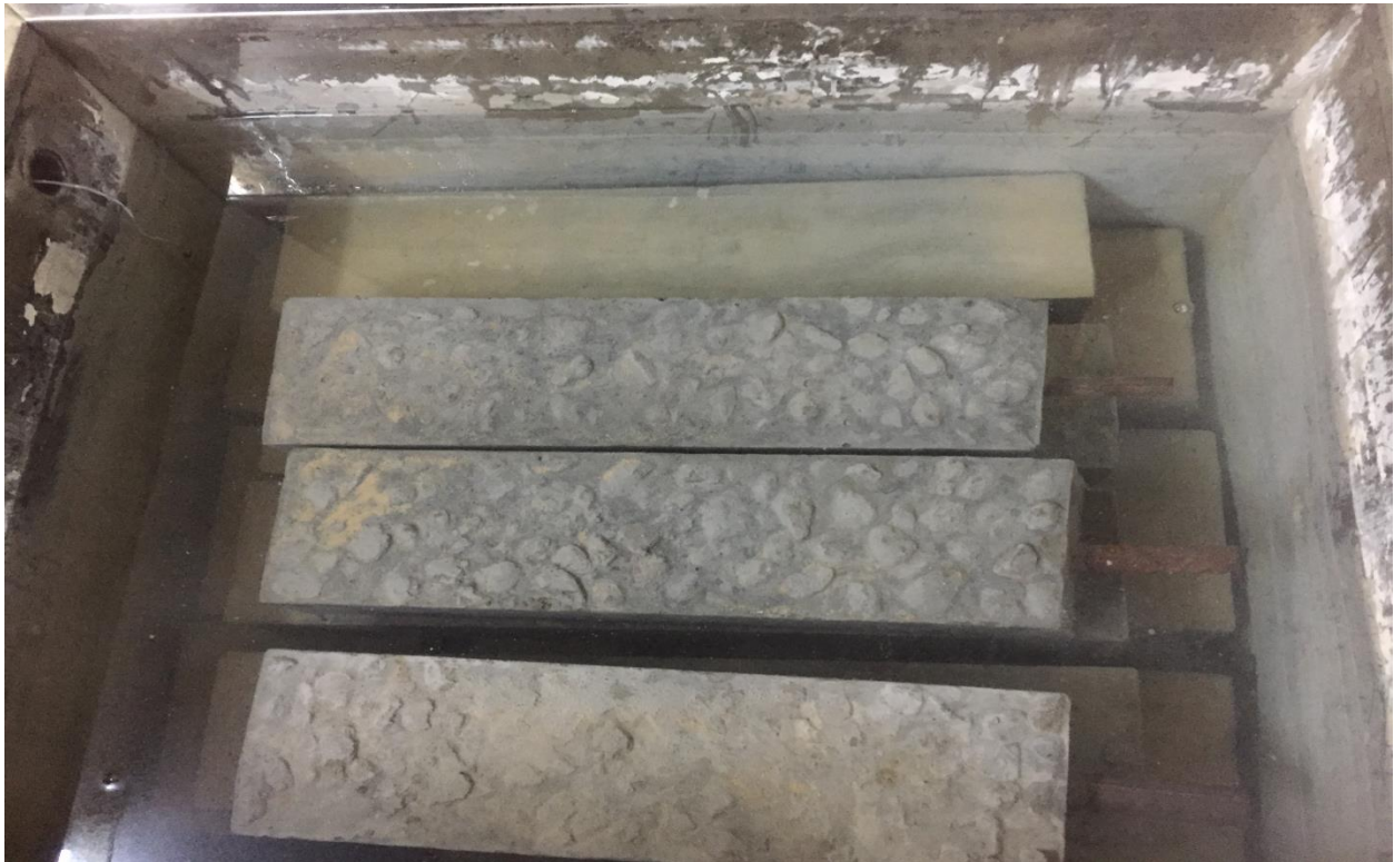
Figure 3.4 Beams in rapid Curing Tank
