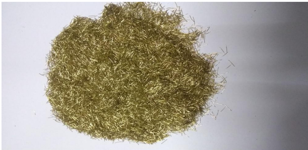
Figure 4.1 Short fibers Length 6 mm aspect ratio 30
