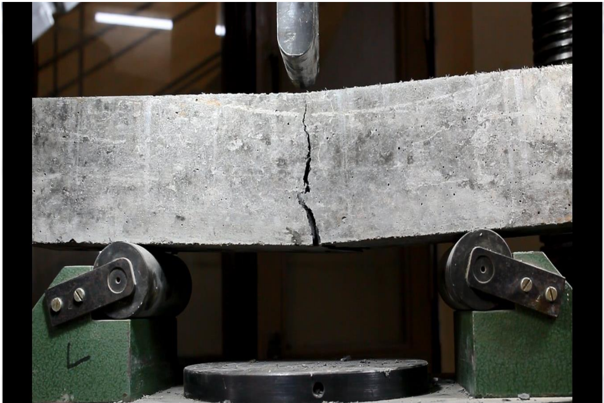
Figure 3.3 Flexure Test Failure
