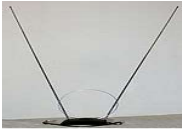
Figure 3.3. A typical rabbit antenna [11] .
