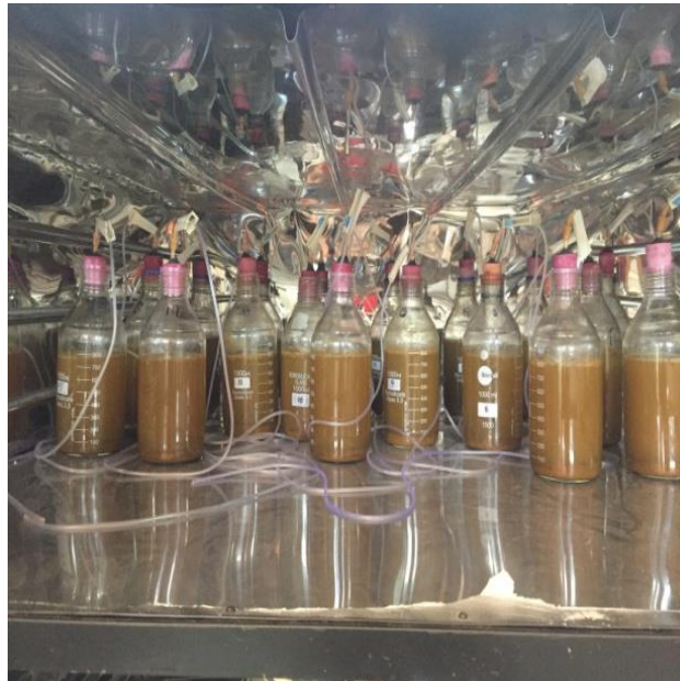
Fig3.2 Digesters in Incubator at 35°C
